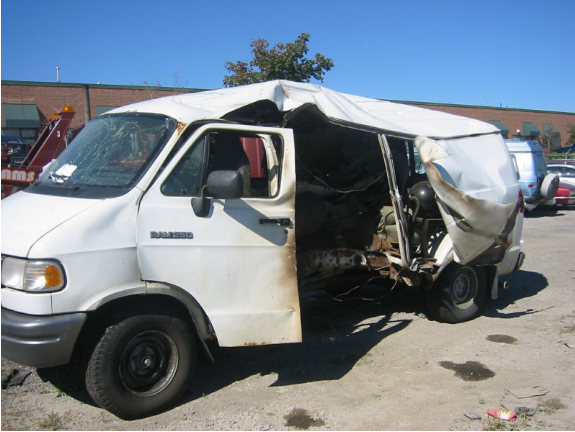
Figure 3 - A Vehicle after Fuel Tank Failure
