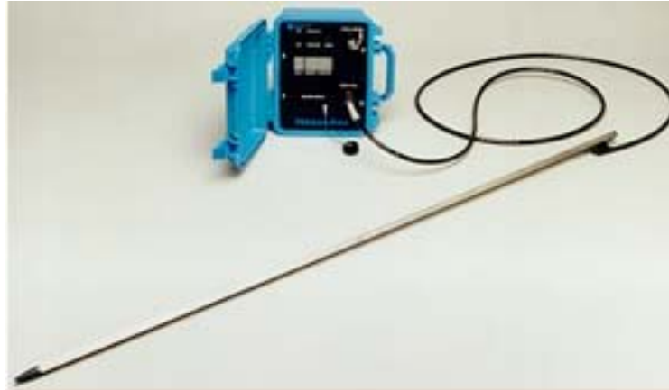
Figure C-6: Environmental Sensors Inc. – TDR Unit
