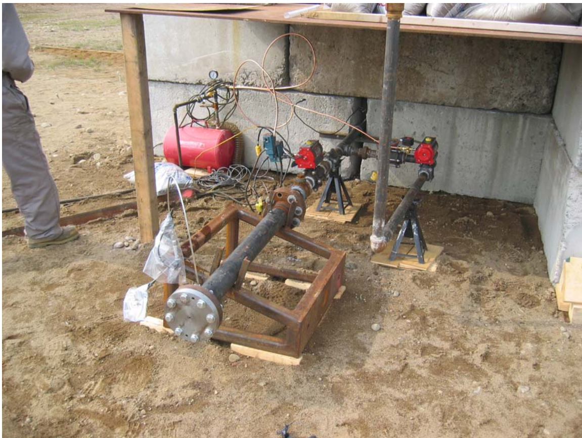
Figure 3.9: Computer-controlled PRV (air reservoir, control valve, backup PRV stack valve, nozzle plate)
