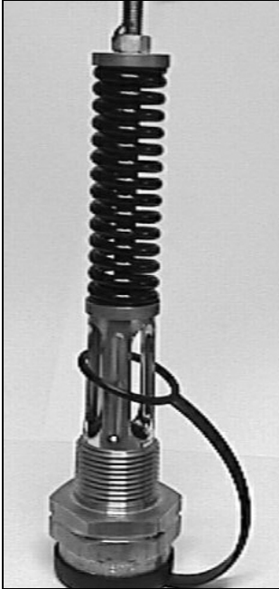
Figure 3.6: Original tank PRV (250 psig, 1 in. diameter, 2565 scfm)
