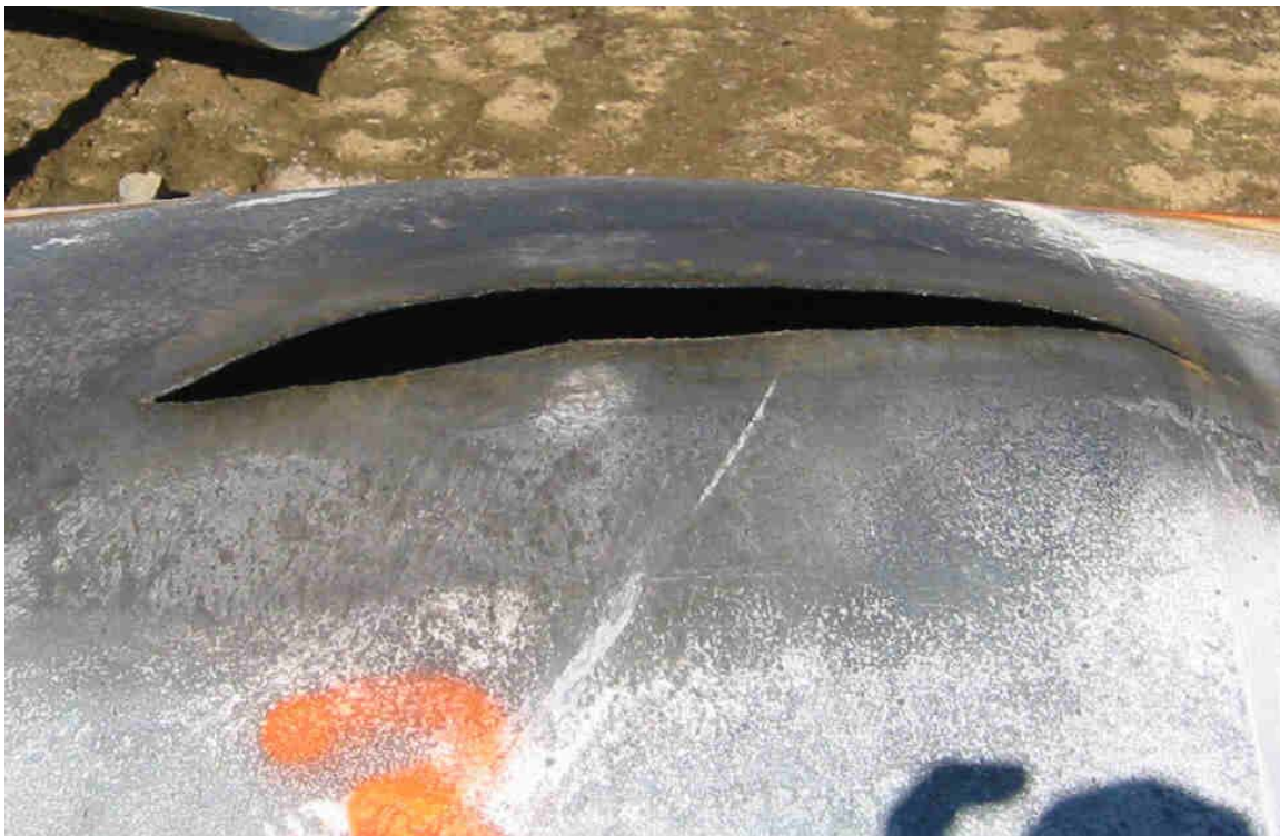
Figure 4.32: Tank failure, Test 04-3
