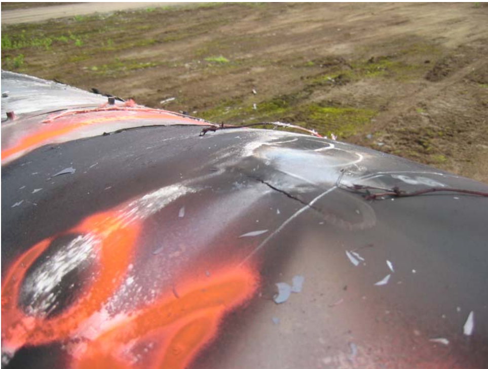
Figure 4.42: Test 04-5, small rupture with small insulation defect (again, tank wall contact with the outer steel jacket is suspected)
