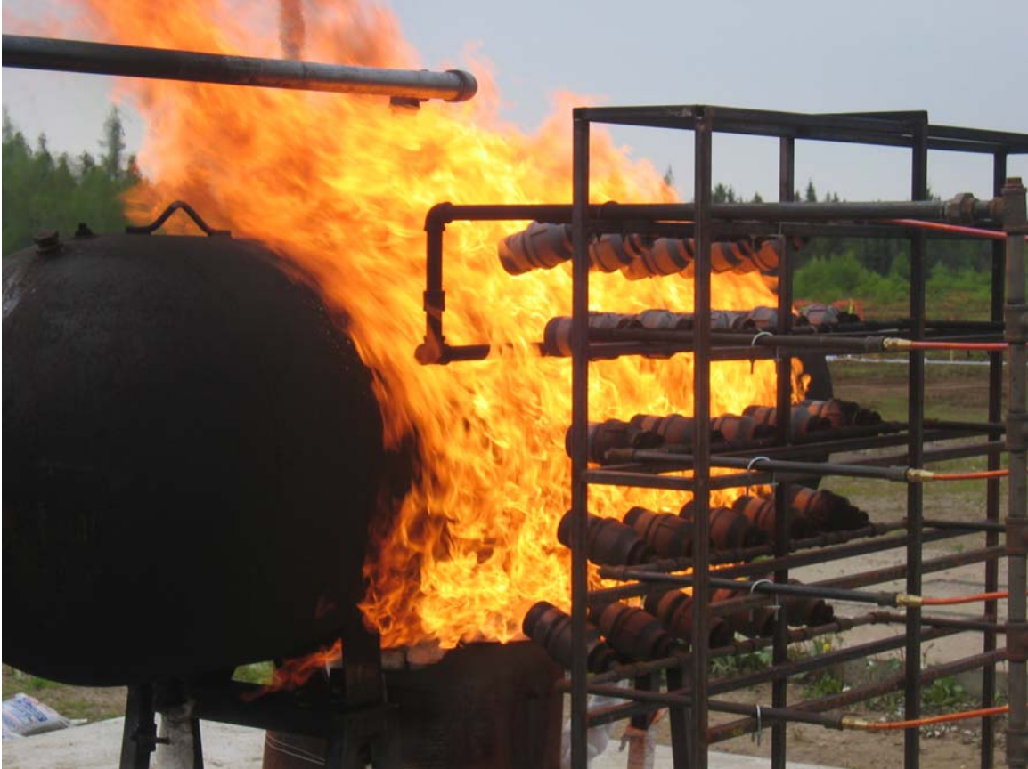
Figure 4.1: Burner system in operation (note luminous pool fire-like flame, and flame wrapping around tank with wind from right to left (northwest wind))
