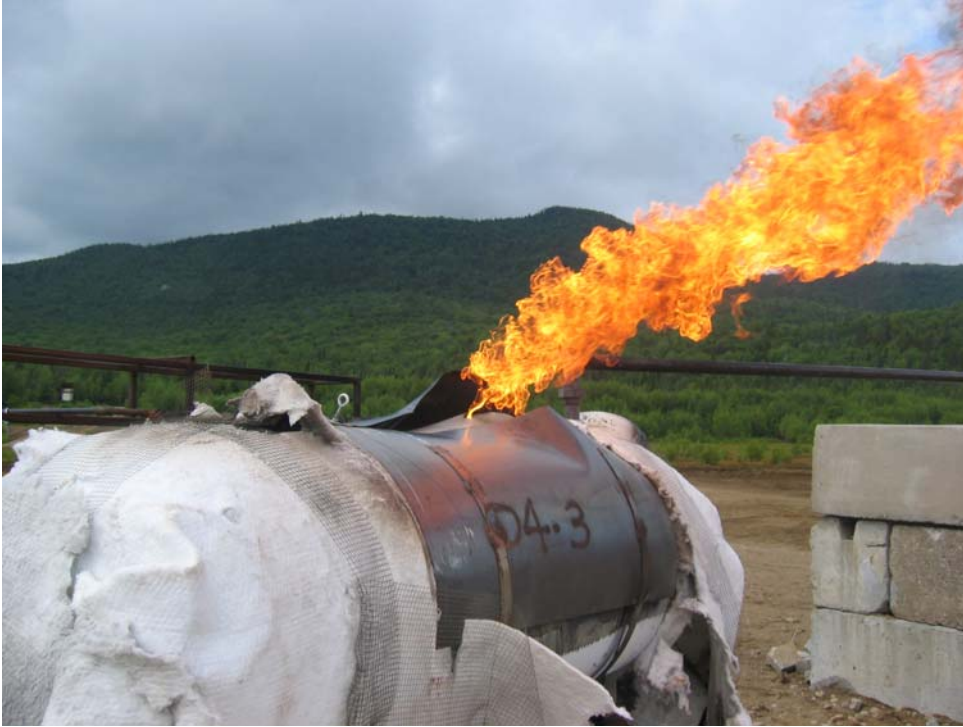
Figure 4.30: Test 04-03 tank after rupture (the steel jacket split open at the top tack weld)
