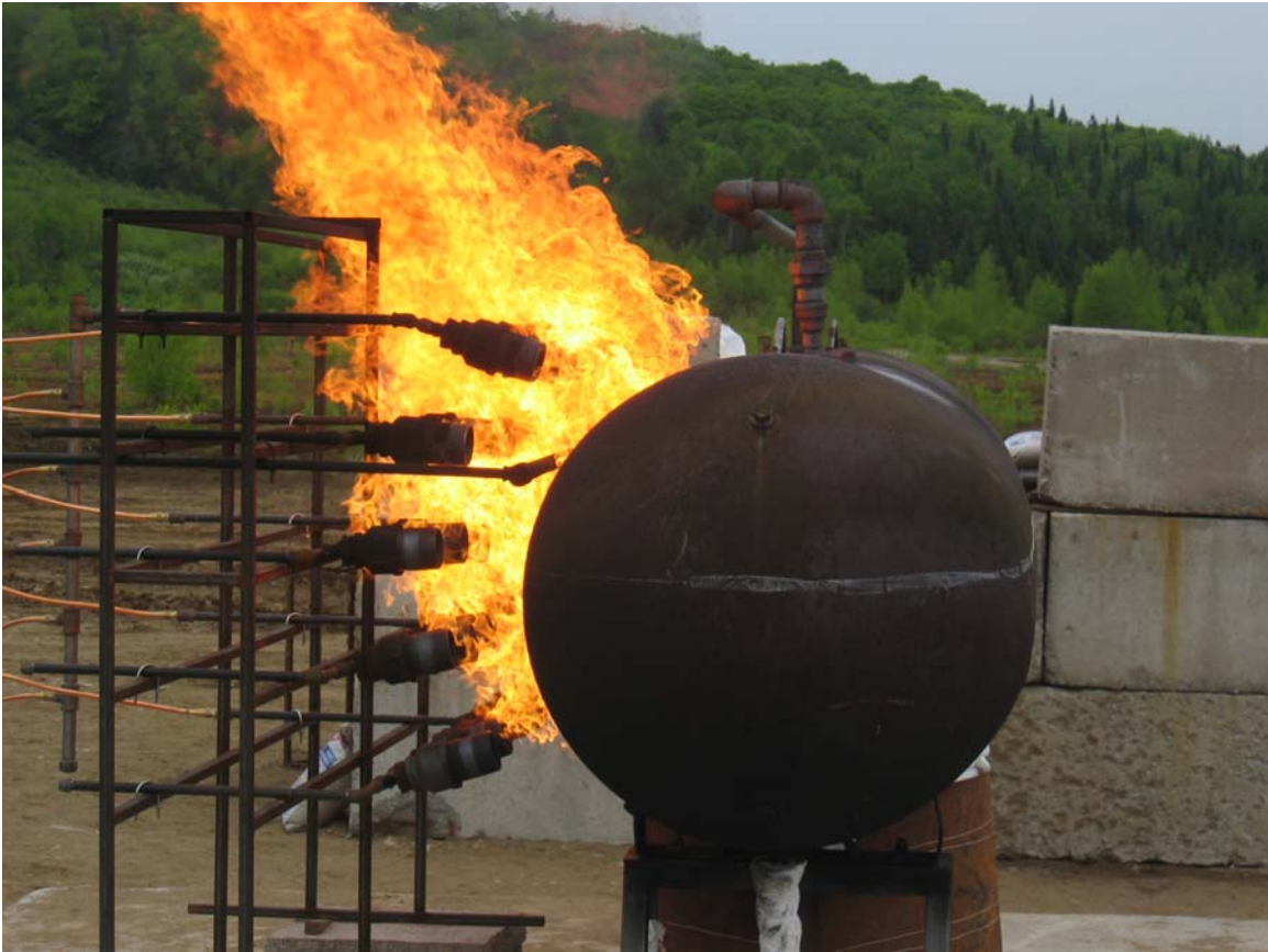
Figure 4.4: Picture showing poor fire contact on tank top (wind from east (right to left))
