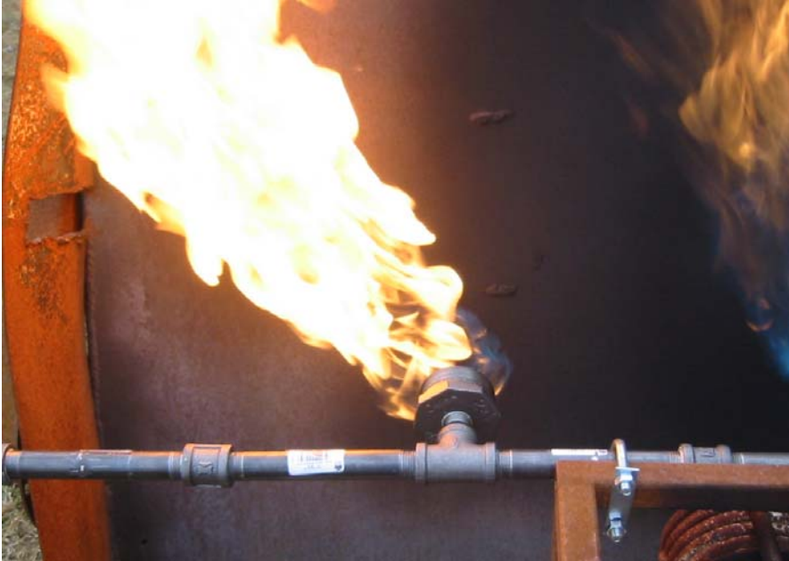
Figure J.4: Burner Design C flame. Note that flame is luminous and well attached to burner, but directional stability is not good.
