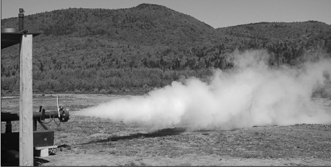
Figure 3.10: PRV nozzle operating with steam flow
