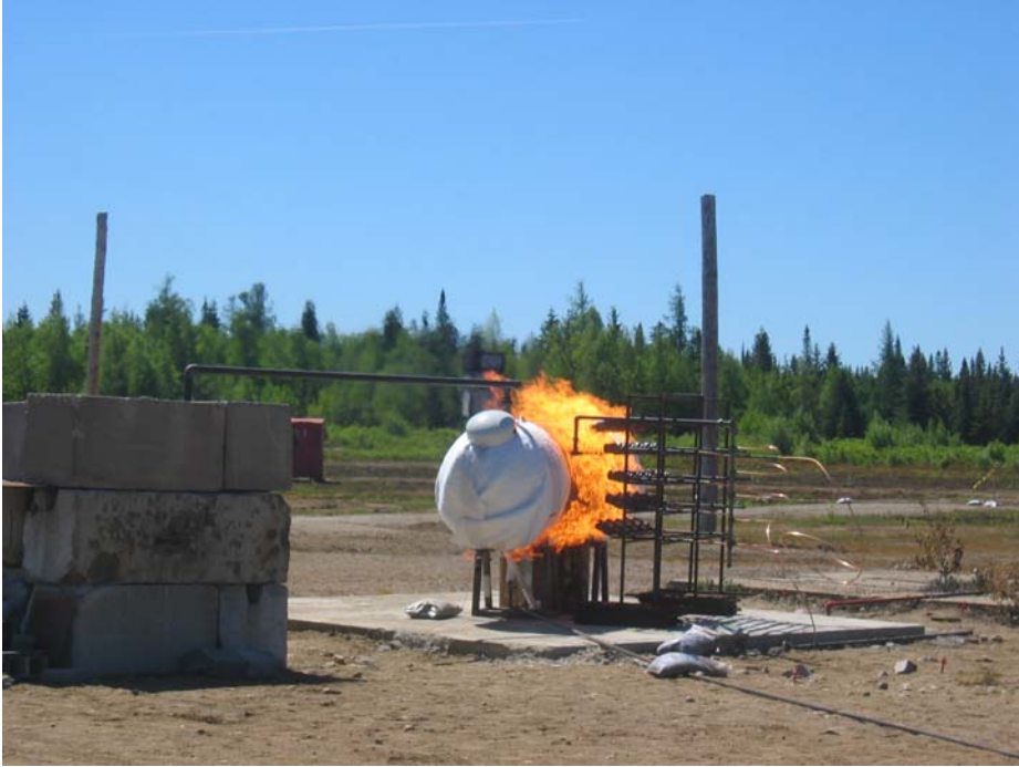
Figure 4.17: Fire condition at beginning of Test 04-02
