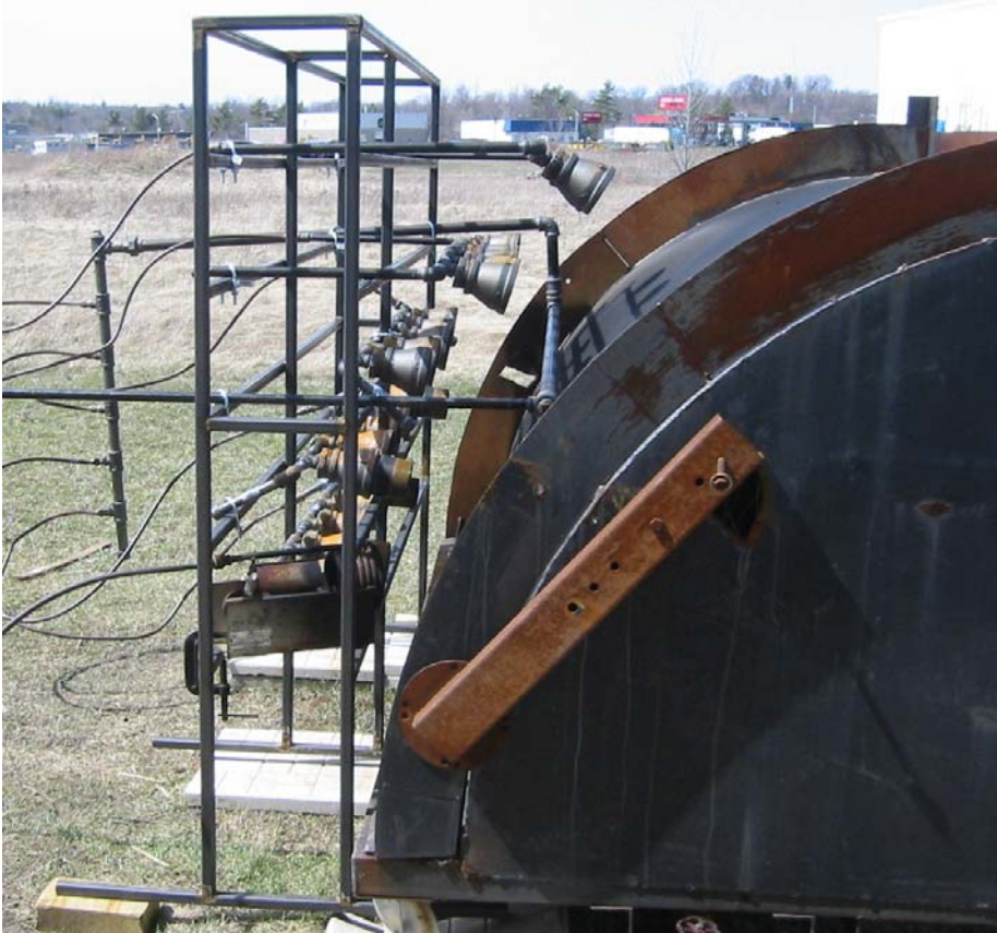
Figure J.8: Side-view of five 5-burner arrays on 1/4 section test shell.
