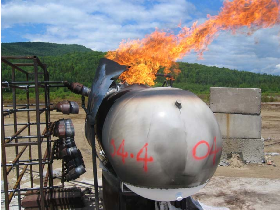
Figure 4.36: Test 04-04 rupture with split jacket (note burned vapour space)
