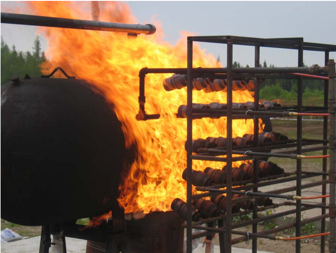
Figure D.1: Burner system in operation. Note luminous pool-fire-like flame, and flame wrapping around tank with wind from right to left (northwest wind).
