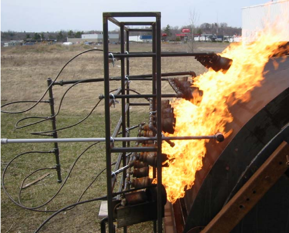
Figure J.10: Side view of flame from five 5-burner arrays on 1/4 section test shell. Note frost on evaporator inlet.
