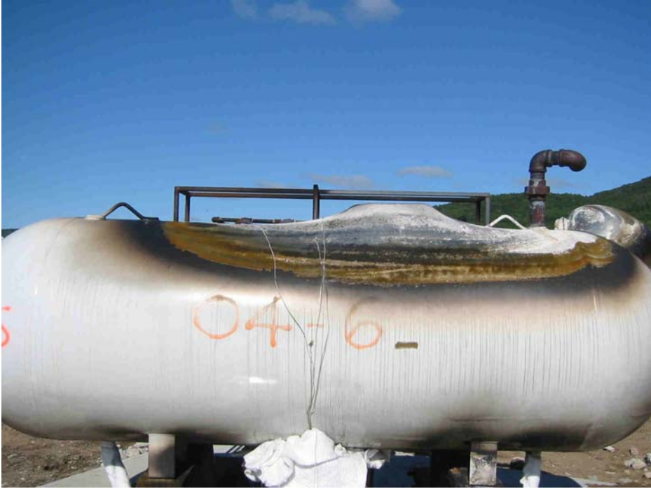
Figure 4.12: Tank after failure, Test 04-6
