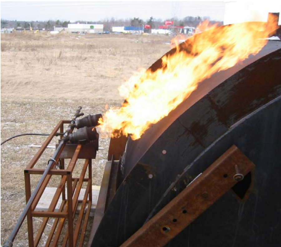
Figure J.5: Burner Design D flame. Note that flame is luminous, attached to burner and directional stability is better than Design C.
