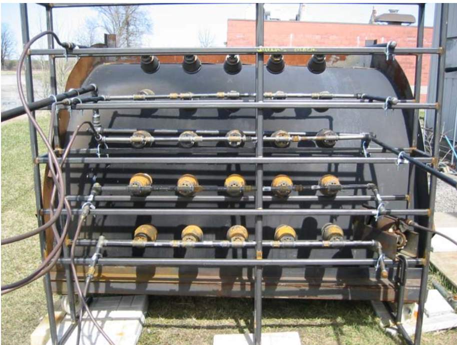
Figure J.9: Back view of five 5-burner arrays on 1/4 section test shell.
