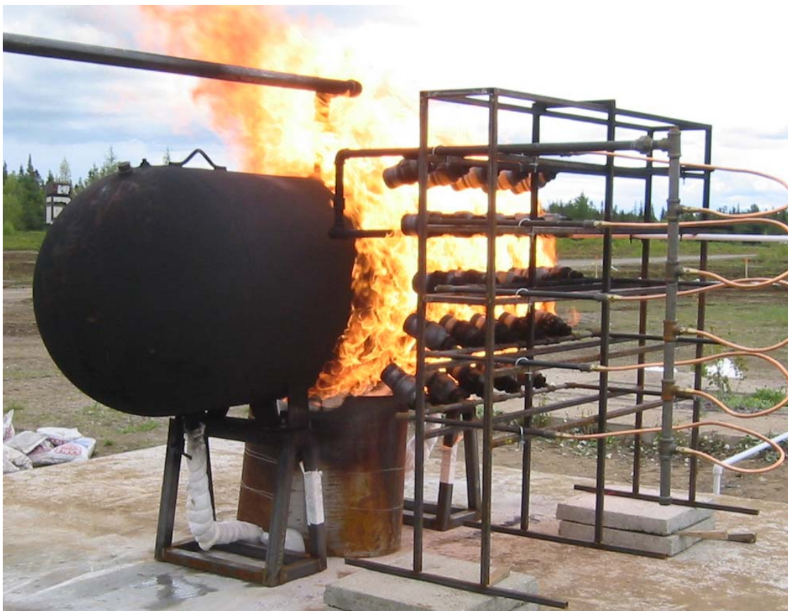
Figure 3.3: Burner array and evaporator set-up
