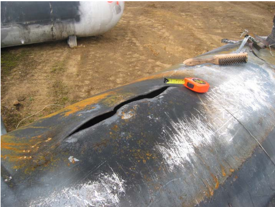
Figure 4.37: Tank rupture, Test 04-04 (note jagged tear, suggesting wall made contact with jacket and jacket provided some support)
