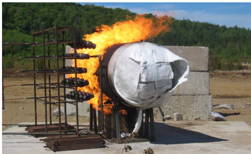
Figure 4: ASME Code 500 gal. Test Tank with 25% Fire Engulfment (fire blackbody temperature 800-900°C) [4]
