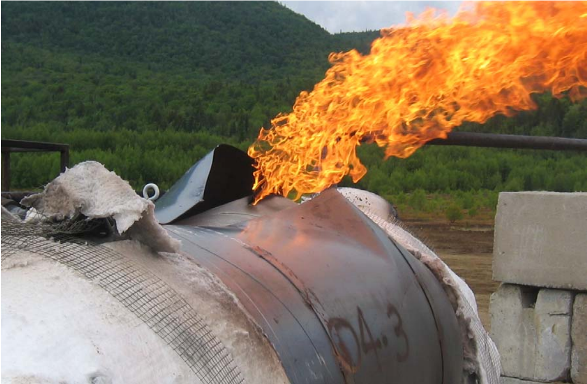
Figure 9: Ruptured Tank with 15 percent Thermal Protection Defect [4]
