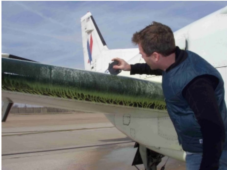
Photo 2.5: APS Personnel Taking a Fluid Thickness Measurement
