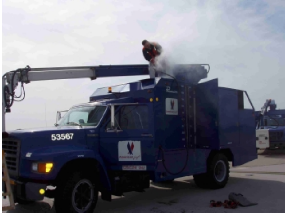
Photo 2.1: Type I Spray Vehicle Used in Type III Fluid Spray Tests at DFW
