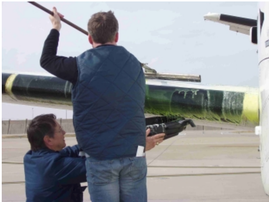
Photo 2.4: Collecting a Type III Fluid Sample from a Wing
