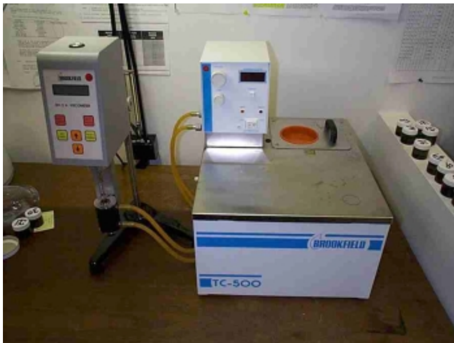
Photo 2.6: Brookfield Digital Viscometer Model DV-1+ and Temperature Bath
