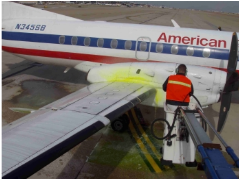
Photo 2.3: Type III Fluid Spray on Saab 340 Aircraft
