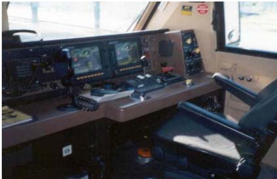
Figure 6: First engineman's driving position with all controls and two screens for engine diagnostics and status
