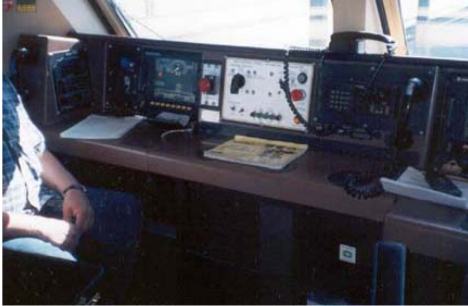
Figure 7: Second engineman's driver station with one screen, limited controls, cellular phone and radio phone
