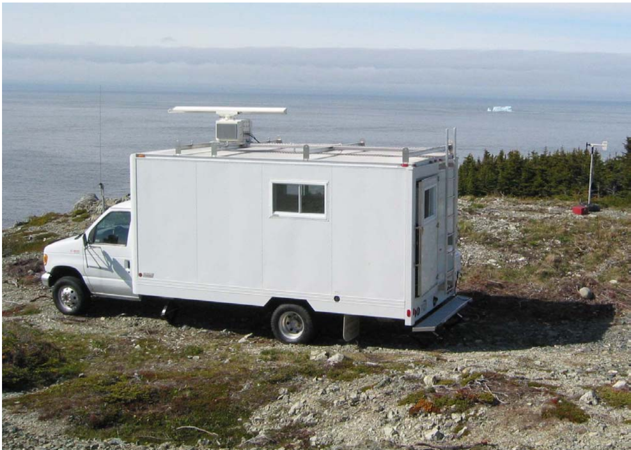
Figure 1 Mobile Radar Unit at Twillingate, Newfoundland
