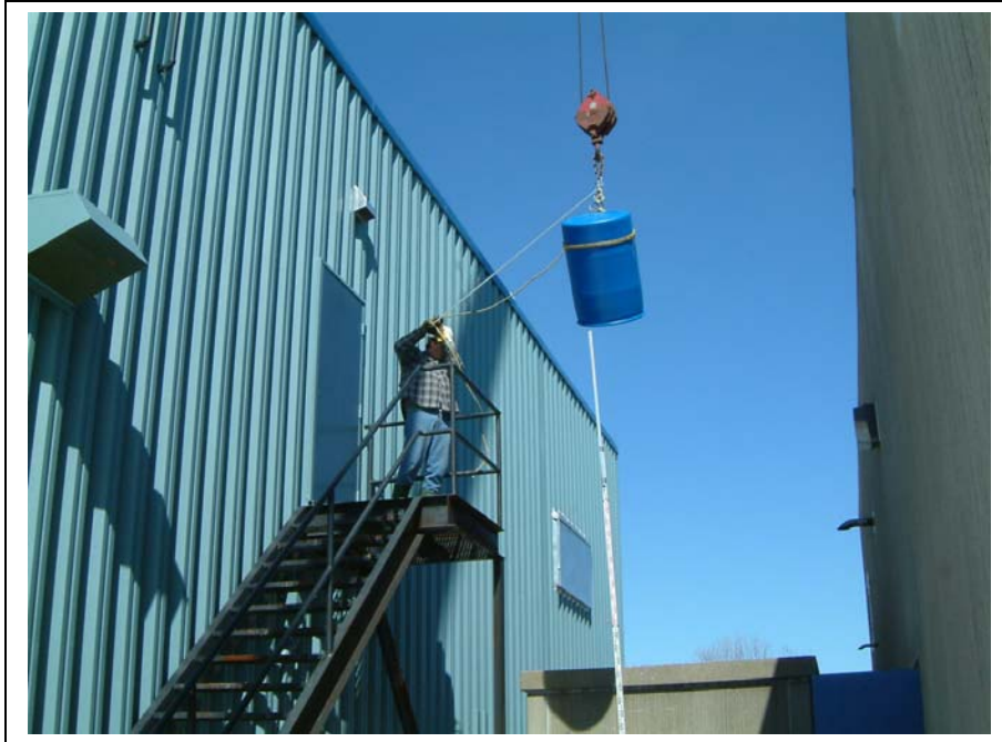
Photo 3 Test setup: Drum in final position for outdoor drop (required for higher drop heights)
