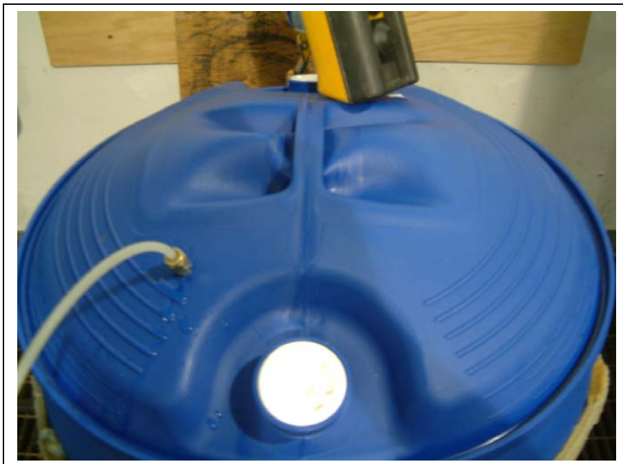
Photo 30 Drum Set G: Pressure test under way
