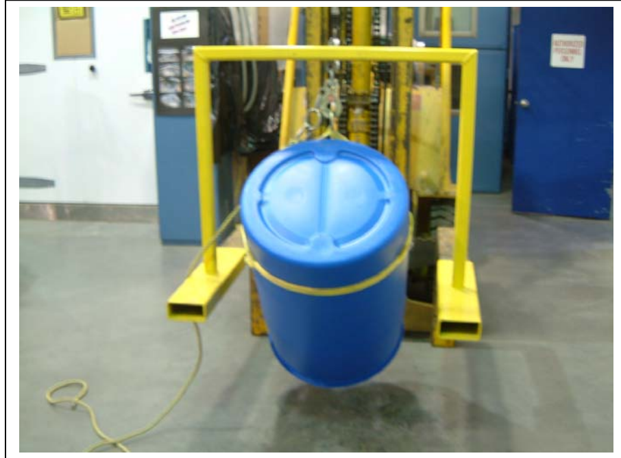
Photo 1 Test setup: Drum holding arrangement for indoor drops
