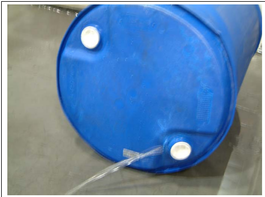
Photo 24 Drum Set F: Second failure mode - Rupture around closure
