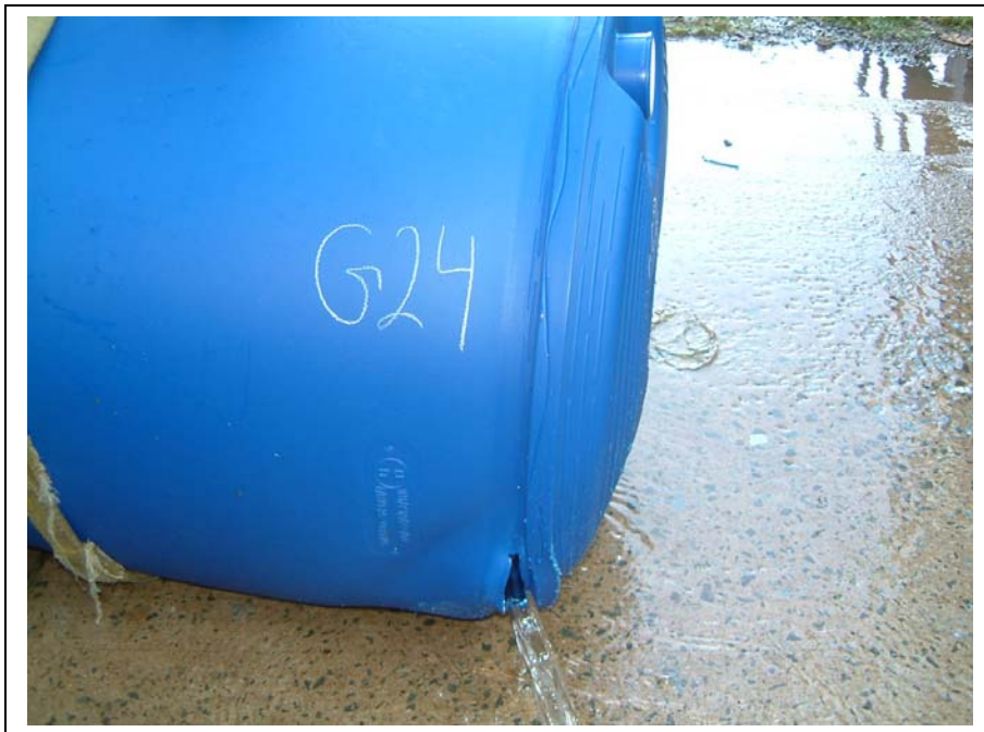
Photo 28 Drum Set G: Typical failure mode - Rupture at top/sidewall line
