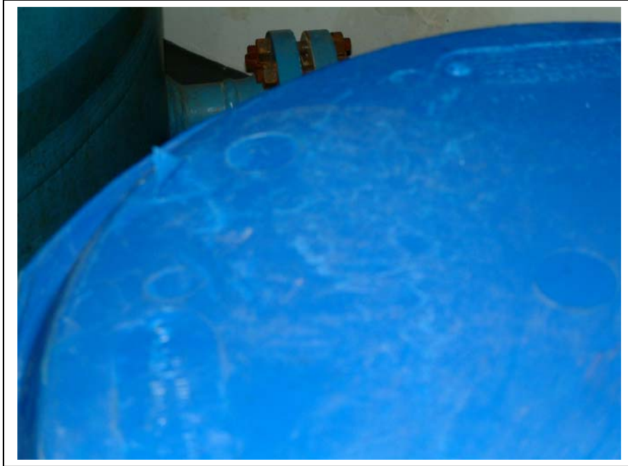
Photo 25 Drum Set F: Close-up of drum top showing delamination of material
