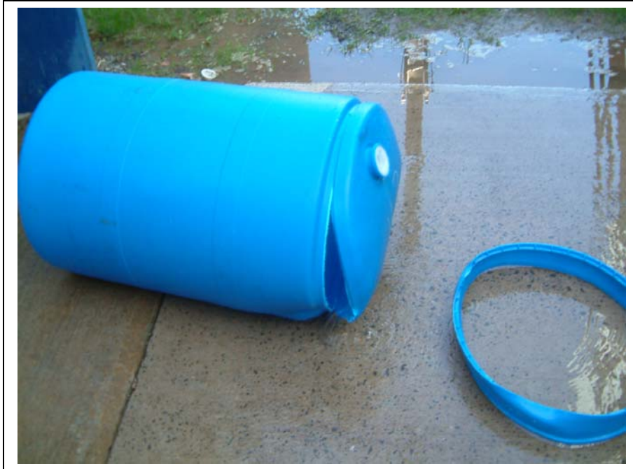
Photo 11 Drum Set C: Failure mode - Fracture at cover/sidewall seam (note top ring separated)
