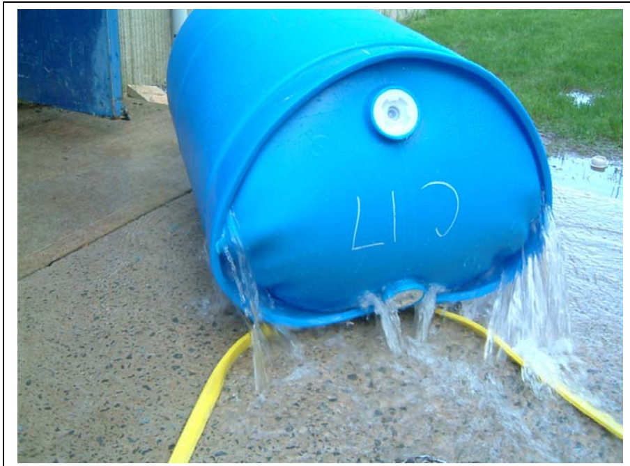
Photo 12 Drum Set C: Failure mode - Fracture at cover/sidewall seam, under the recess where top ring locates
