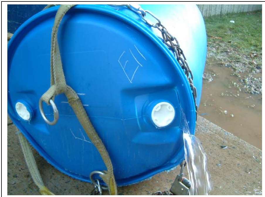
Photo 20 Drum Set E: Failure mode - Fracture between closure neck and top/sidewall seam
