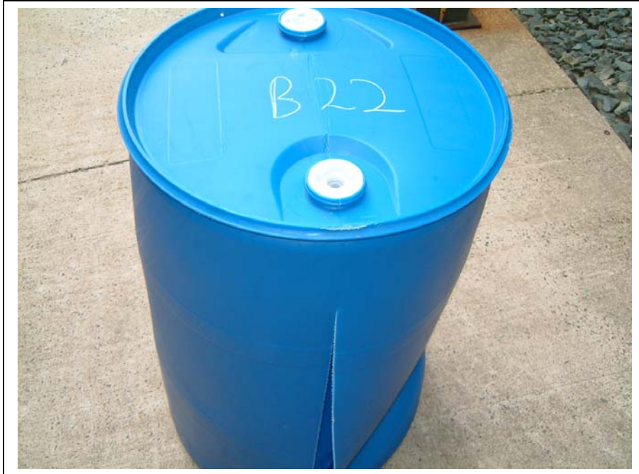
Photo 9 Drum Set B: Failure mode - Longitudinal fracture of body
