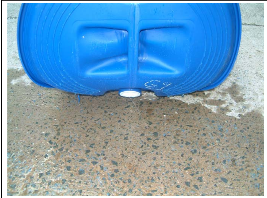
Photo 29 Drum Set G: Second failure mode - Leaking from closure
