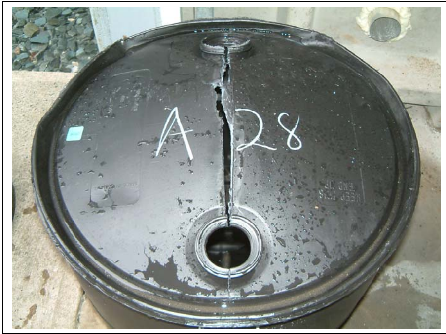
Photo 5 Drum Set A: Typical failure mode - Fracture at cover mold line
