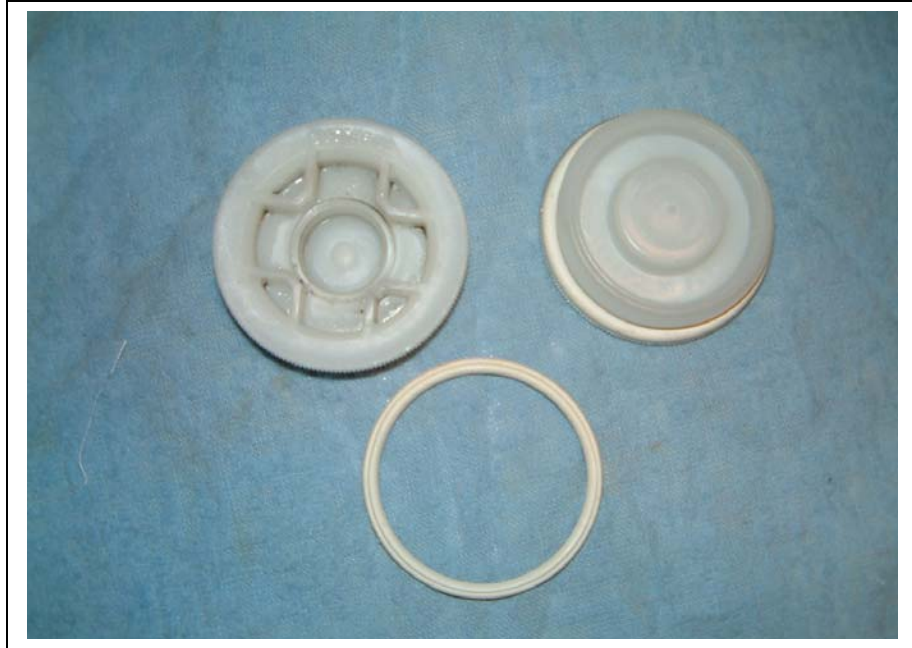
Photo 33 Example of a type c closure: Note the small, threaded knockout bung in the centre
