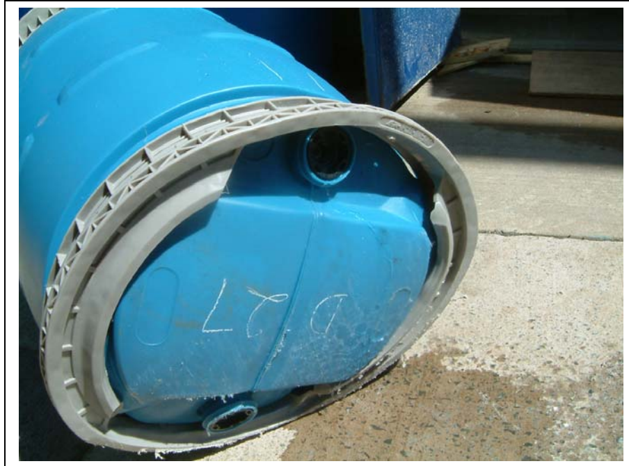
Photo 15 Drum Set D: Failure mode - Dripping from opposite closure from the one impacted
