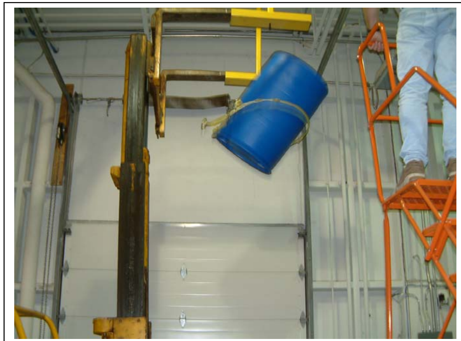
Photo 2 Test setup: Indoor drop underway
