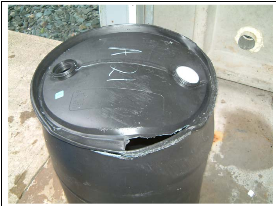
Photo 6 Drum Set A: Typical failure mode - Fracture at cover/body seam
