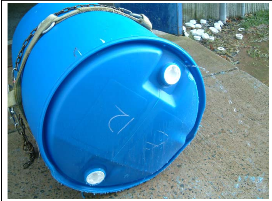
Photo 21 Drum Set E: Failure mode - Small hole near closure neck
