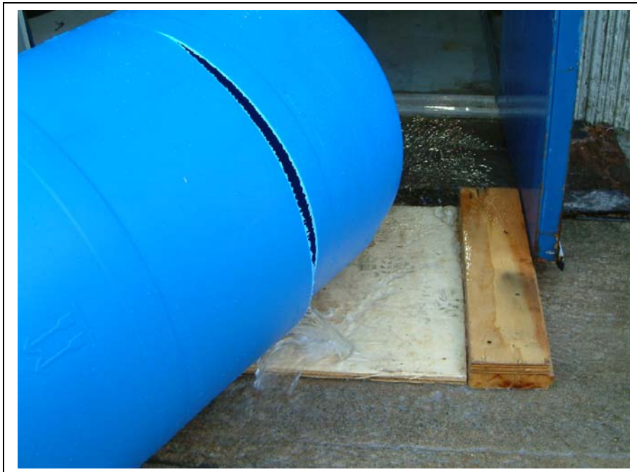
Photo 10 Drum Set B: Failure mode - Circumferential fracture next to rolling rib
