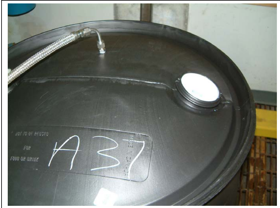
Photo 7 Drum Set A: Pressure test in showing test fitting location
