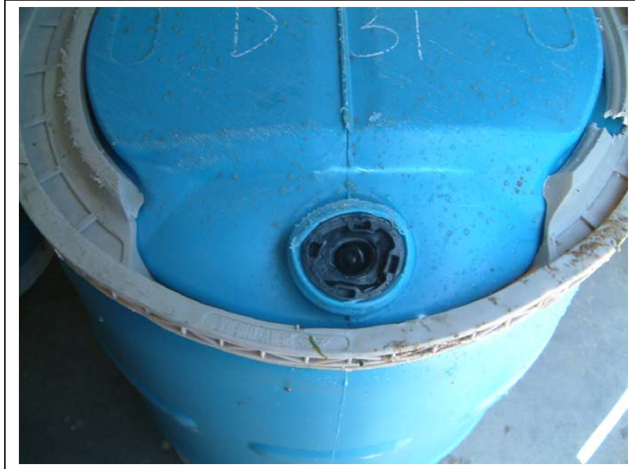
Photo 17 Drum Set D: Example of severely distorted closure neck – Still no leaks
