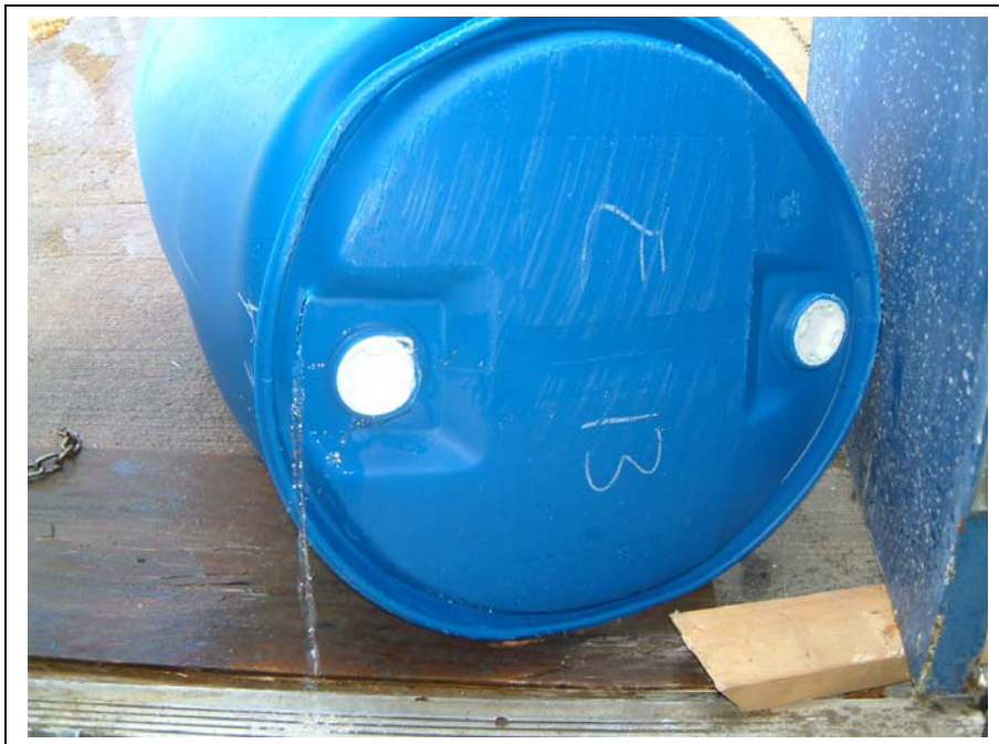
Photo 22 Drum Set E: Failure mode - Separation at edge of closure well
