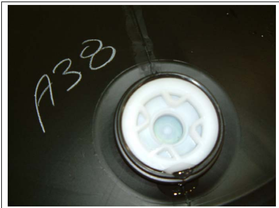
Photo 8 Drum Set A: Typical pressure test failure mode - Drip from NPS closure
