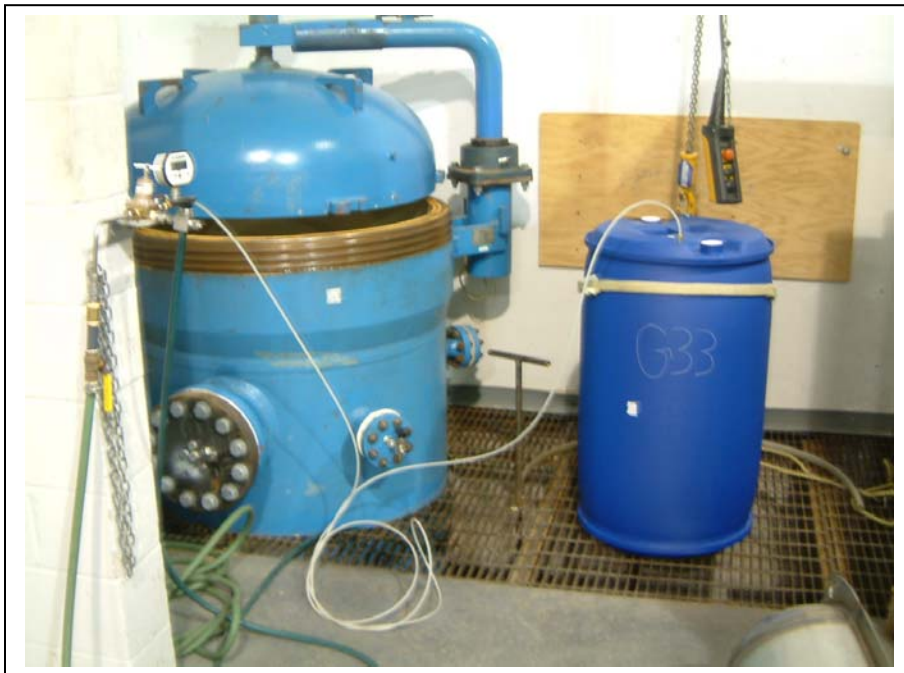
Photo 4 Test setup: Internal pressure test
