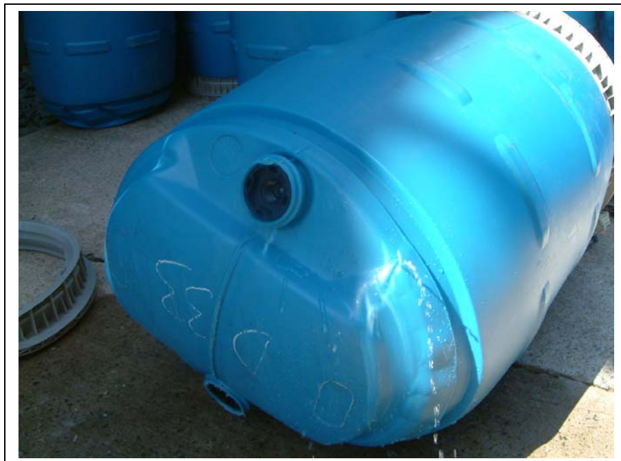
Photo 18 Drum Set D: Failure mode - Small split on edge of top/sidewall seam
