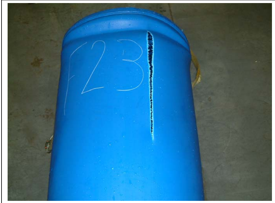
Photo 23 Drum Set F: Failure mode - Longitudinal split along sidewall
