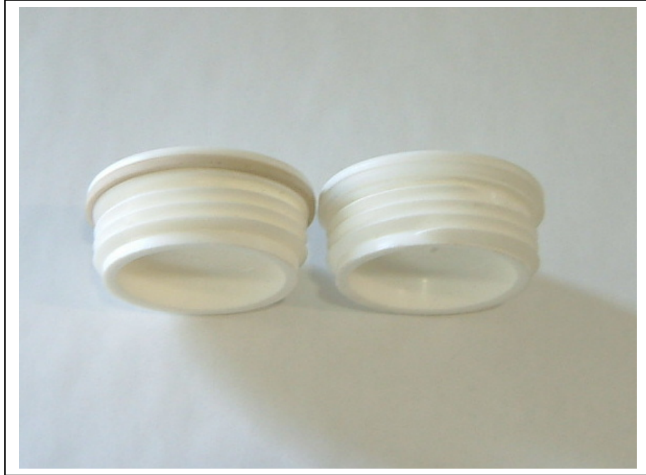
Photo 31 Comparison of two gasket types: Rectangular section, soft rubber on the left, round section, hard plastic on the right (both closures with butress threads)
