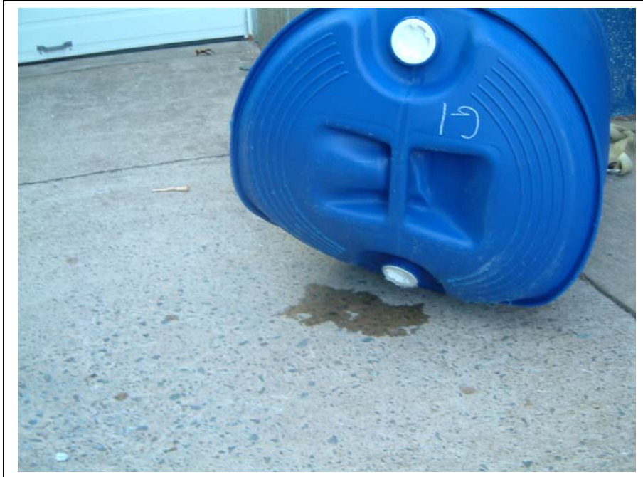
Photo 27 Drum Set G: Failed drum showing extent of distortion of top handle area
