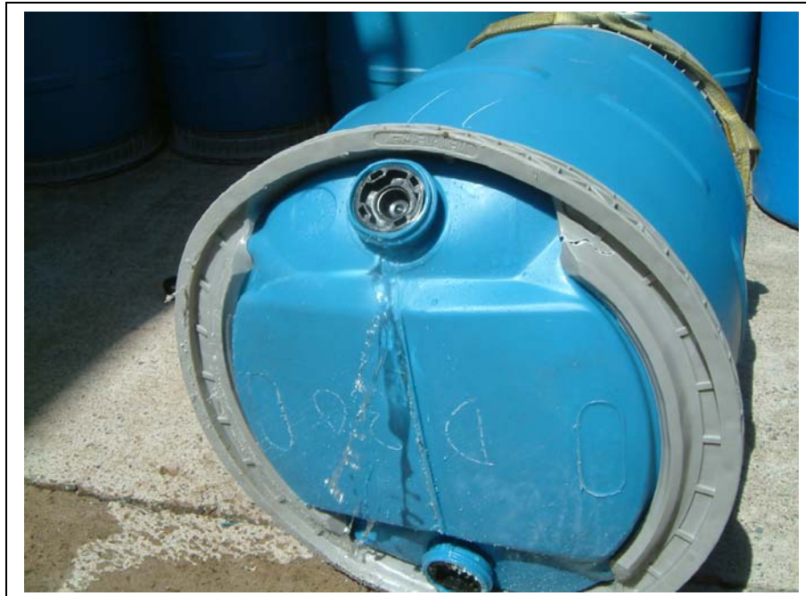
Photo 16 Drum Set D: Failure mode - Small split on closure neck (opposite from impact side)
