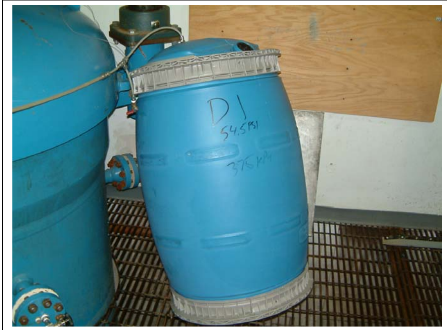
Photo 19 Drum Set D: Pressure test at maximum pressure
