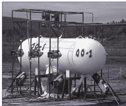
Test set-up for PRV trials
