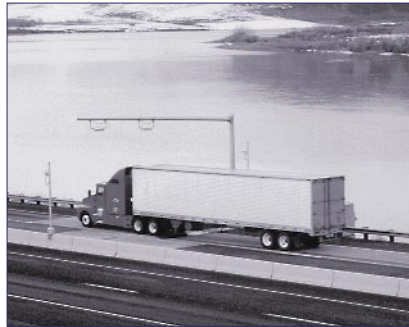
One of the trucks in the Green Light Project passing under the transponder readers that allow in-transit weighing and preclearance
