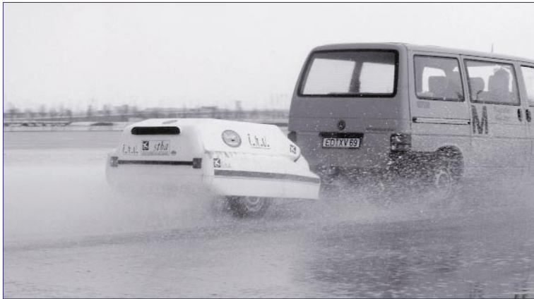
Reference ground friction measuring vehicle being used in the development of an international runway friction index
