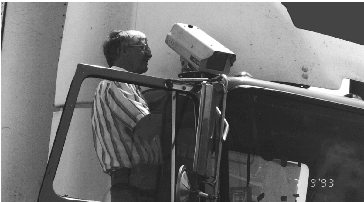
Figure 2. Lane tracker mounted on roof of truck cab
