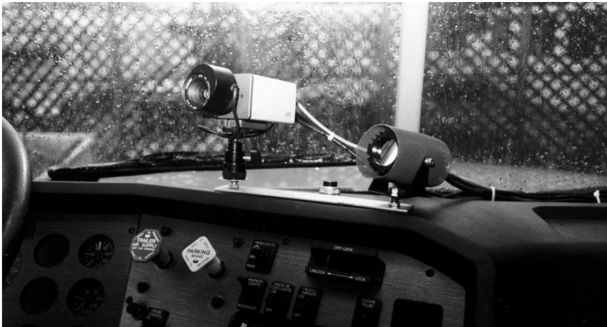
Figure 3. Face camera and infrared illuminator
