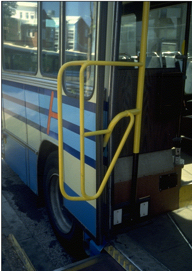
Figure 6 Handrails that extend beyond the entrance of a Swedish transit bus
