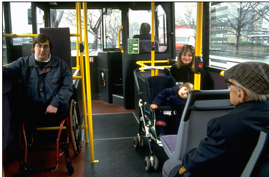
Figure 19 Interior of a low-floor bus, showing the compartment for a wheelchair on the left and space for a baby stroller or shopping cart on the right (Photo: London Transport)
