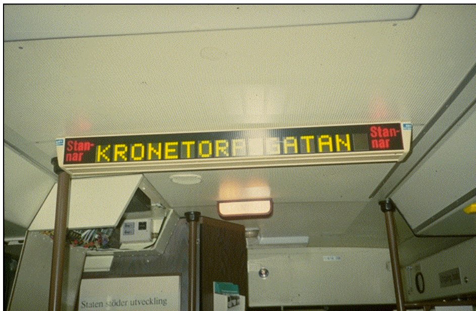
Figure 8b Display of the name of the next stop in a bus in Malmo, Sweden
