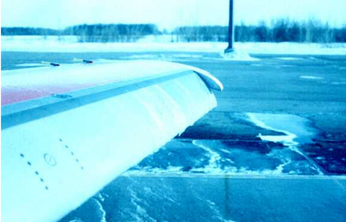
Photo 4.9 Run 3 (33% Failure) Ice on Extended Leading Edge Slat – Following Takeoff Run
