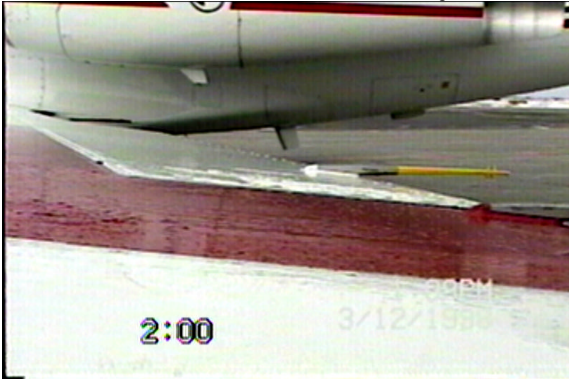
Photo 4.1 Run 1 (Initial Failure) Ice on Outboard Aileron - Following Takeoff Run
