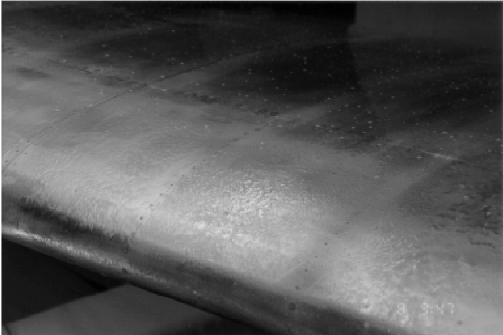
Figure 7a Type III Brand B (anti-icing) fluid with 25 minutes of snow contamination
