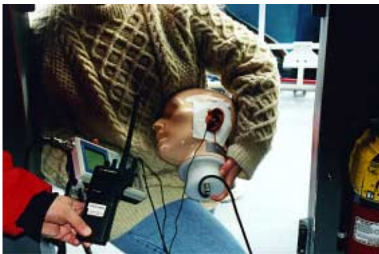
Figure 5: Data Collection with Electro-acoustic Communications Devices using Kunov Head on the CCGC W. Jackman
