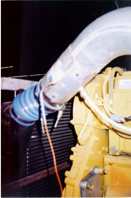
Figure A-4b: CWI between Air-to-Air Charge Cooler and Intake Manifold
