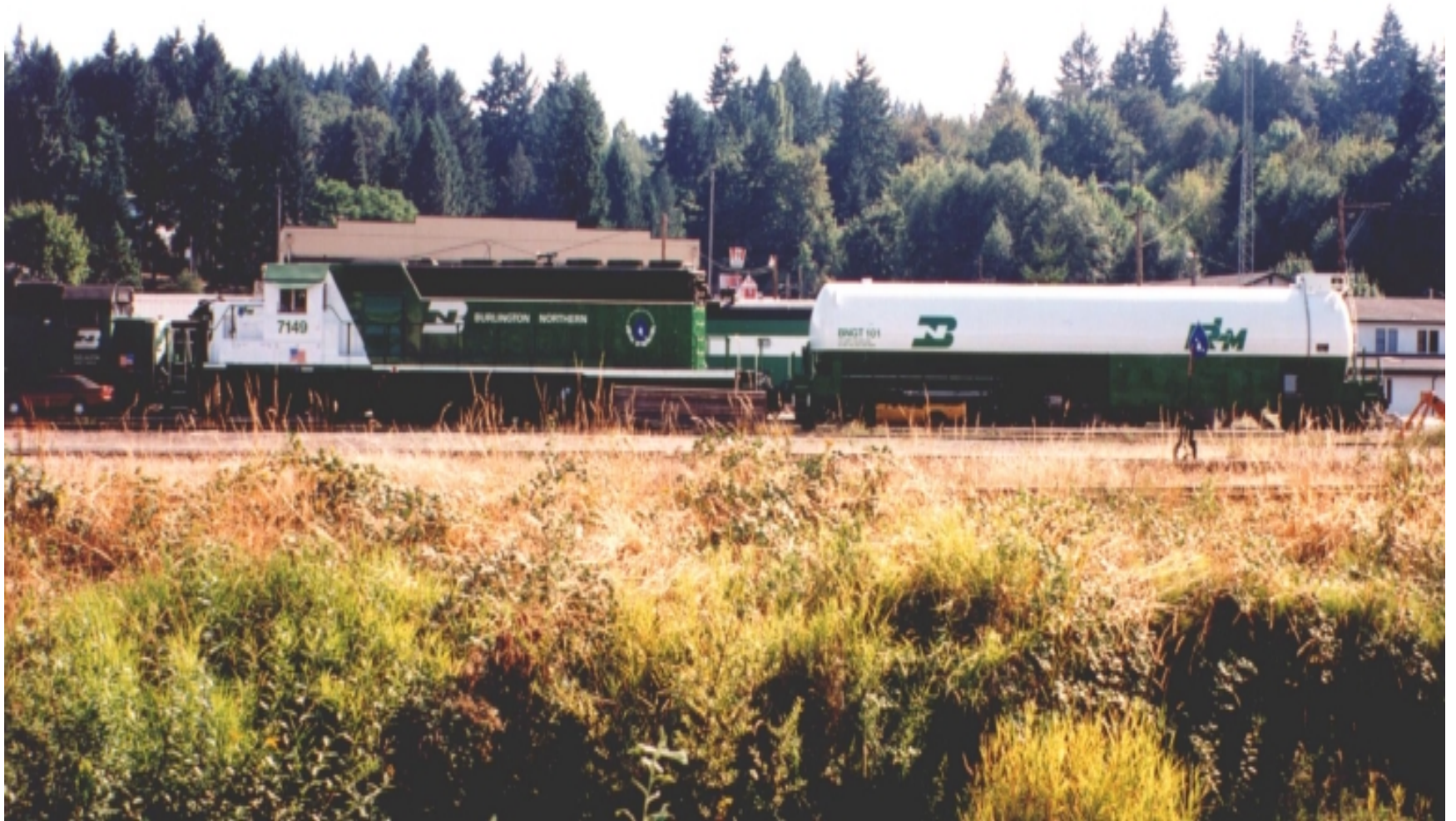
Figure 4: BN's Dual-Fuelled Locomotive and Its RLM Tender Car
