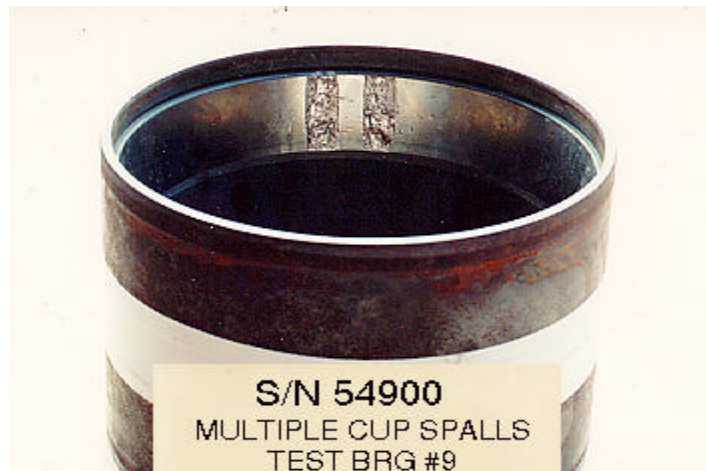
Figure 7: Multiple Cup (outer race) Spalling
