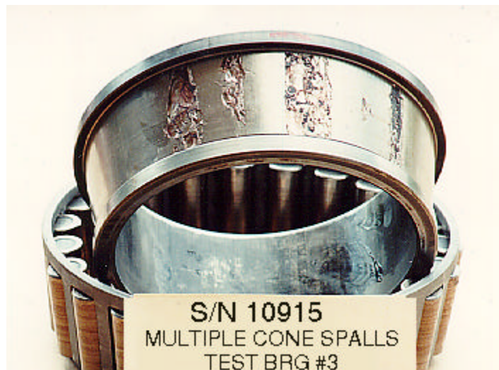
Figure 5: Multiple Cone (inner race) Spalling
