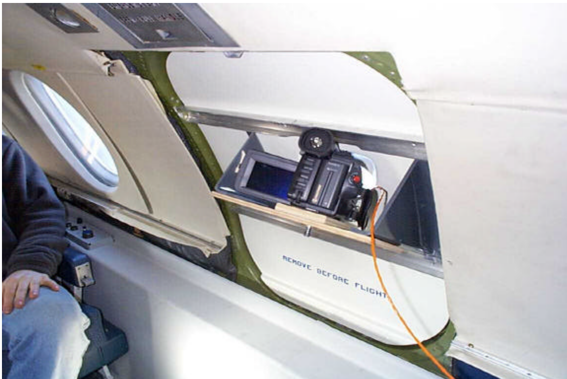
Photo 2.18 Video Camera Installation
