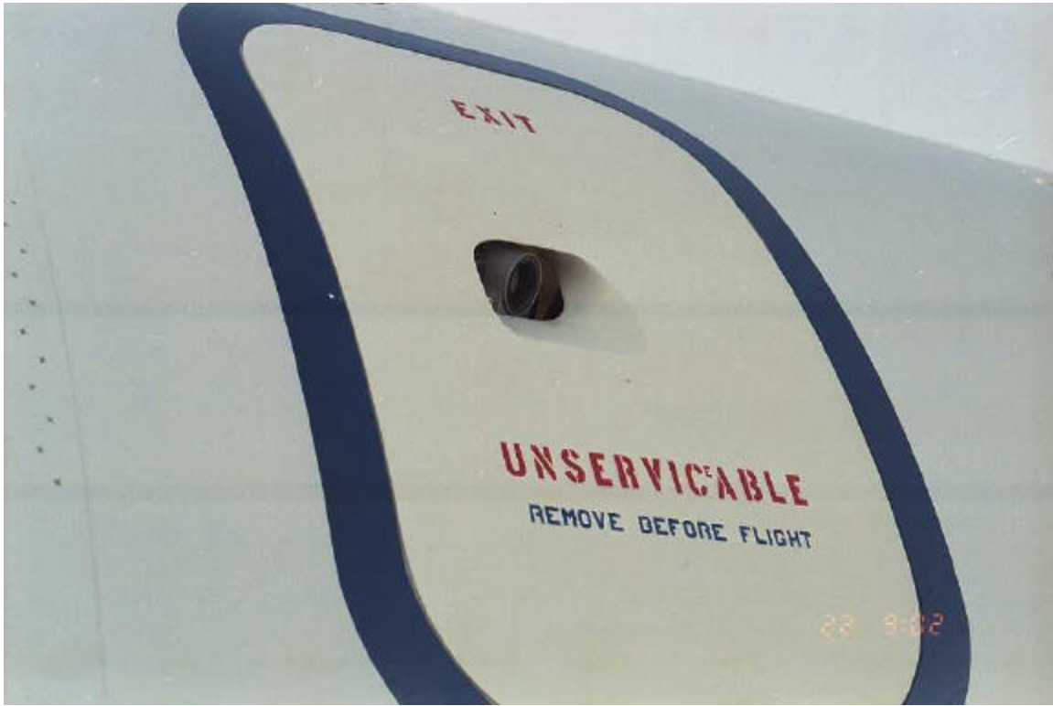
Photo 2.19 Video Camera Lens Trained on Test Area
