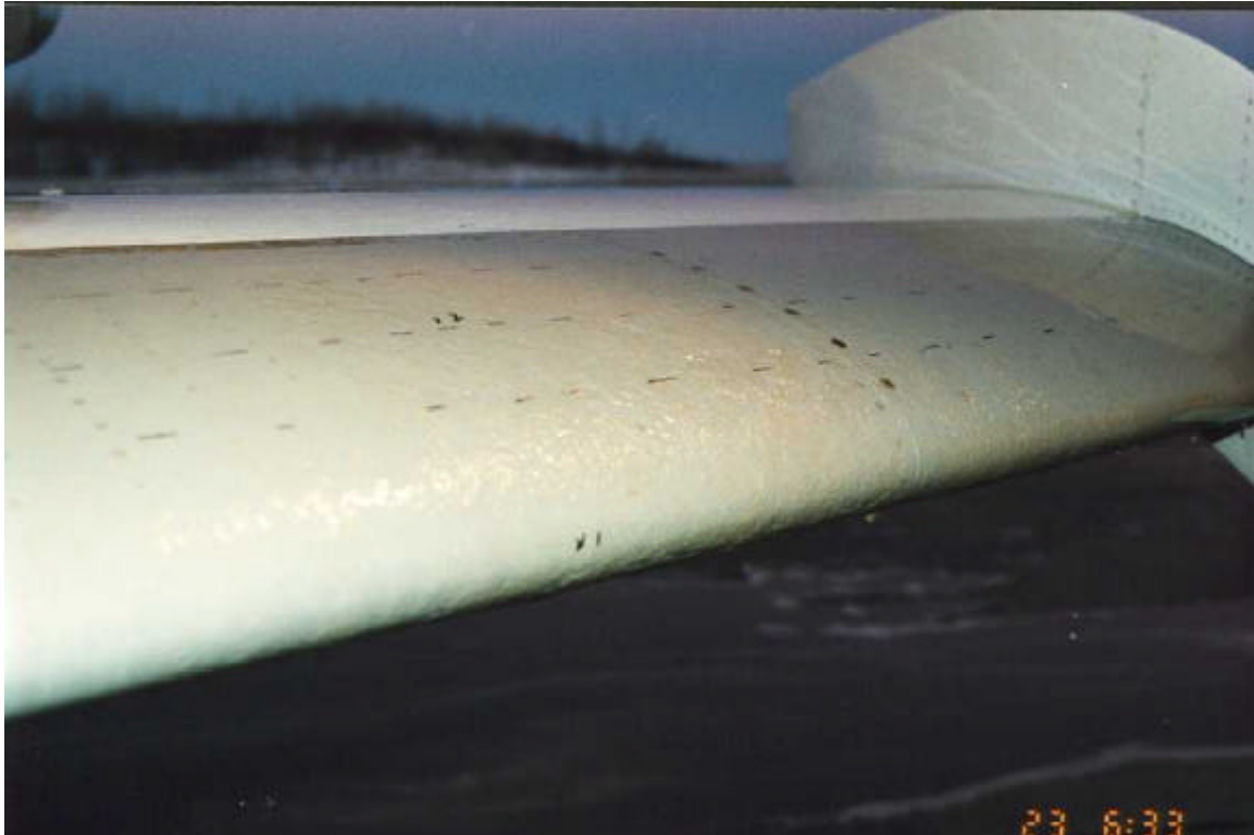
Failed Fluid on Leading Edge
