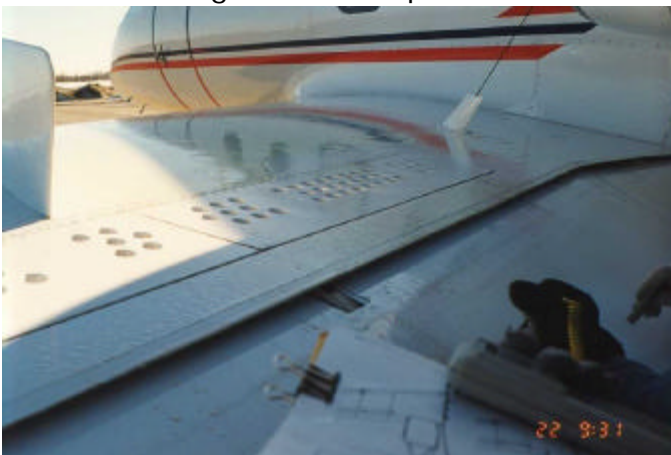
Puddling Ahead of Spoiler Panel
