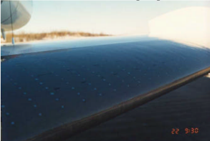
Thin Film on Leading Edge
