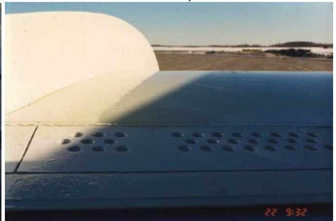
Fluid Ahead of Spoiler Panel
