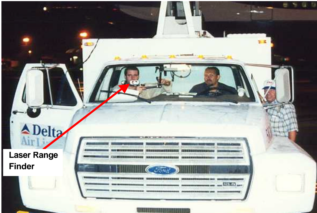
Photo 2.6 Front View of Laser Range Finder Inside Deicing Truck Cab
