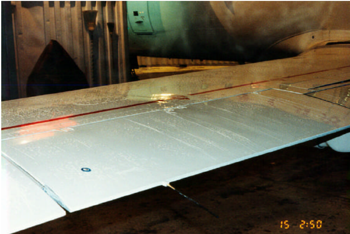
Photo 4.11 Overall Photo of the Frost Formation on the Aileron (ID# 3)
