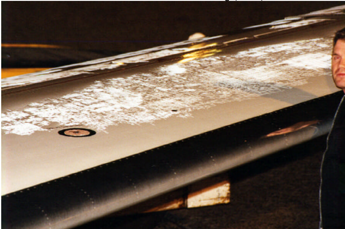
Frost Accumulation on Port Wing (ID# 1)
