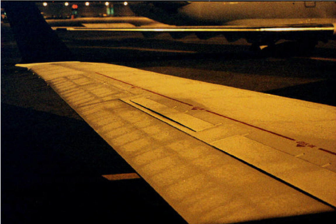
Photo 4.5 Frost Accumulation on Port Wing (ID# 2)
