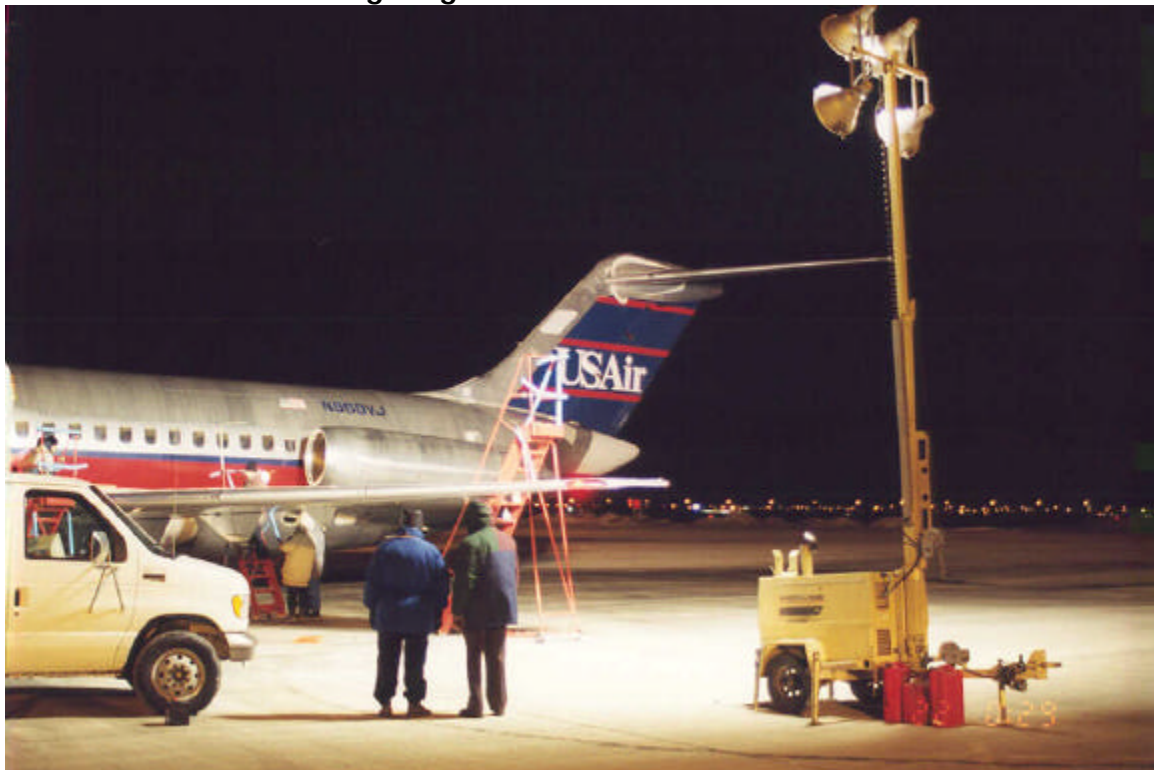
Photo 2.4 Mast-lighting Used for Aircraft Illumination
