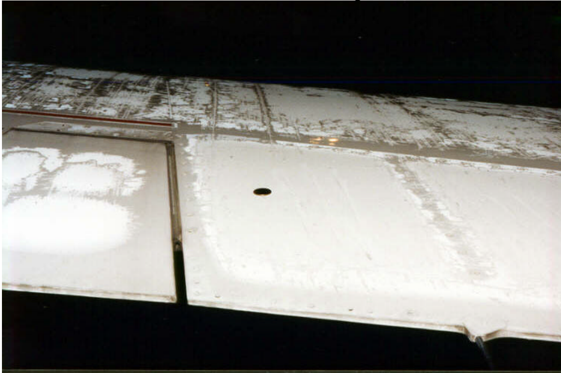
Heavy Frost Accumulation on the Aileron and Trailing Edge Outboard of the Aileron of the Starboard Wing (ID# 1)
