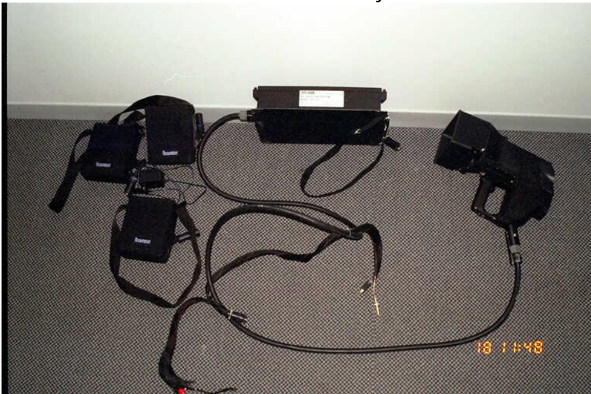
Photo 2.6 Hand-Held Ice Detection Sensor by RVSI ID-1H
