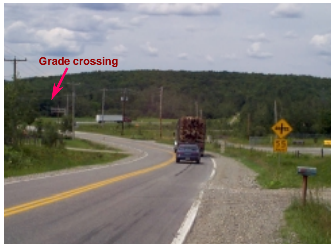
Downhill approach to a grade crossing requiring an automatic grade crossing advance warning sign
