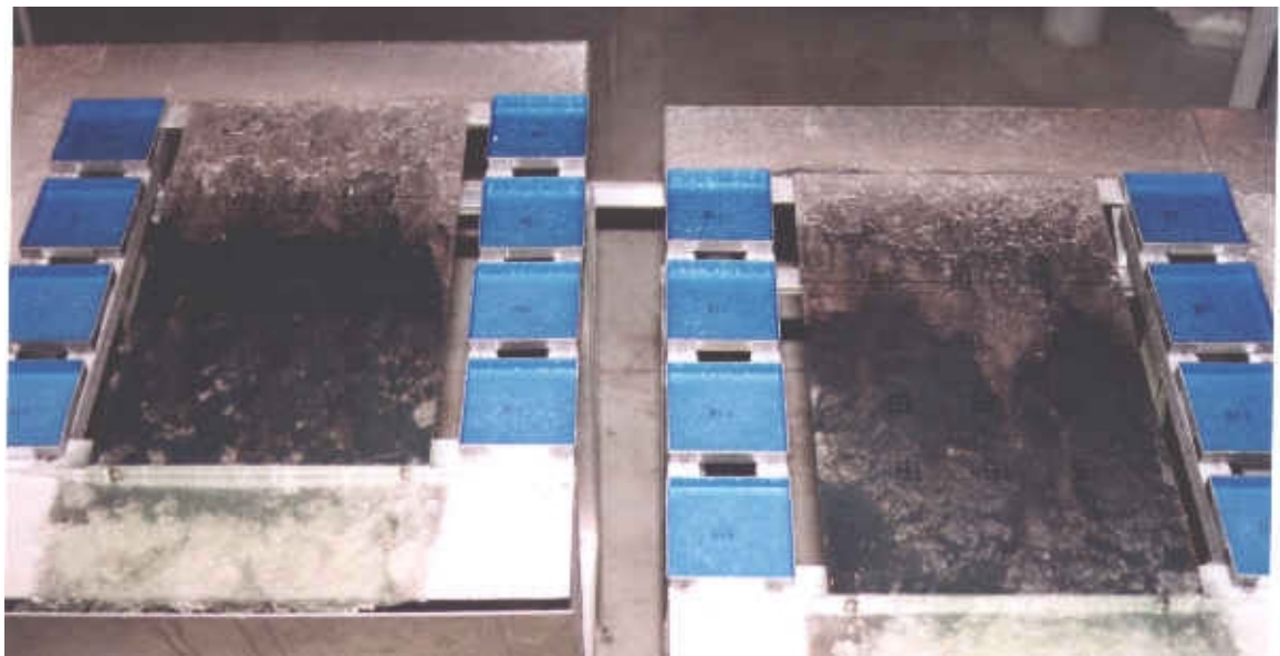
Figure 31: Ice Formation on Type IV Fluid
