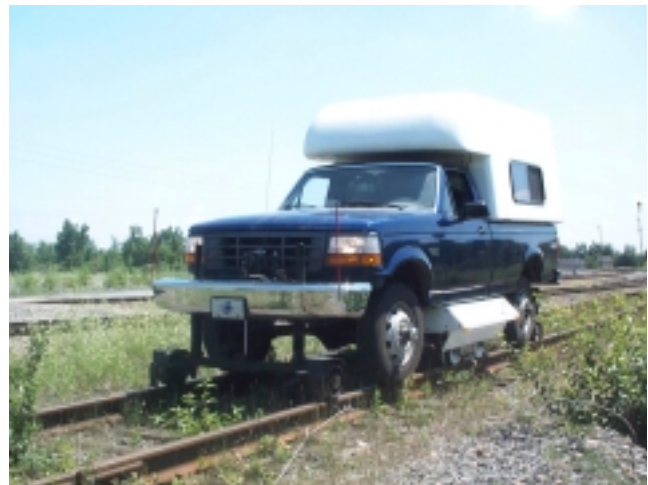
Figure 2 Integrated mobile inspection system
