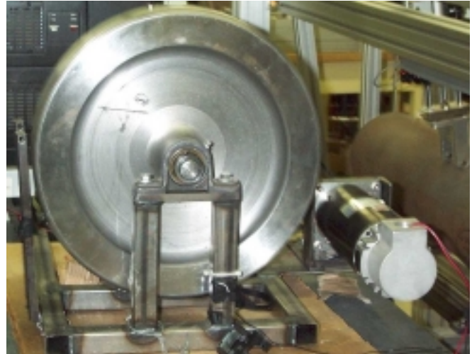
Figure 22 Flywheel used for dynamic tests in the laboratory environment
