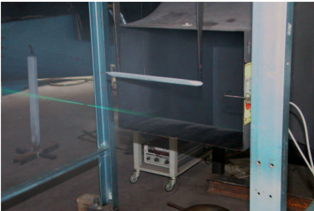
Figure 6: Experimental investigation of the rollup of the near wake emanating from a rectangular wing with A_R = 3.7 . Close view of the wing (top); view of the open test section and of the laser beam for LDV measurements within the rolling wake (bottom)
