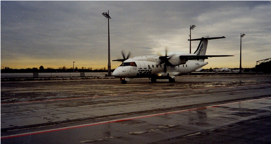
Figure 14. View of the Dornier D328-100 aircraft making a tare run on a freshly prepared and cleaned contaminated strip on 24 February 2000. Note the meltwater formed on the pavement after several runs.
