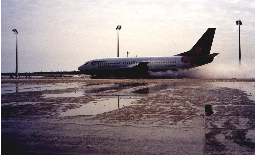
Figure 9. Ground level view of Deutsche British Airways Boeing B737-300 aircraft during the second run on Tuesday 22 February 2000
