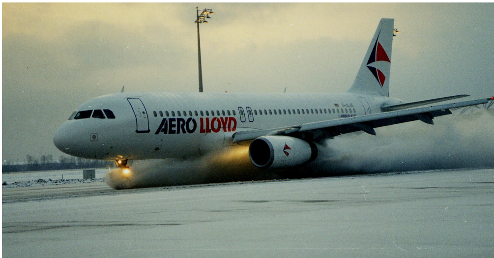
Figure 6. View of Aero Lloyd Airbus A320-DALAE aircraft during a braking run on Monday 21 February 2000. Note the freshly fallen snow in the foreground.
