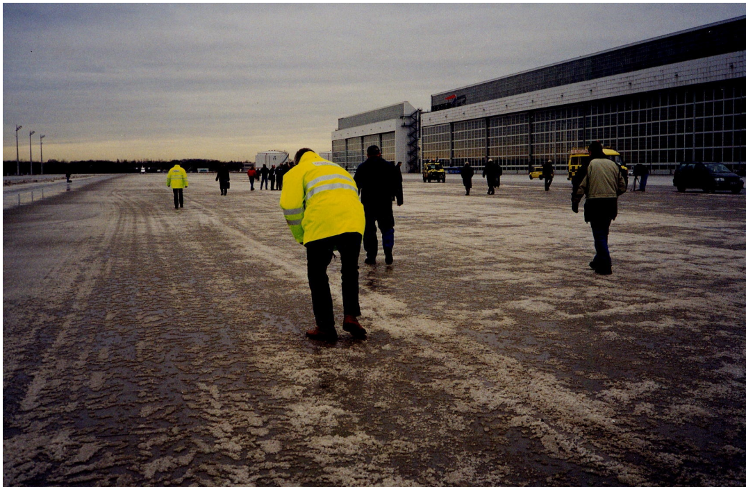
Figure 13. Manual cleaning action of picking up undesirable foreign objects from the strip before the commencement of the Dornier D328-100 aircraft test on 24 February 2000. Note the tire marks left on the snow by the front loader that crushed the large ice particles.
