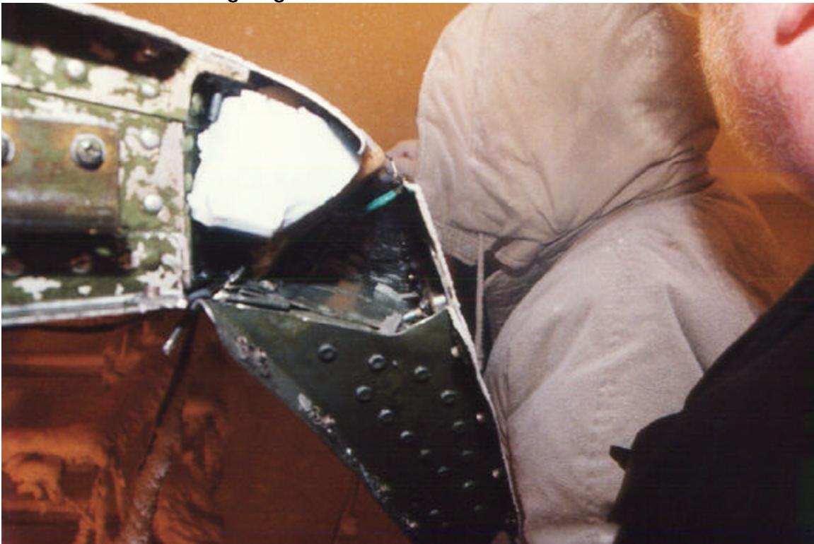
Photo 2.14 Leading Edge Slat Lowered to Examine Residue
