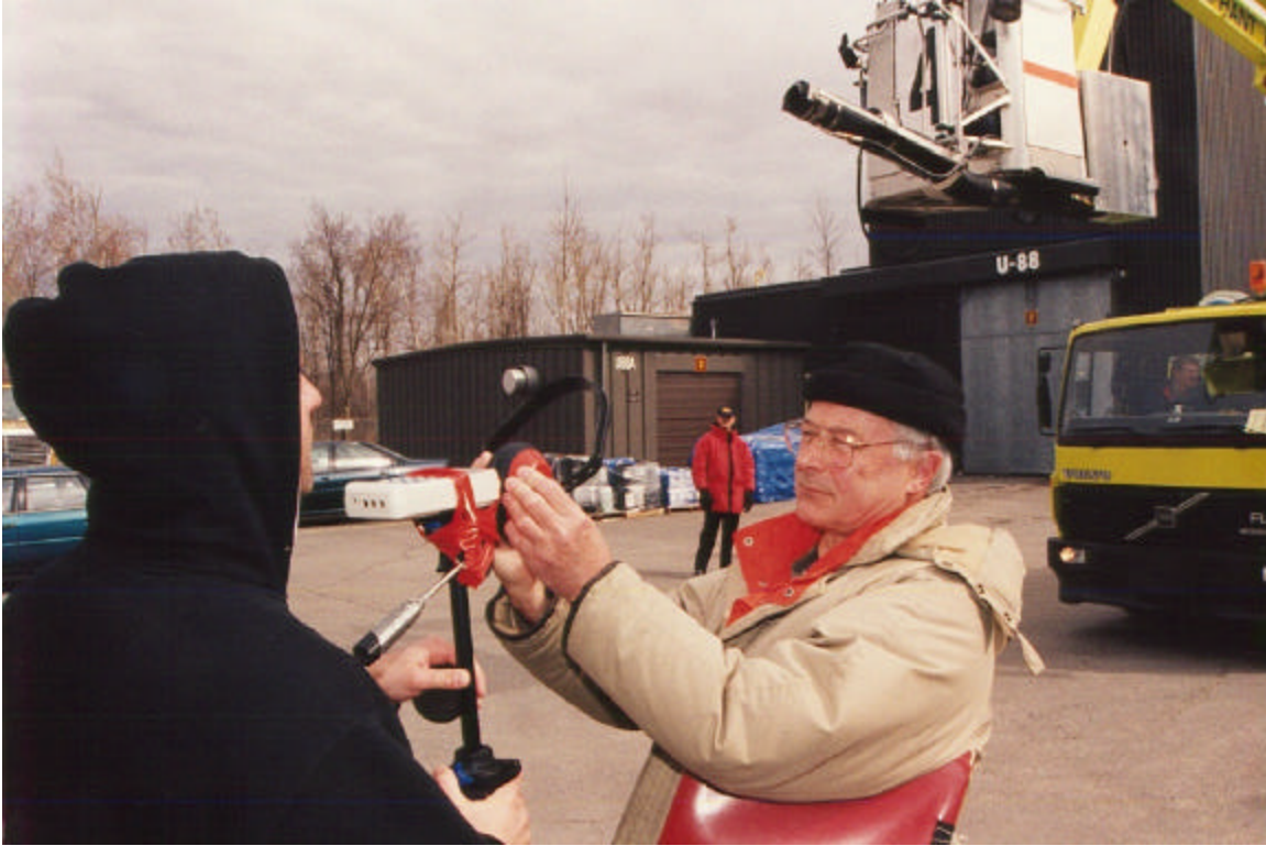
Photo 2.3 Noise Sensor Enclosed in Hearing Protector
