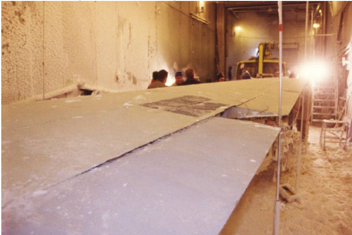
Photo 4.3 Wing Condition Following Air Deicing of Wet Snow
