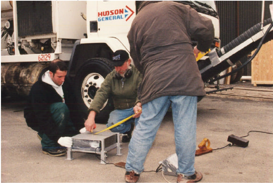
Photo 2.9 Adjusting Distance and Angle of Forced Air Stream
