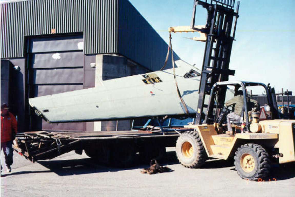
Photo 2.5 Removal of the Wing from the Transportation Vehicle
