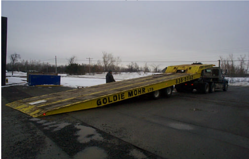
Photo 2.11 Flatbed Truck Moveable Ramp Used to Transport JetStar Wing and Wing Mounting System
