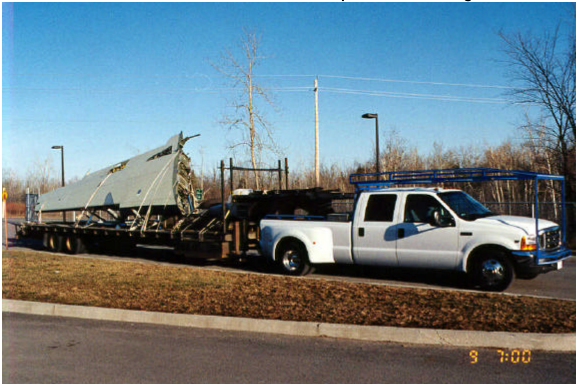
Photo 2.2 Truck and Trailer Used to Transport JetStar Wing
