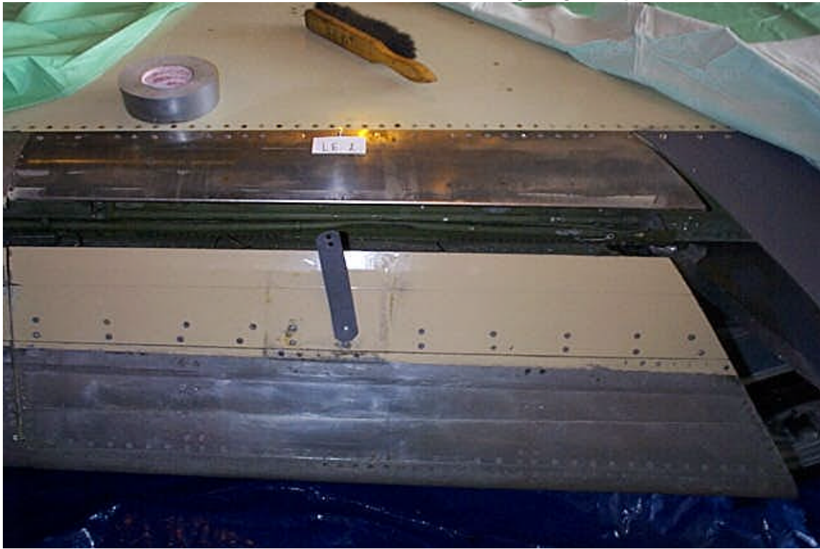
Photo 2.7 Bracket Used to Secure Leading Edge Flap
