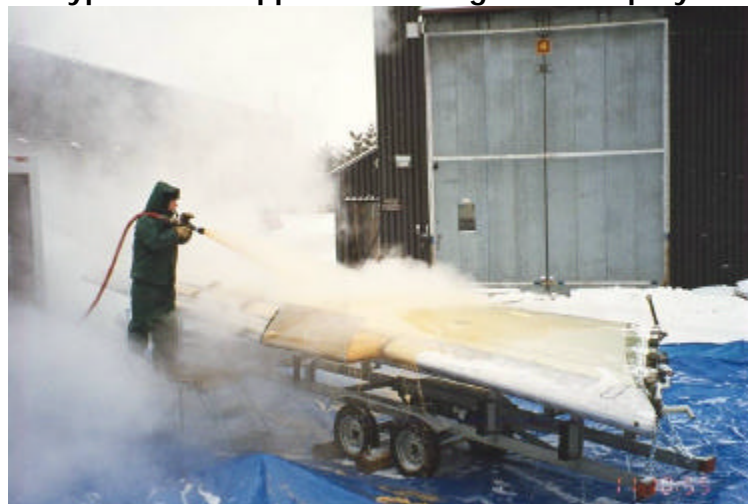
Type I Fluid Application using Mobile Sprayer
