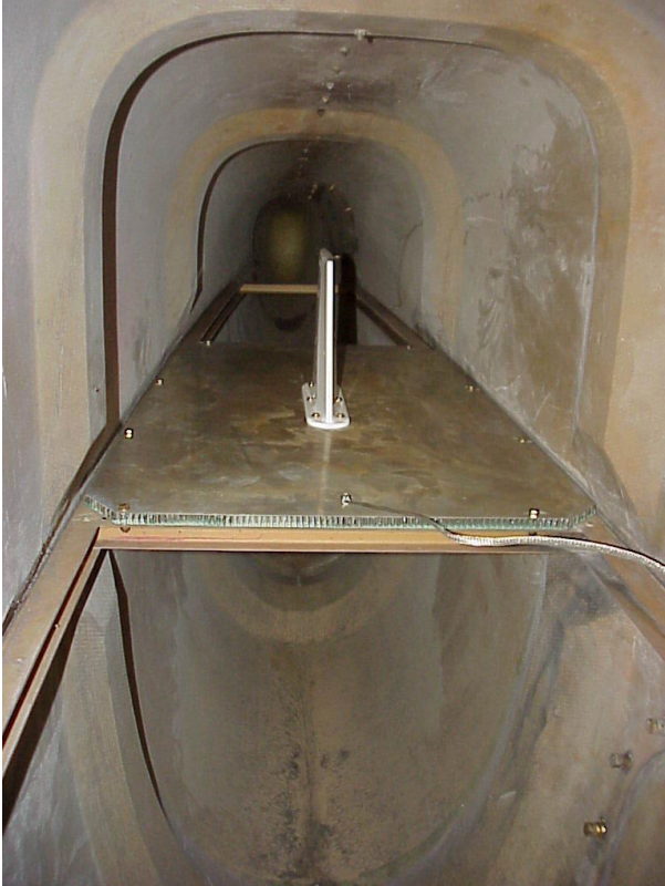
Figure 4: Antenna Mounted on Ground Plane Inside Tail Cone
