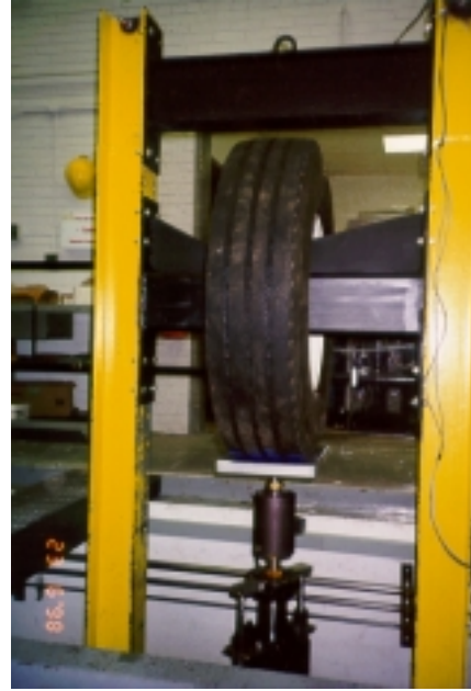
Figure 3.4: Tire test stand
