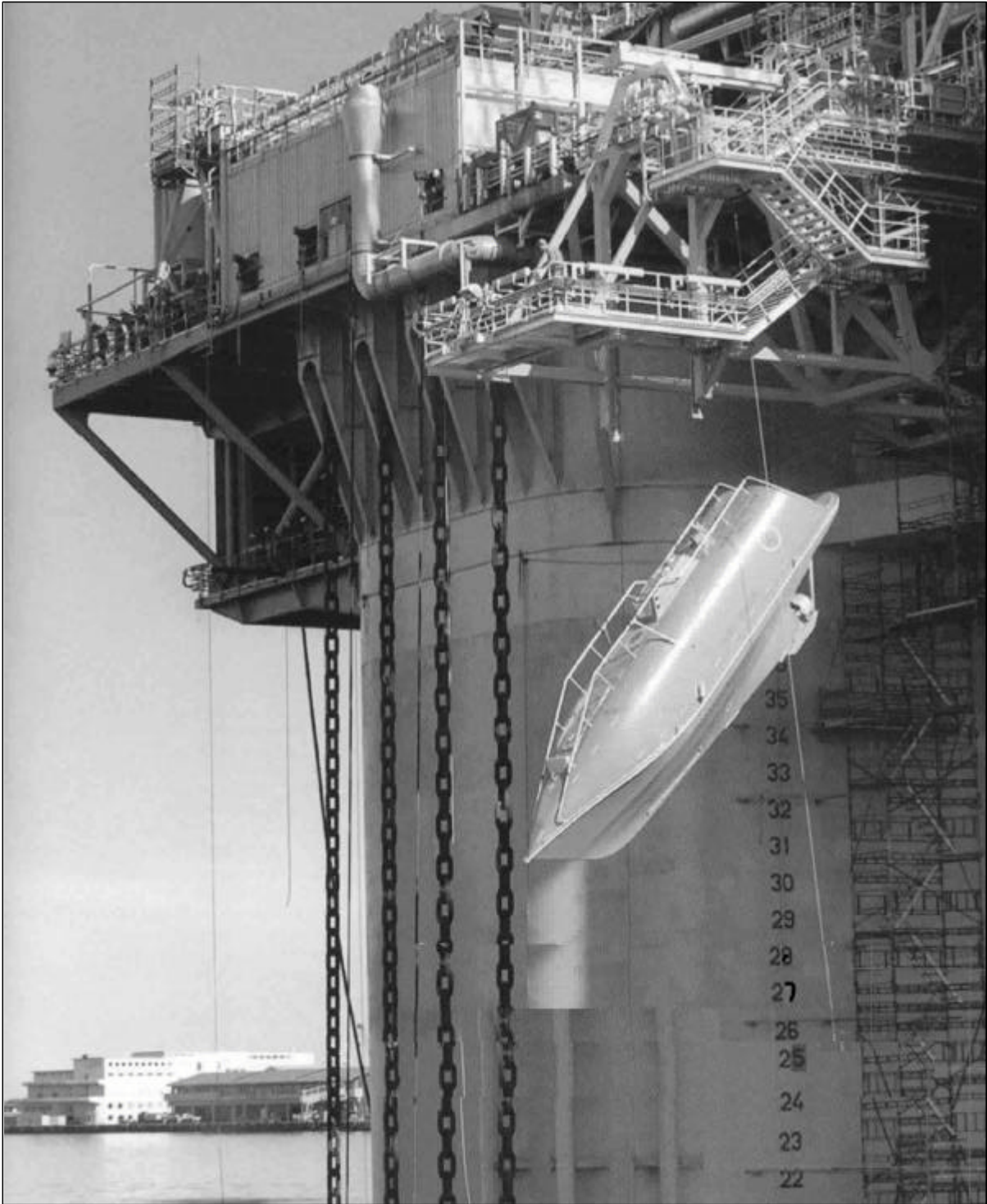
Figure 2.7 Vertical drop boat (courtesy of Umoe Schat-Harding)
