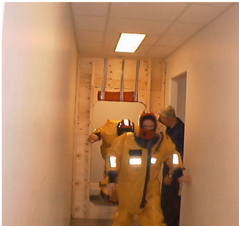
Figure 4.9 Walkway experiments with hatch bottleneck
