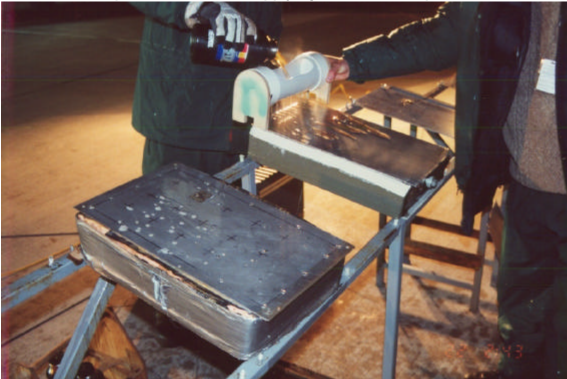
Photo 2.7 Proposed Method for Applying Fluid with a Spreader
