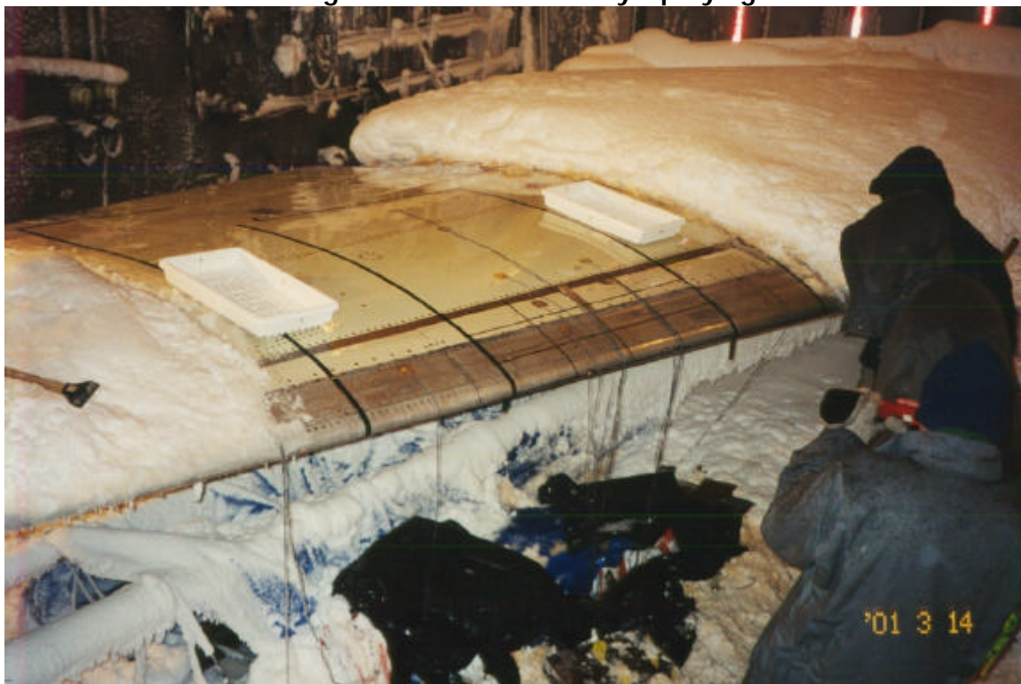
Photo 2.12 Wing Test Area Cleaned by Spraying
