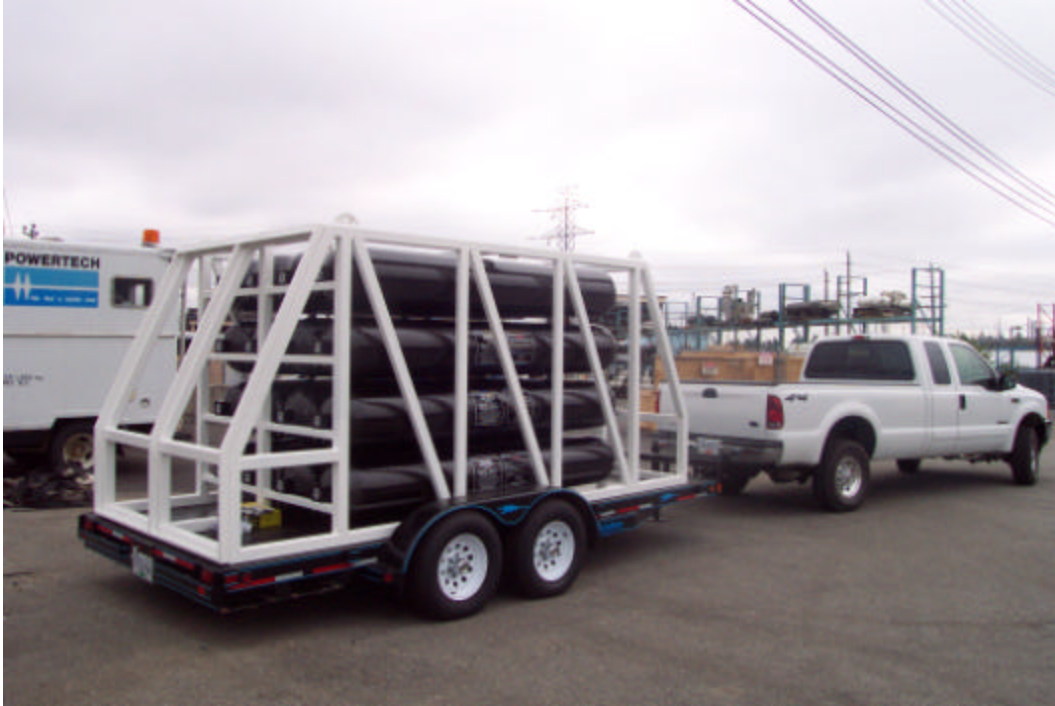
Figure 3 Support framework for transportable container unit of Dynetek cylinders
