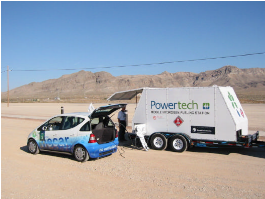
Figure 4 Complete transportable container unit being used to refuel a fuel cell vehicle
