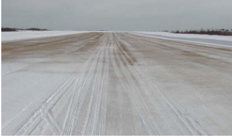
Figure 3.10: Test Surface January 16, 2002: Sanded Bare Ice on the Right, Sanded Compacted Snow on the Left
