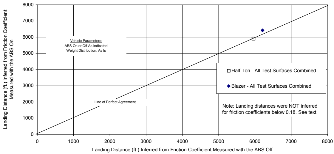
Figure 6.15: Effect on Inferred Landing Distances: ABS On or Off for the Bowmonk for All Test Surfaces Combined
