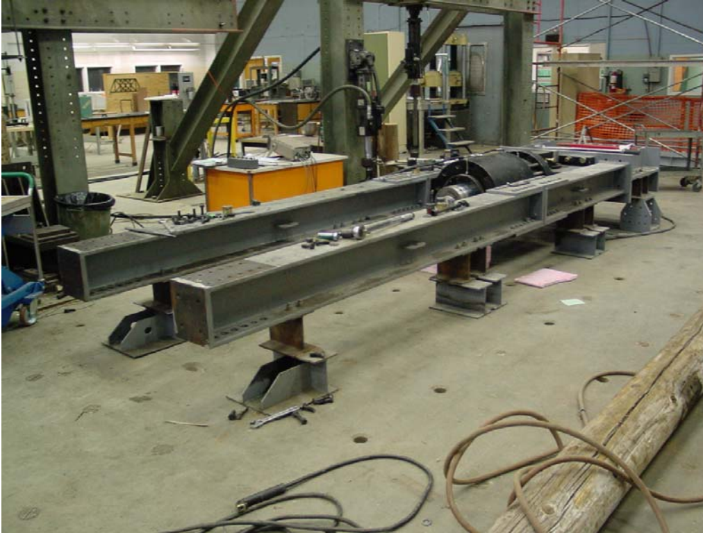
Figure 2. MUN Structures Lab showing a 600,000 lb. actuator in a frame being prepared for a test. The lab has a 3 ft. thick reinforced concrete floor slab with anchor points at 2 ft. centres (with access from below).
