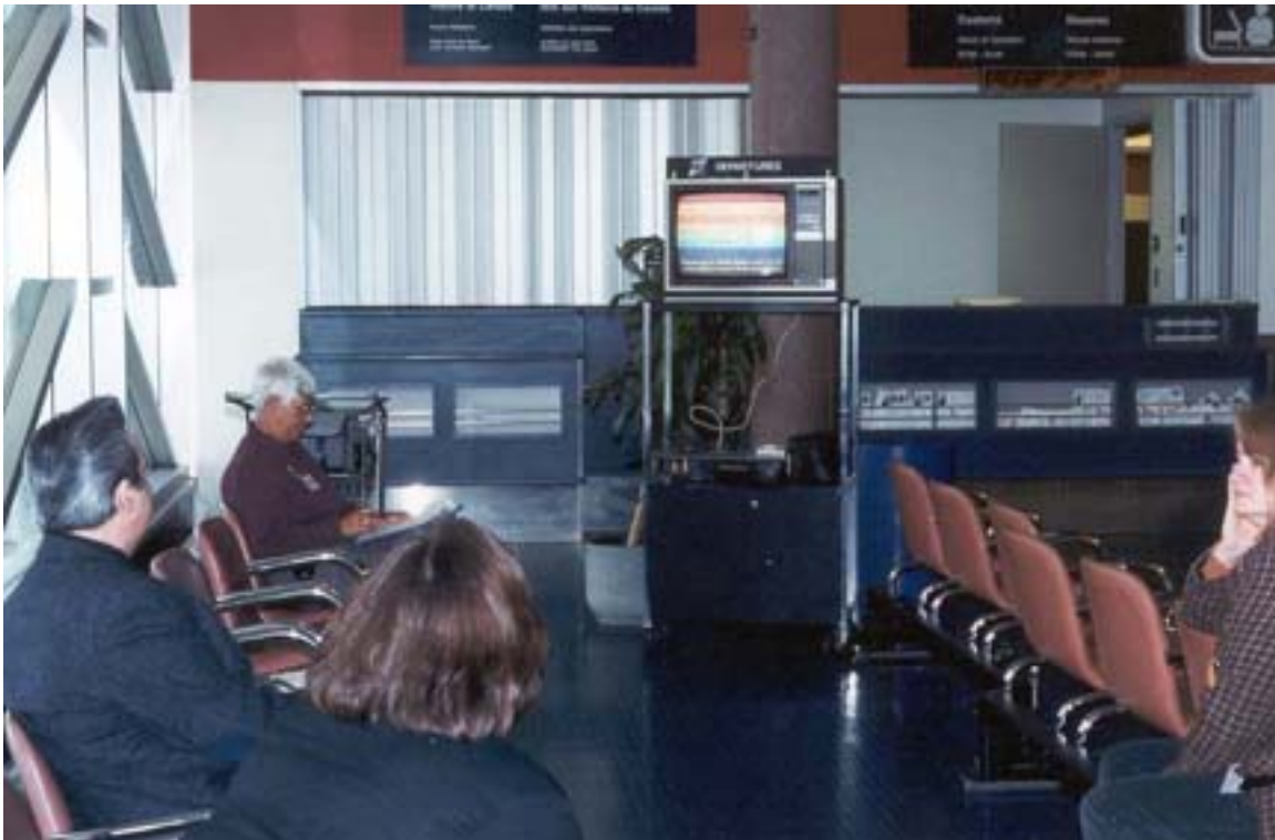
Figure 16: Test set-up for FID monitor mock-up at waiting lounge, international arrivals, Ottawa International Airport
