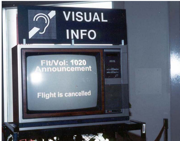
Figure 13: Close-up of text message shown on visual info monitor. Monitor panel showing international symbol for persons who are hearing impaired or deaf
