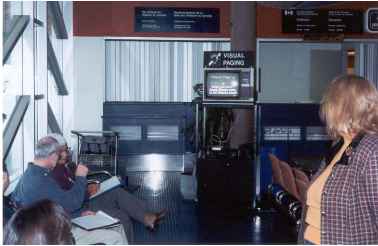
Figure 19: Test set-up for visual paging monitor at international arrivals
