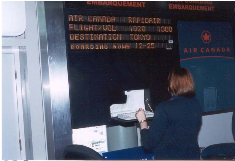
Figure 11: Electronic board display, data input by gate agent via laptop
