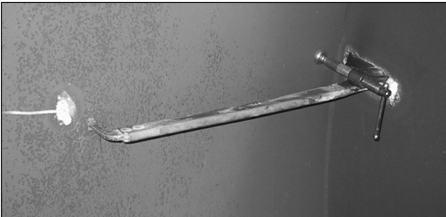
Figure 15: Back Side of Clamped Wall – Clamped at Thermocouple Location (Test 12)
