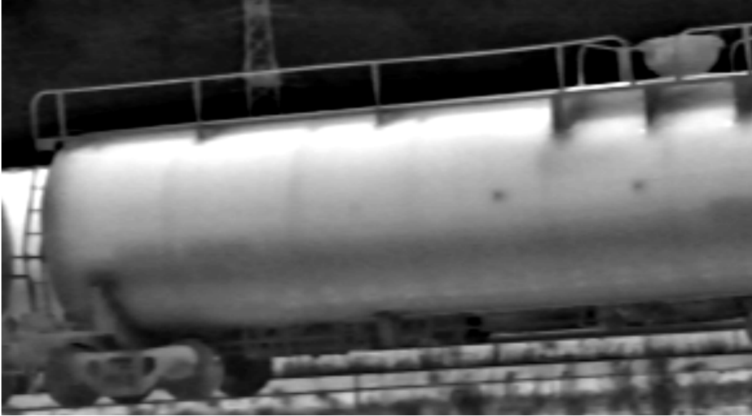
Figure 3: Tank-Car with No Thermal Protection Deficiencies (Thermal Image)
