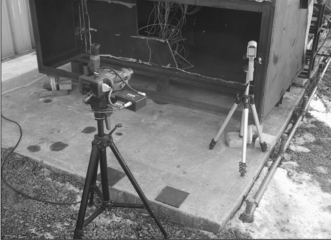
Figure 10: IR Camera (FLIR ThermaCAM SC 1000) and IR Thermometer (Raytek MX4)
