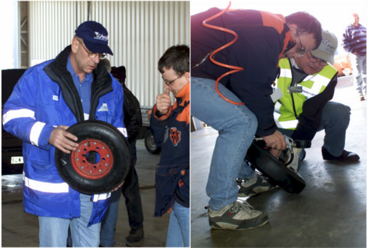
Figure 7. Changing tires to ASTM E1551
