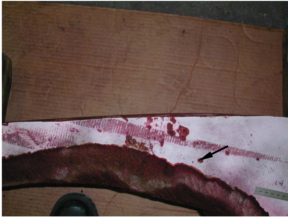
Figure 3.8: LPI Results on the HP Side of the Blade
