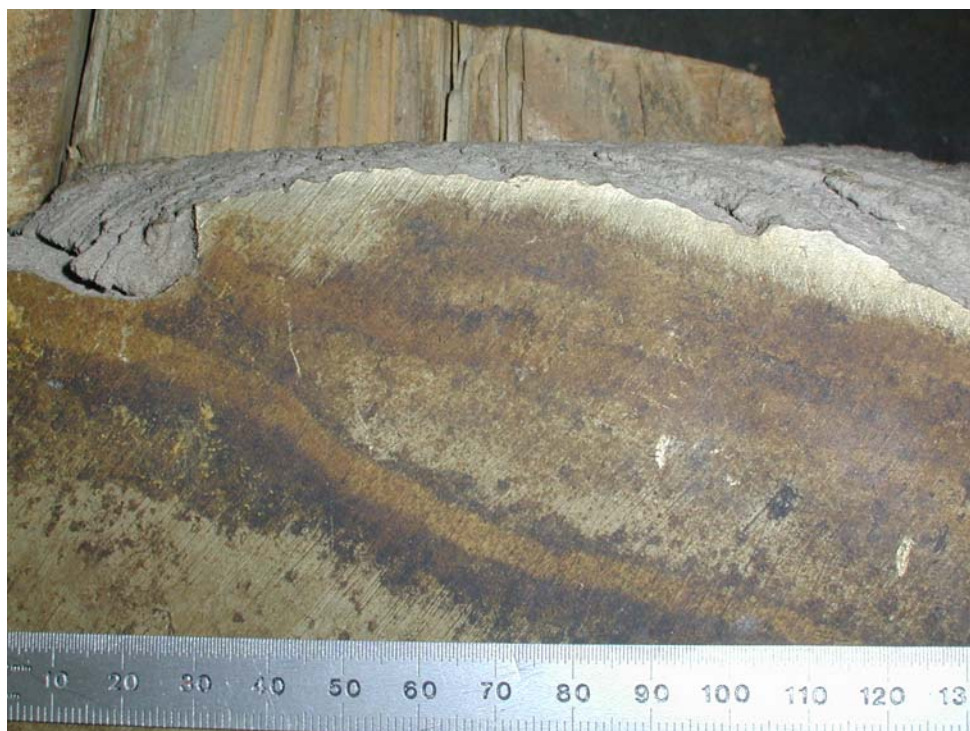
Figure 3.6: View of the HP Side of the Blade Adjacent to Fracture
