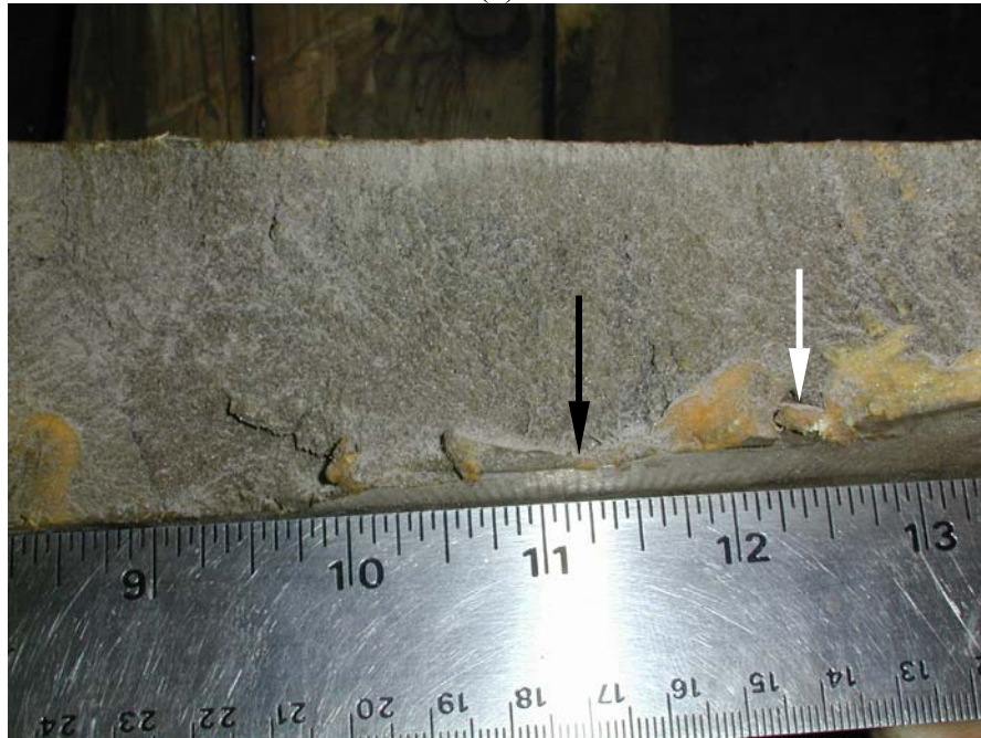
(b) white arrow points to a casting defect.
