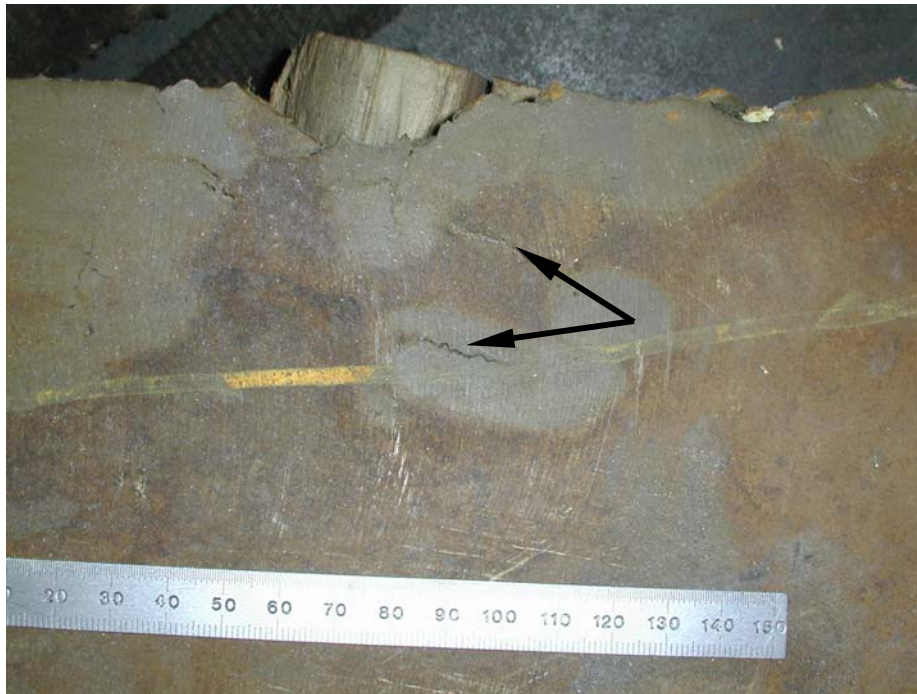
Figure 3.5: Examples of Cracks Close to the Fracture on the HP Side of the Blade
