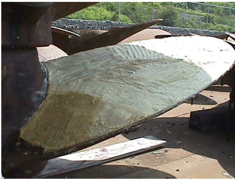
Figure 2.2: Mould on Propeller Blade
