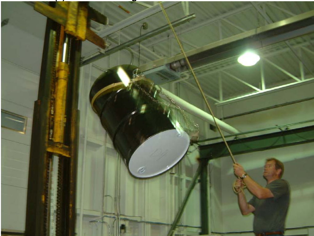
Photo 38 Lot D(4) Drum - Showing 6 O'clock Release from 3.6 Metres
