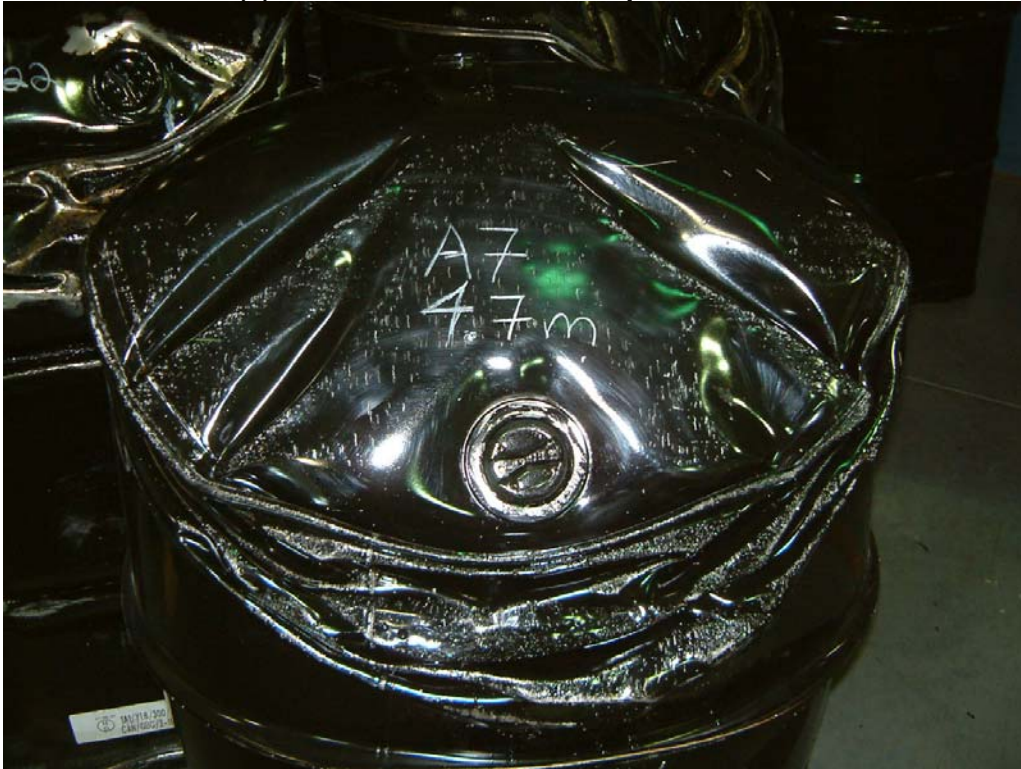
Photo 10 Lot A Drum Drop Setup for Heights Greater than 4.6 Metres
