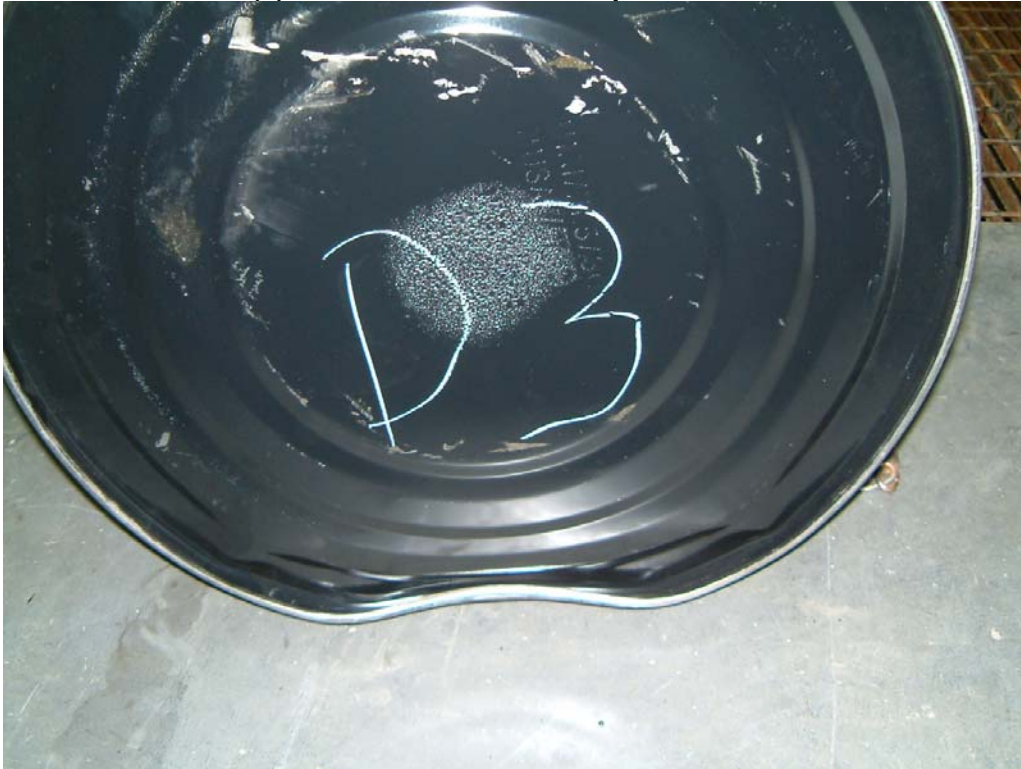
Photo 38 Lot D(4) Drum - Showing 6 O'clock Release from 3.6 Metres
