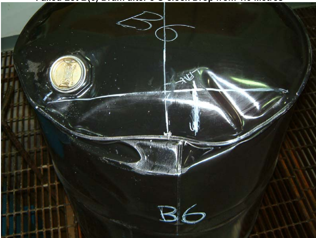
Photo 22 Failed Lot B(6) Drum after 8 O'clock Drop from 1.0 Metres
