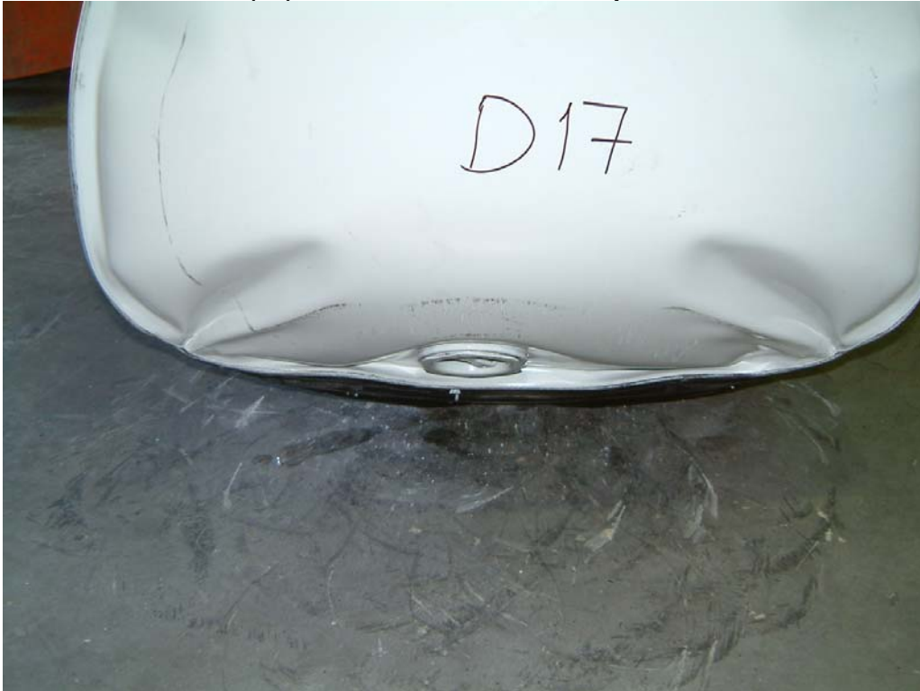
Photo 44 Passed Lot D(26) Drum after 8 O'clock Drop from 1.8 Metres
