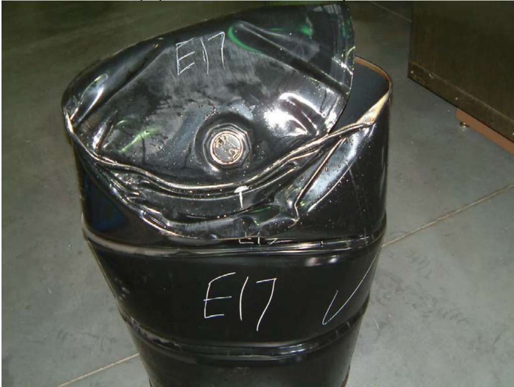
Photo 58 Failed Lot E(18) Drum after 6 O'clock Drop from 4.2 Metres
