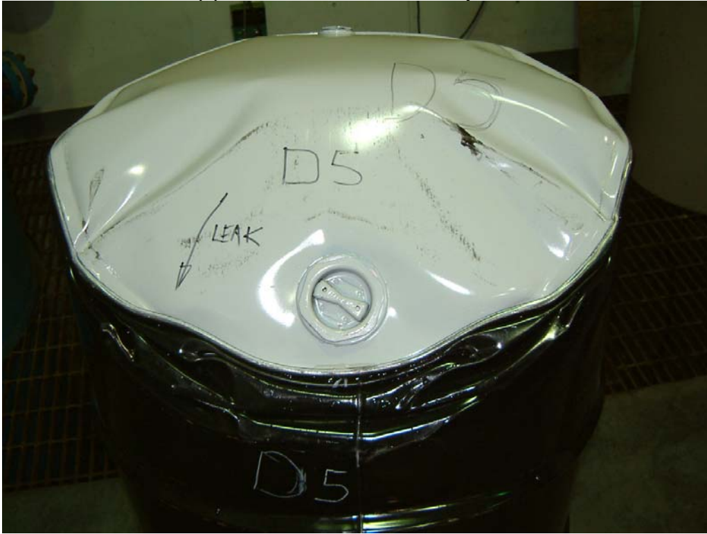
Photo 40 Failed Lot D(11) Drum after 6 O'clock Drop from 2.8 Metres
