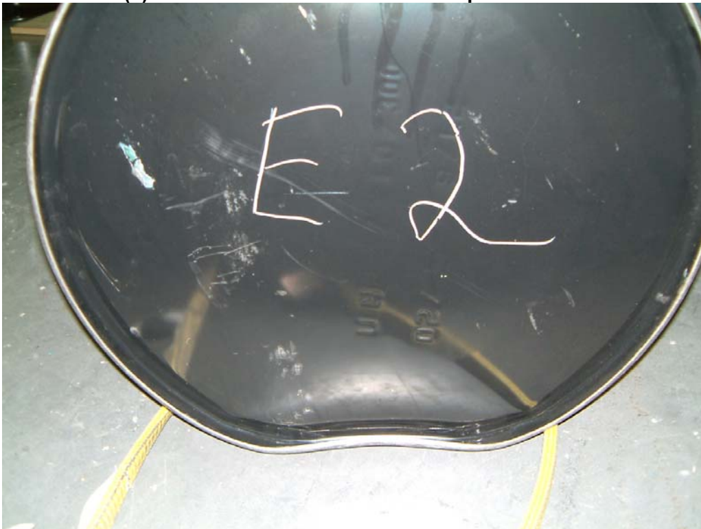
Photo 50 Lot E(2) Drum Bottom after 6 O'clock Drop from 2.0 Metres
