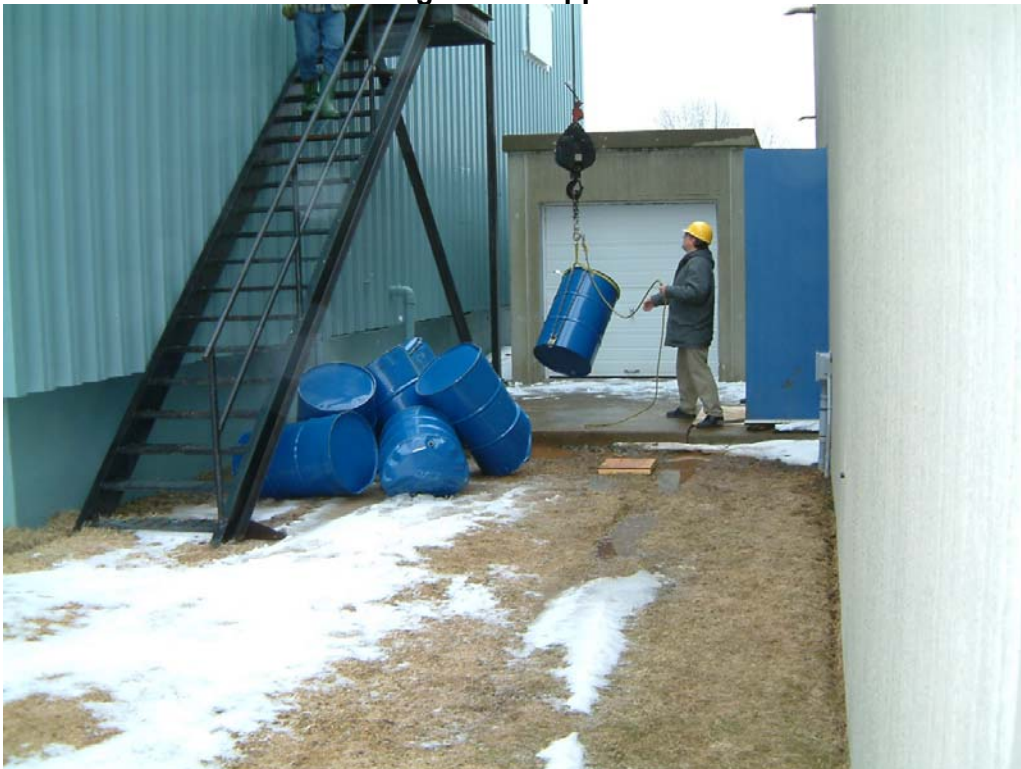
Photo 78 Lot F Drums Showing Drum Support and Release Hook
