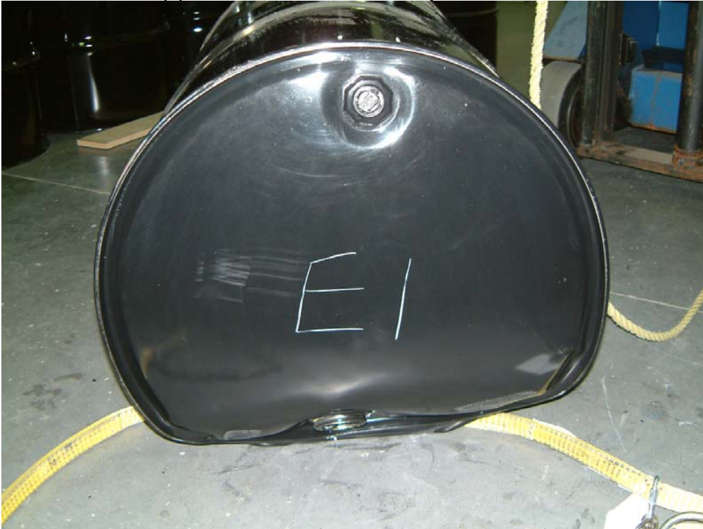
Photo 48 Lot E(2) Drum Showing 6 O'clock Drop from 2.0 Metres
