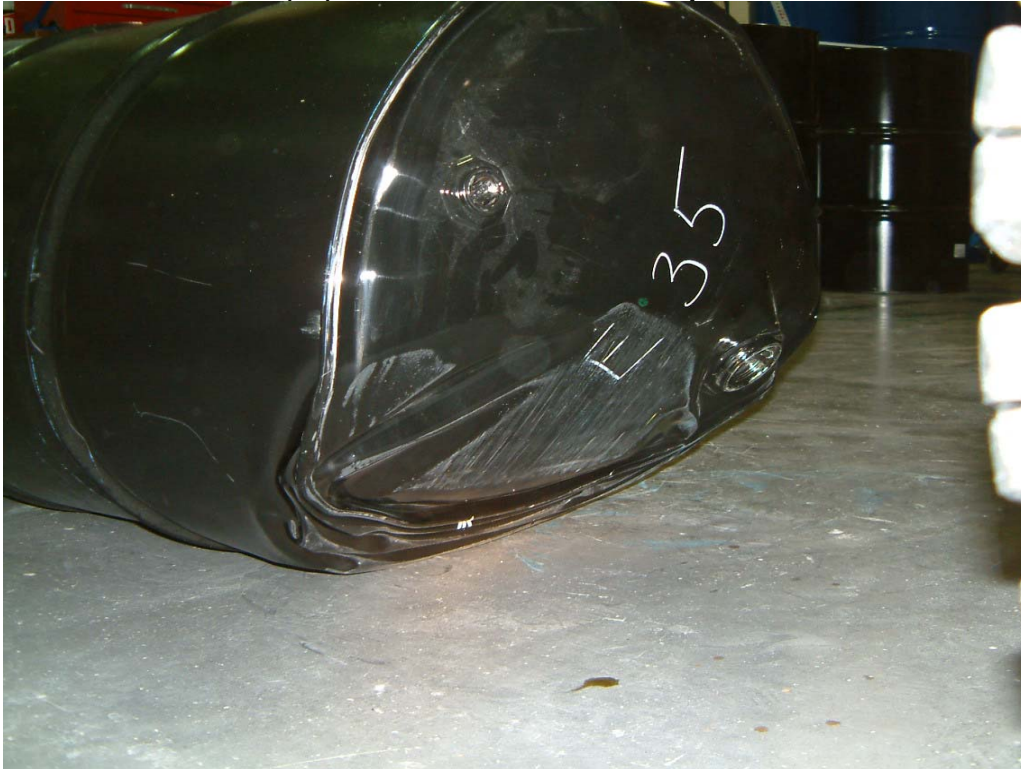
Photo 64 Failed Lot E(43) Drum after 8 O'clock Drop from 3.4 Metres
