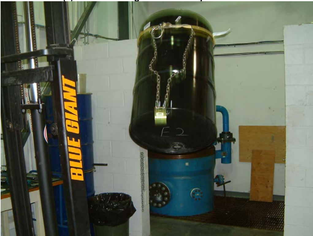
Photo 48 Lot E(2) Drum Showing 6 O'clock Drop from 2.0 Metres
