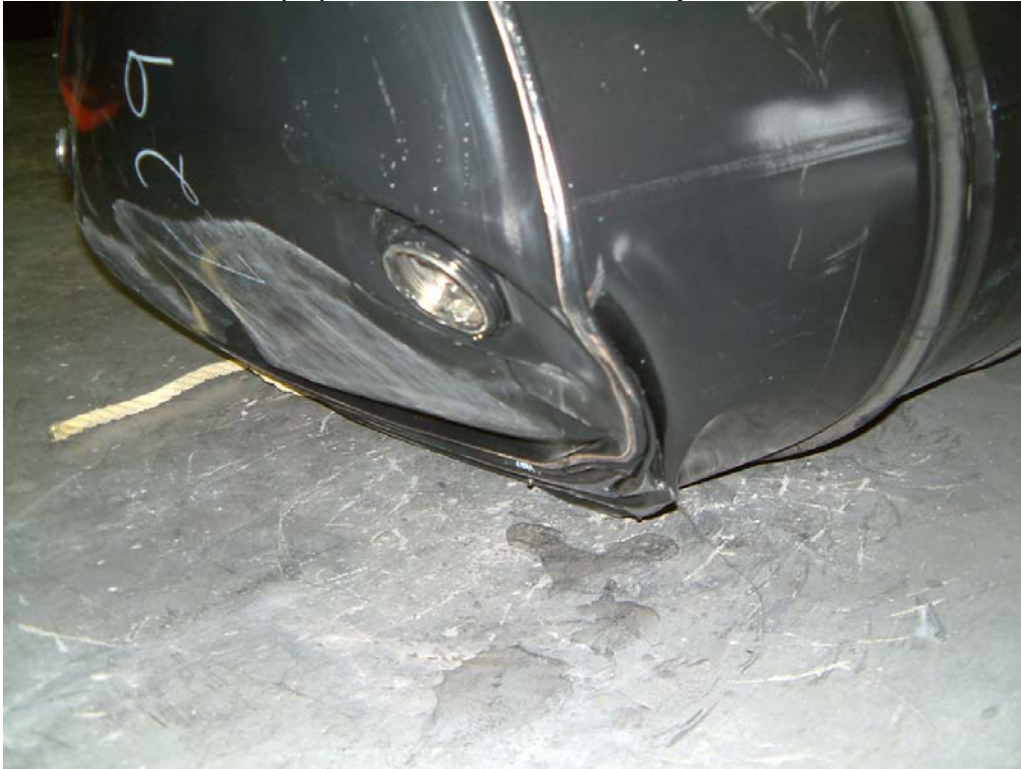
Photo 62 Failed Lot E(32) Drum after 8 O'clock Drop from 3.6 Metres
