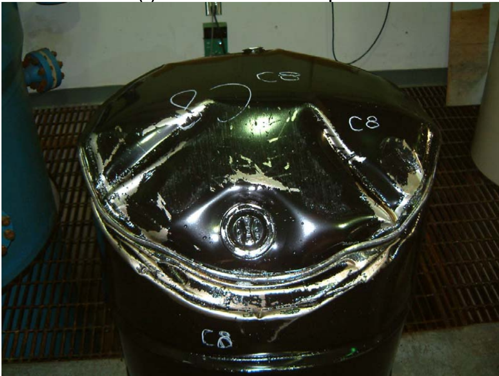
Photo 30 Failed Lot C(8) Drum after 6 O'clock Drop from 3.4 Metres
