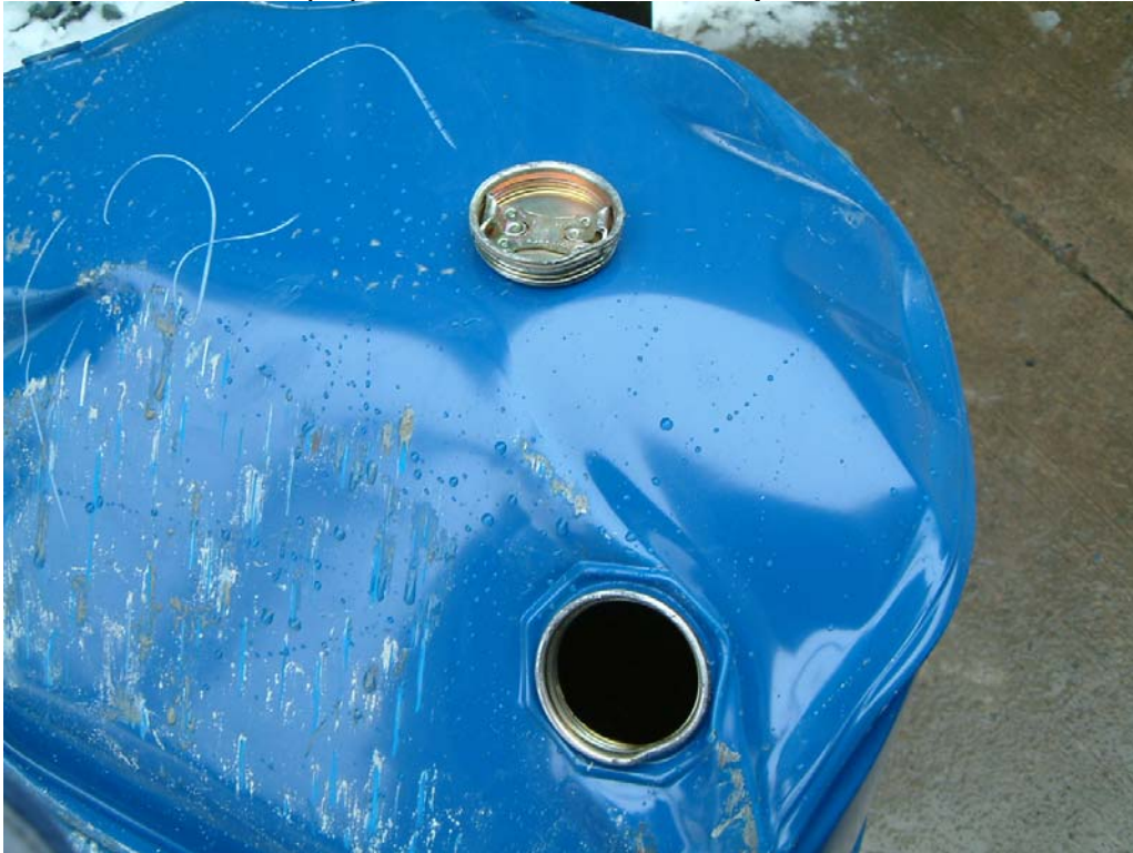
Photo 74 Cap from Lot F(27) Drum after 8 O'clock Drop – 4.8 Metres
