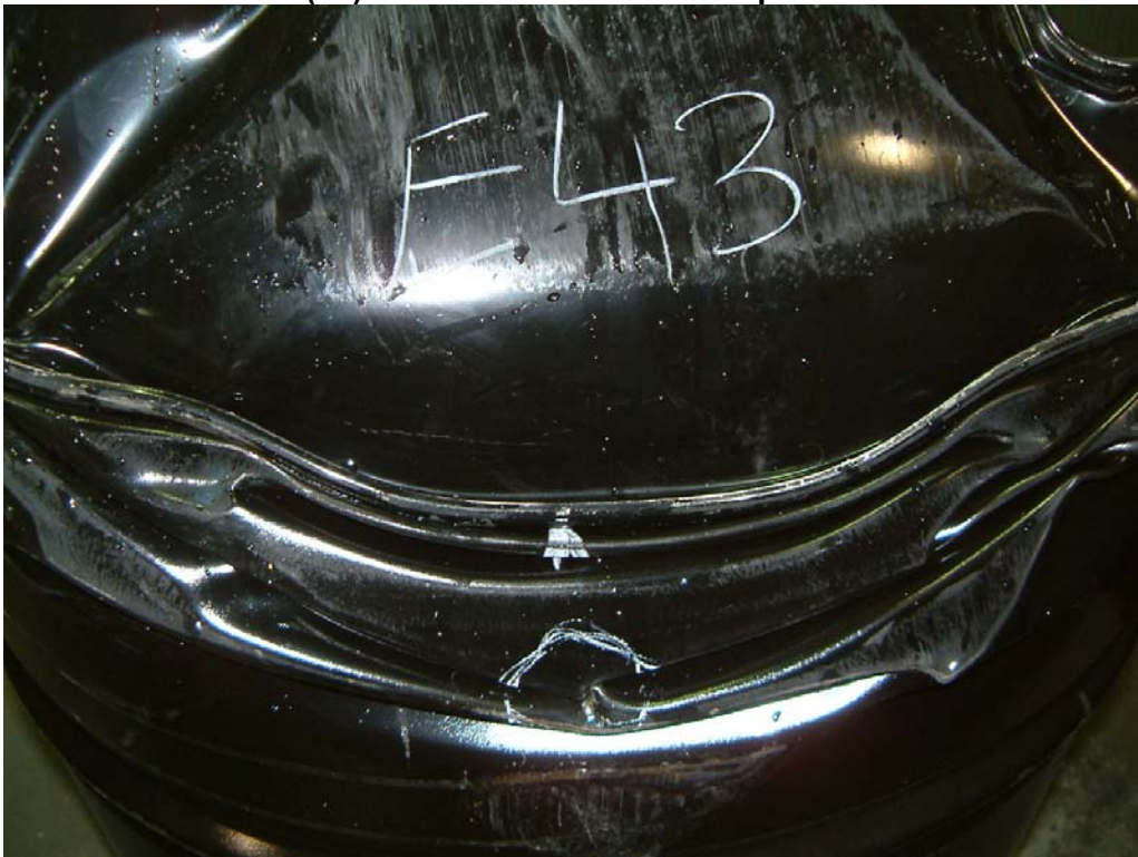
Photo 64 Failed Lot E(43) Drum after 8 O'clock Drop from 3.4 Metres
