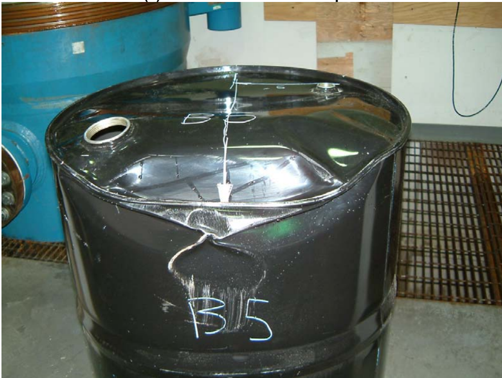
Photo 22 Failed Lot B(6) Drum after 8 O'clock Drop from 1.0 Metres
