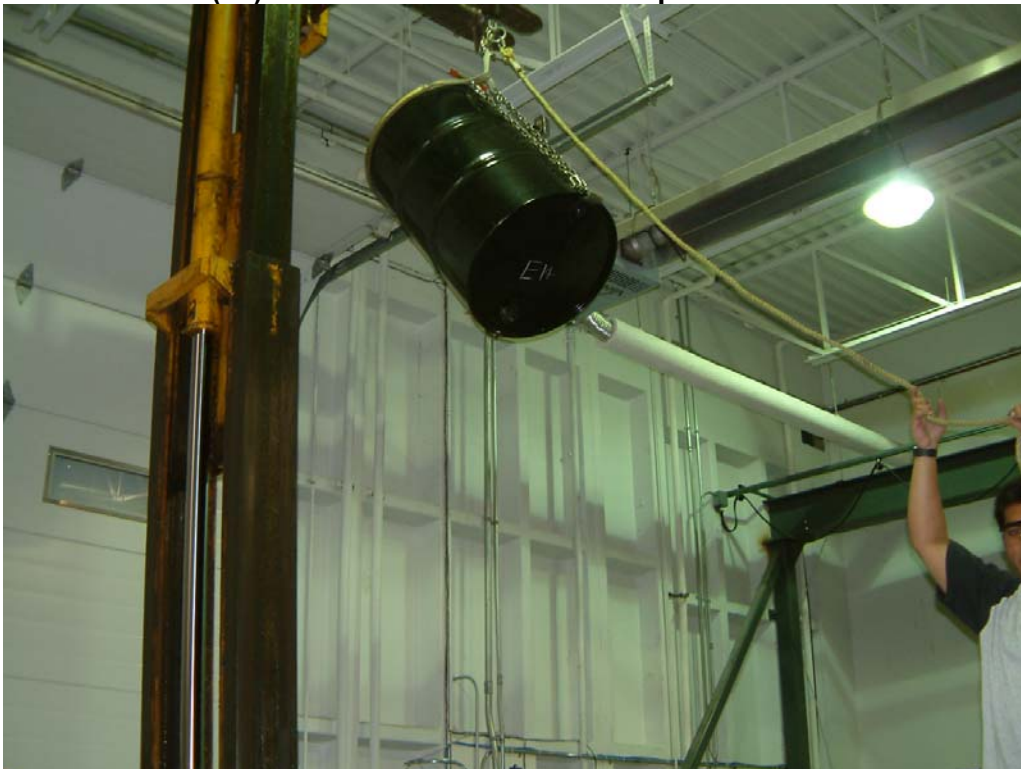
Photo 56 Lot E (14) Drum Prior to 6 O'clock Drop from 3.8 Metres
