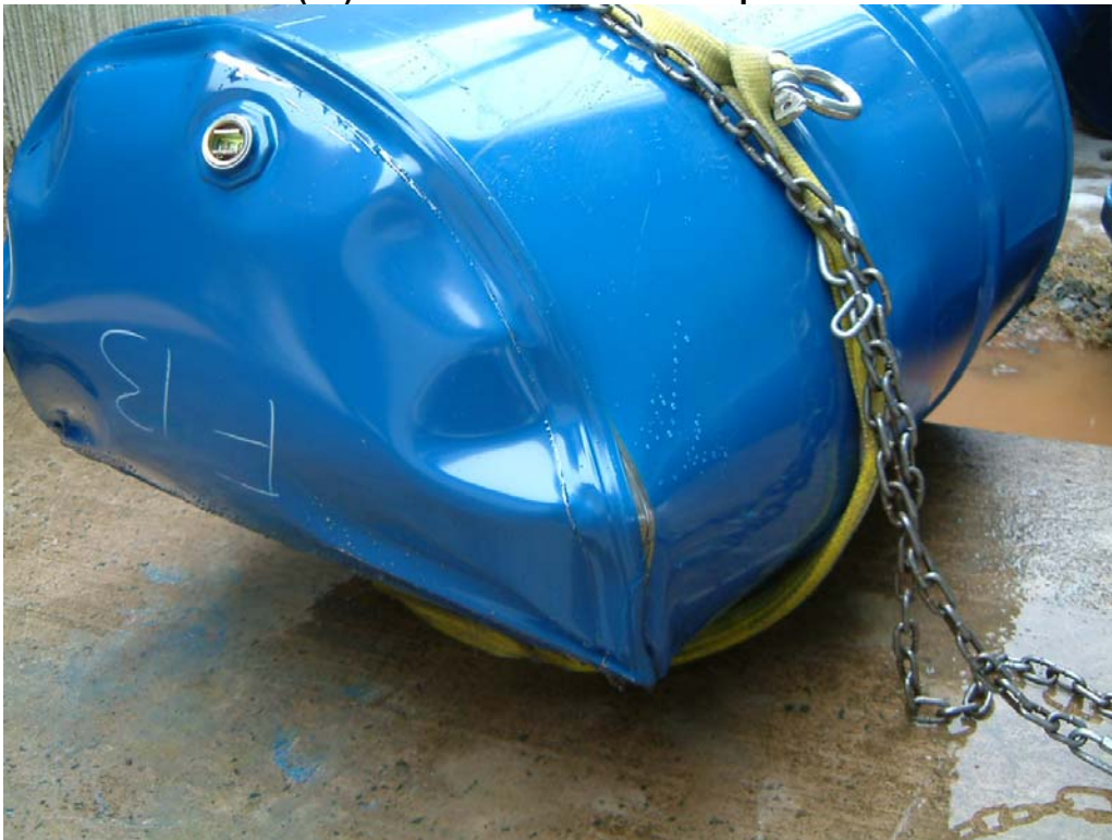
Photo 72 Failed Lot F(13) Drum after 6 O'clock Drop from 5.6 Metres
