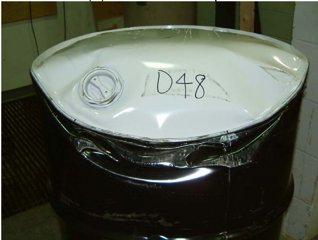
Photo 46 Lot E(1) Drum - Showing Preliminary Drop from 1.2 Metres
