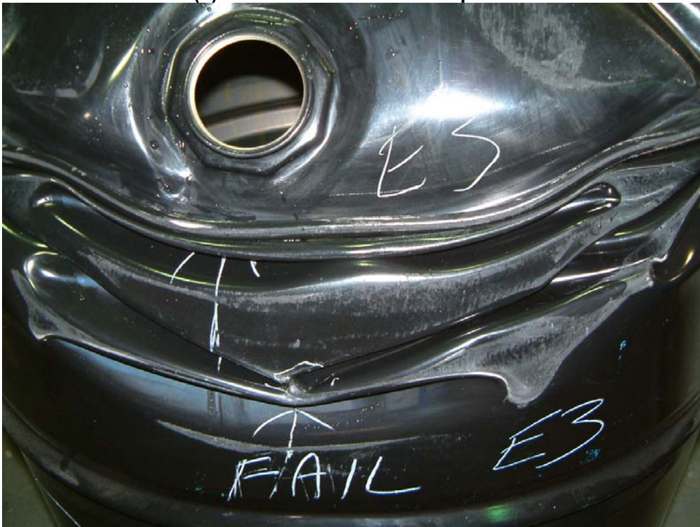
Photo 52 Failed Lot E(3) Drum after 6 O'clock Drop from 3.0 Metres
