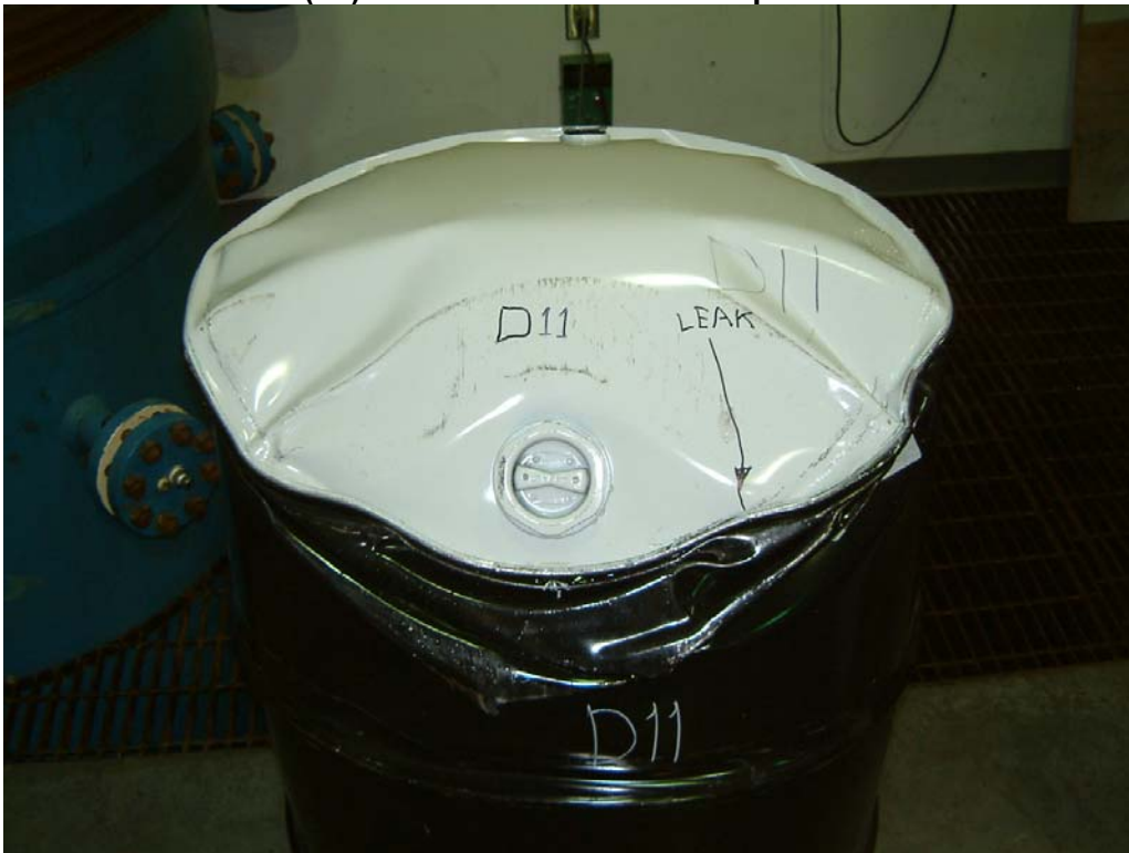
Photo 40 Failed Lot D(11) Drum after 6 O'clock Drop from 2.8 Metres
