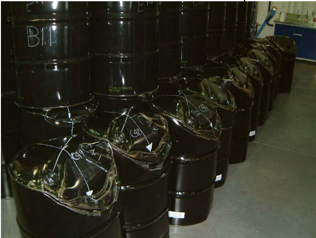
Photo 32 Lot C Drums after Series of 8 O'clock Drops
