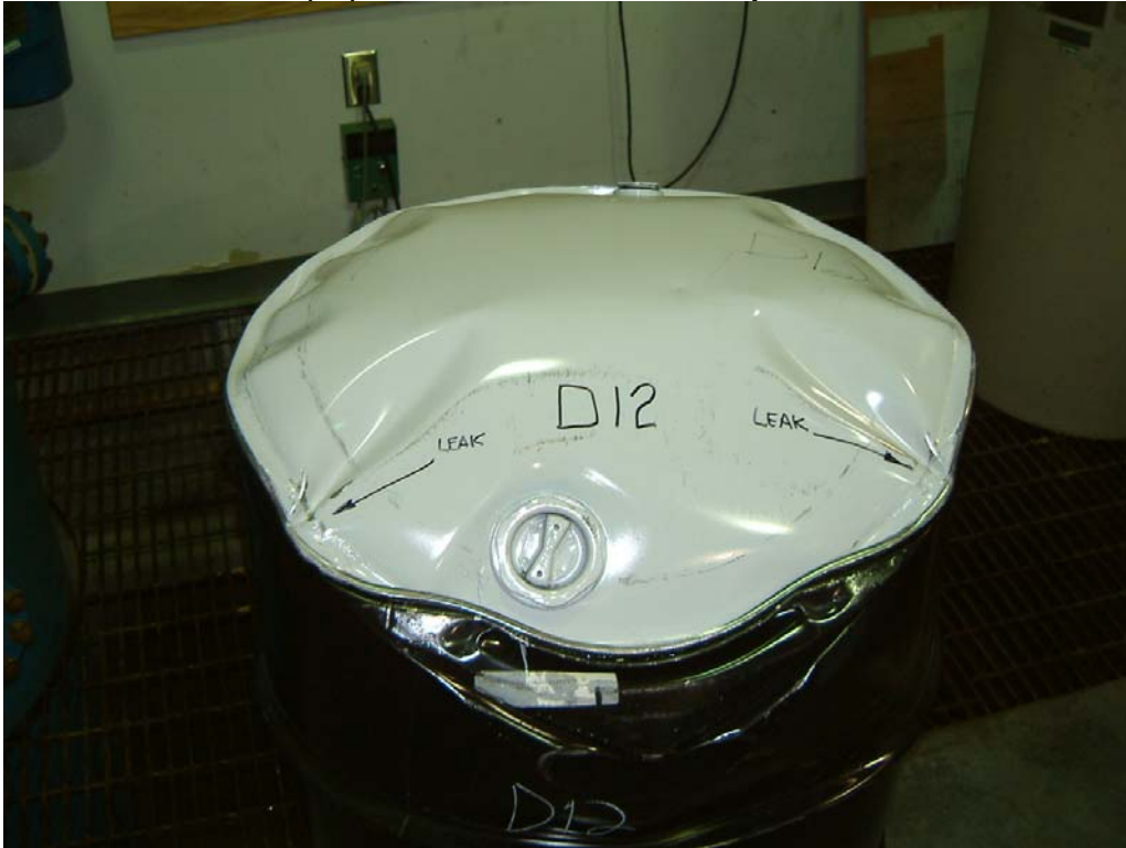
Photo 42 Failed Lot D(36) Drum after 8 O'clock Drop from 2.4 Metres
