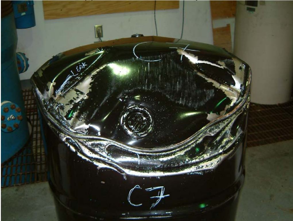
Photo 30 Failed Lot C(8) Drum after 6 O'clock Drop from 3.4 Metres
