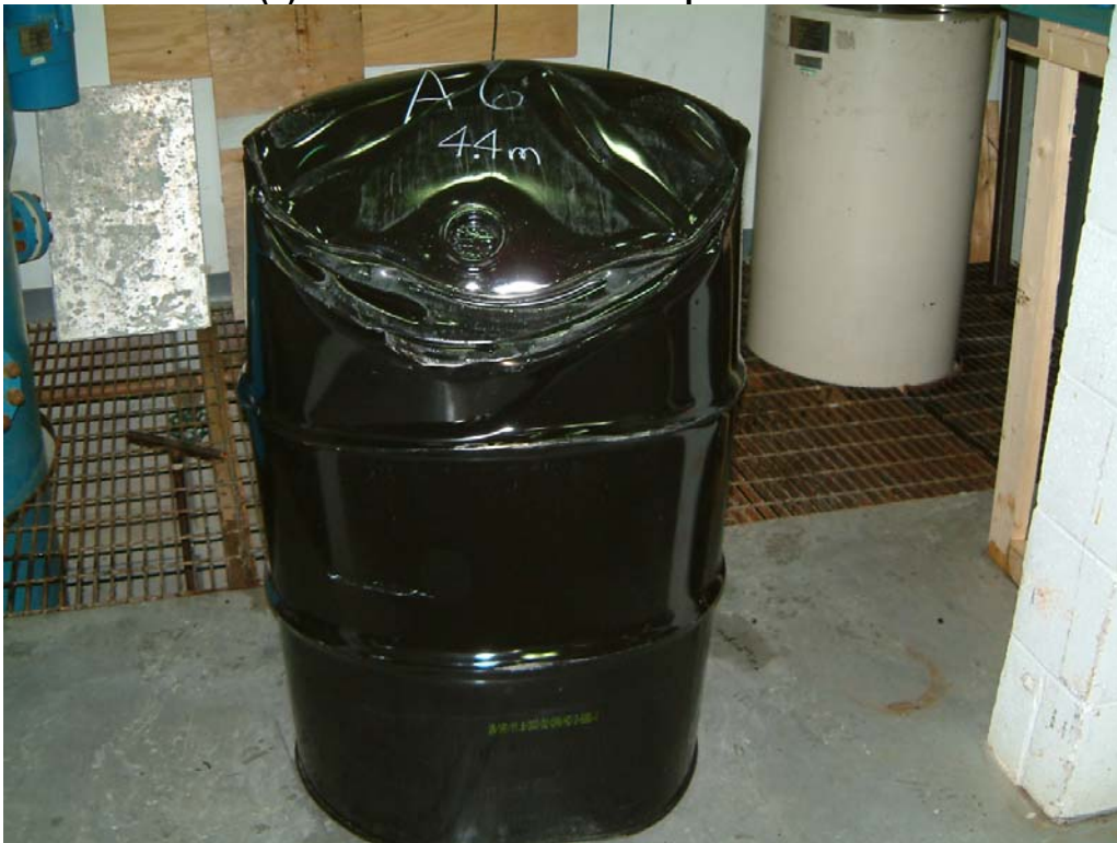
Photo 8 Lot A(6) Drum after 6 O'clock Drop from 4.4 Metres
