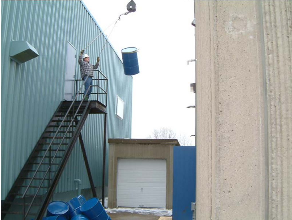
Photo 72 Failed Lot F(13) Drum after 6 O'clock Drop from 5.6 Metres
