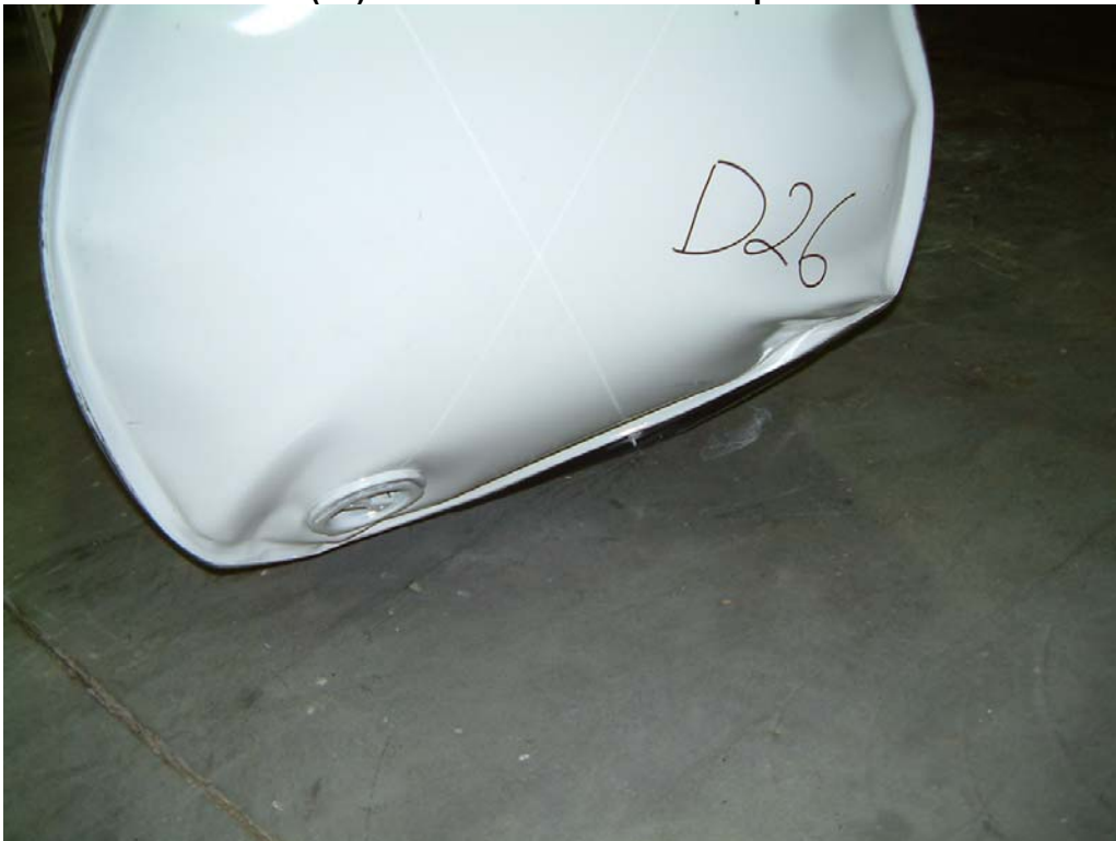
Photo 44 Passed Lot D(26) Drum after 8 O'clock Drop from 1.8 Metres
