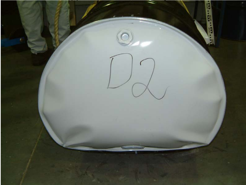
Photo 36 Lot D(3) Drum Release for 6 O'clock Drop from 3.0 Metres
