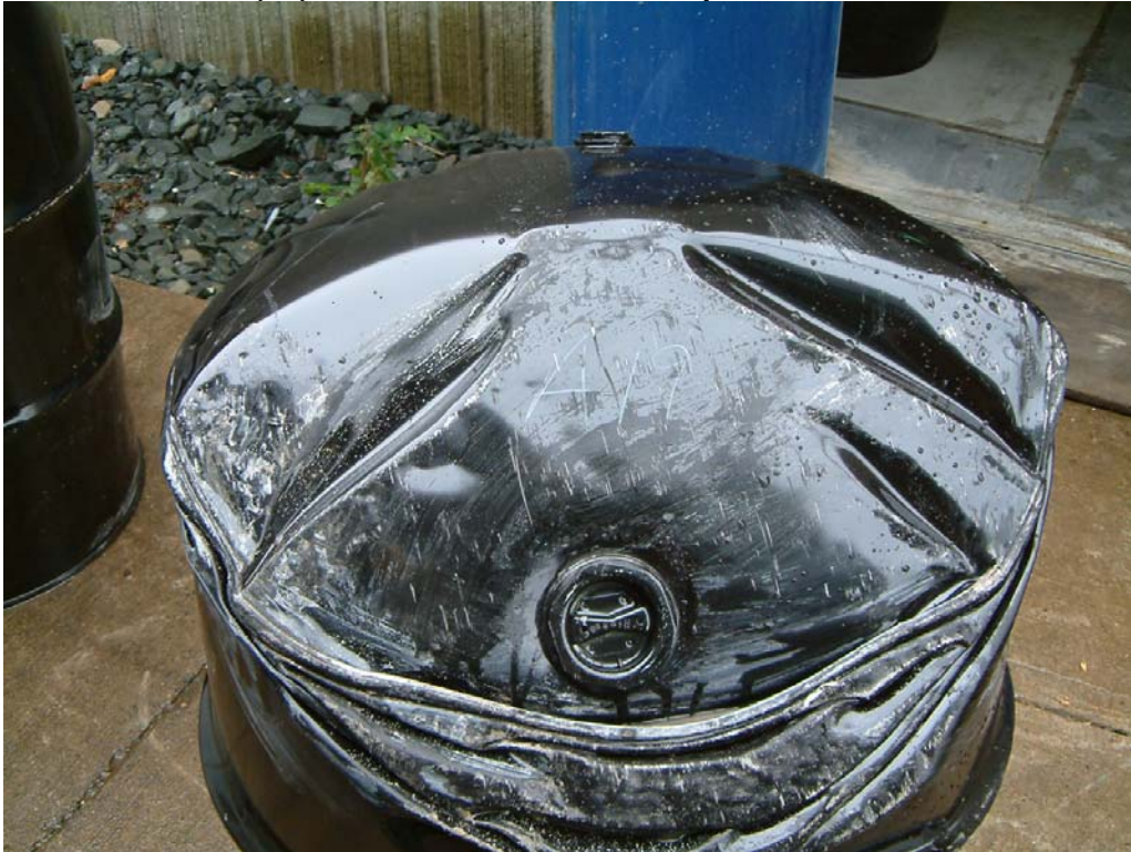
Photo 14 Lot A Drum after 6 O'clock Drop from 5.0 Metres
