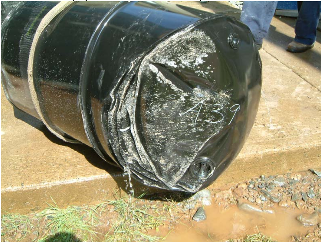
Photo 16 Lot A(39) Drum after 8 O'clock Drop from 4.8 Metres
