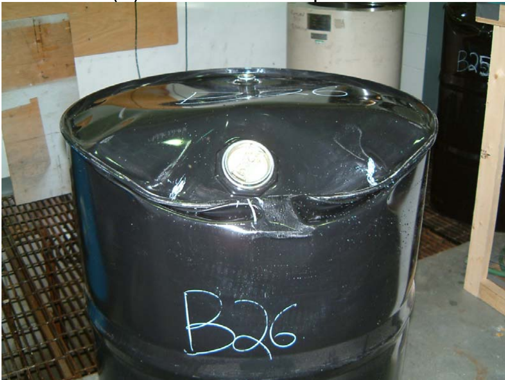
Photo 24 Lot B(26) Drum after 6 O'clock Drop from 1.0 Metres
