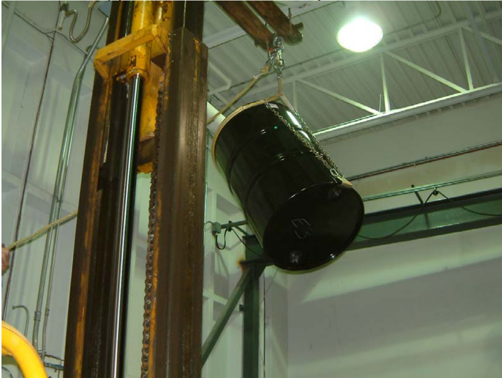
Photo 52 Failed Lot E(3) Drum after 6 O'clock Drop from 3.0 Metres
