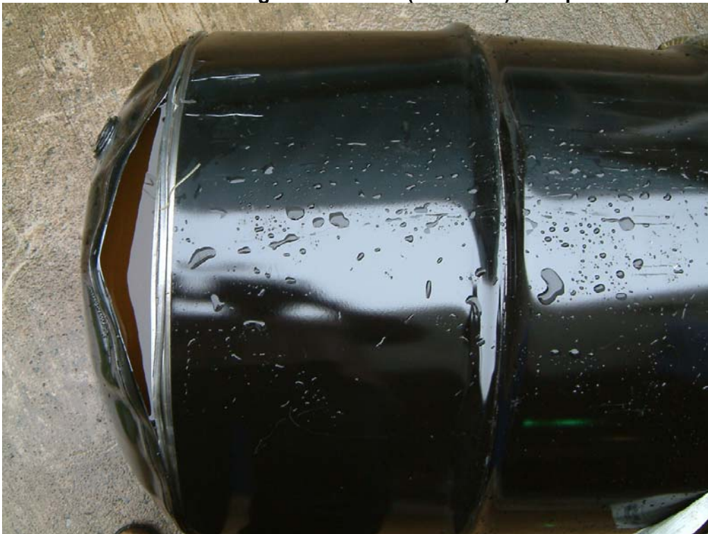
Photo 12 Lot A Drum Showing Failure Mode (6 O'clock) at Top Chime
