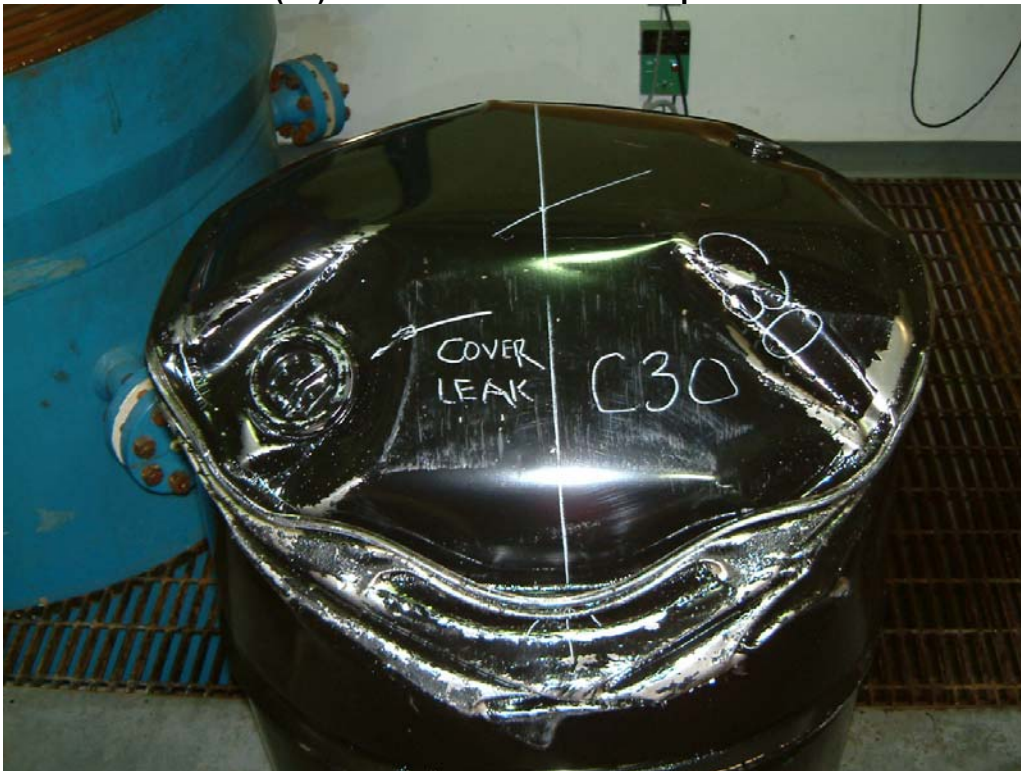
Photo 34 Failed Lot C(30) Drum after 8 O'clock Drop from 2.6 Metres
