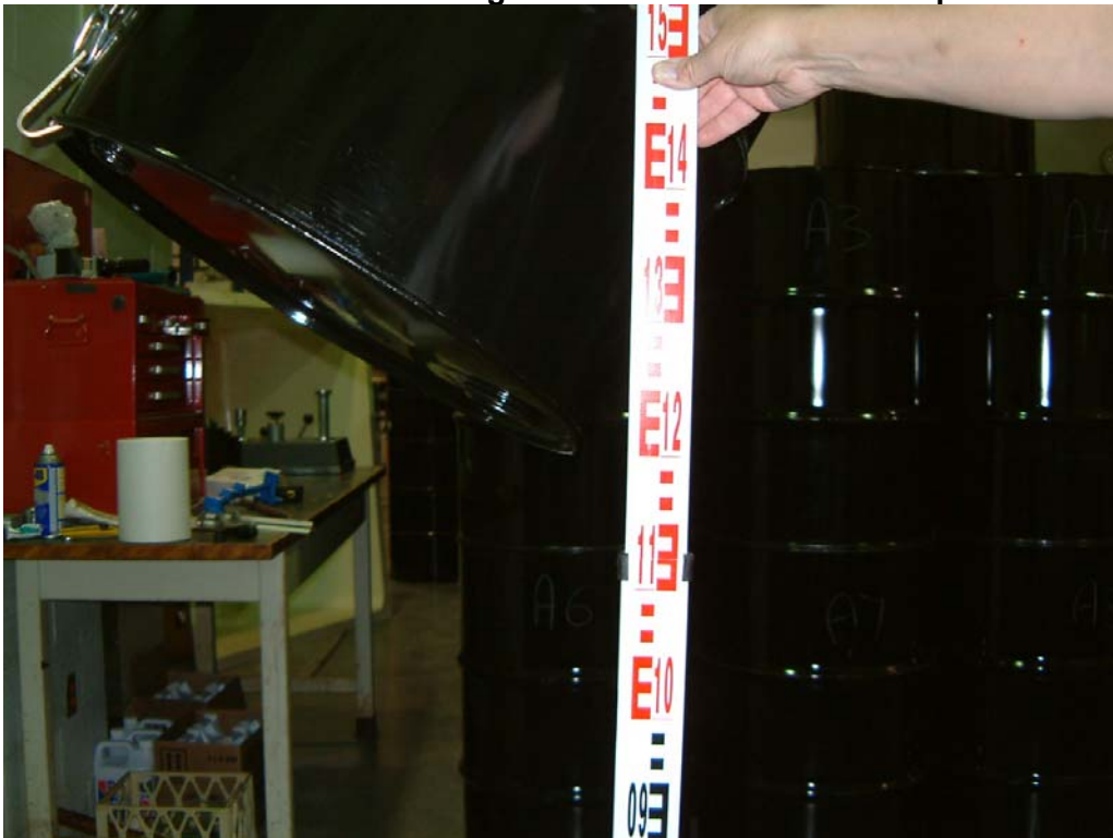
Photo 2 Metre Stick Measuring Procedure for 1.2 Metre Drop
