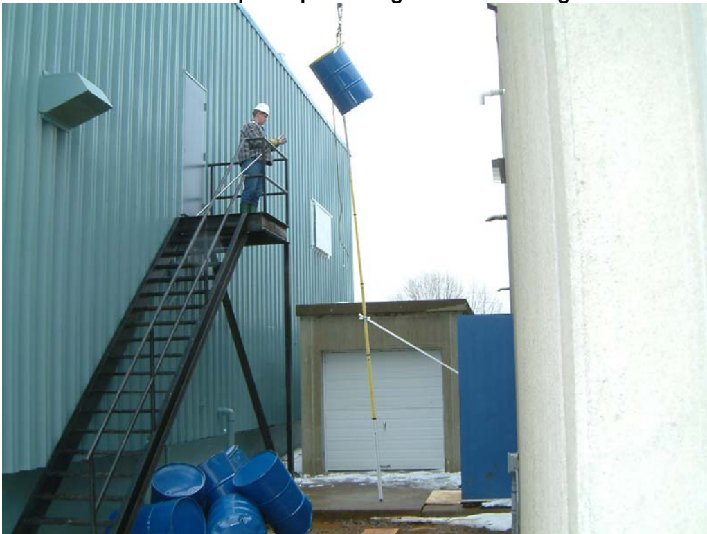
Photo 70 Lot F Drum Drop Setup Showing Metre Measuring Stick
