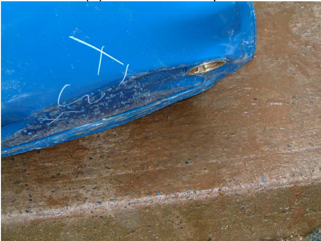
Photo 76 Failed Lot F(34) Drum after 8 O'clock Drop from 4.6 Metres
