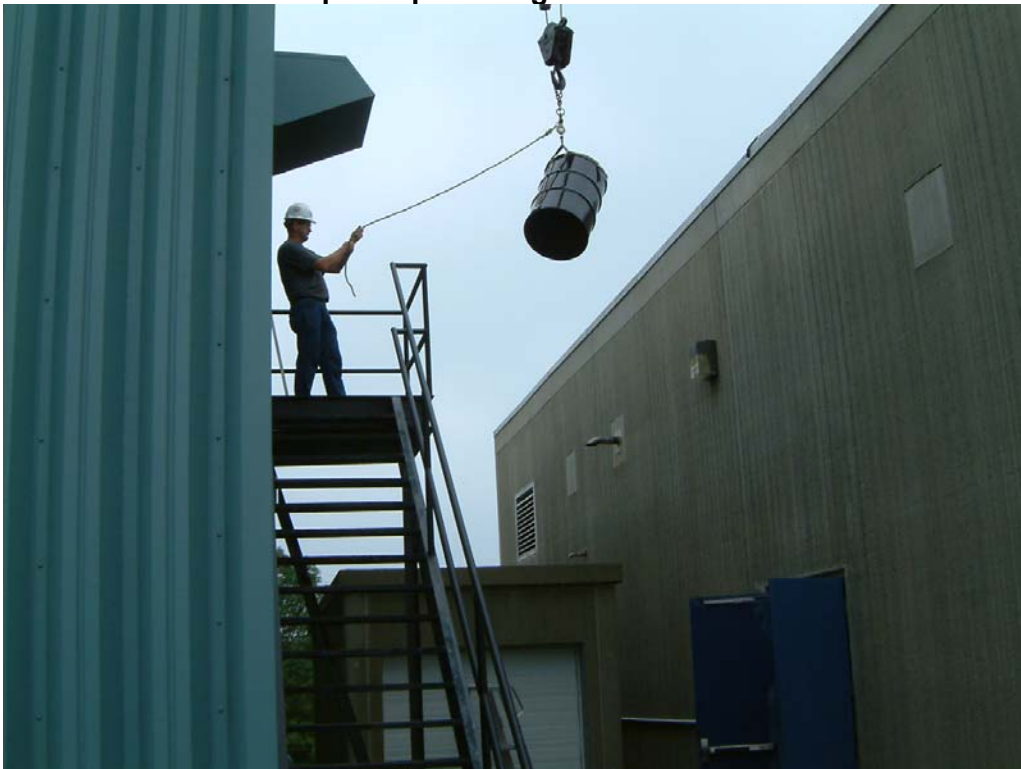
Photo 10 Lot A Drum Drop Setup for Heights Greater than 4.6 Metres
