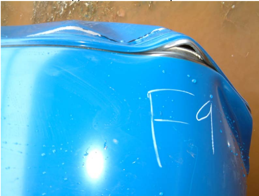
Photo 68 Failed Lot F(9) Drum after 6 O'clock Drop from 5.6 Metres
