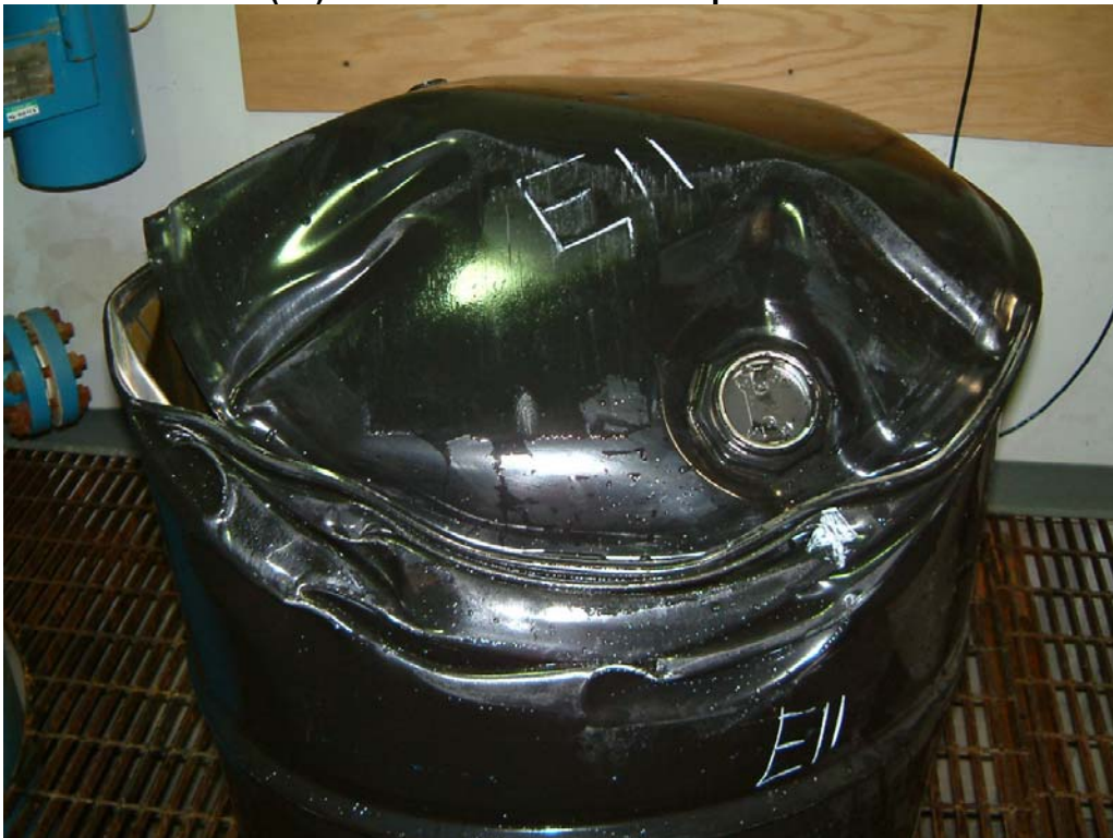
Photo 54 Failed E(11) Drum after 6 O'clock Drop from 3.6 Metres
