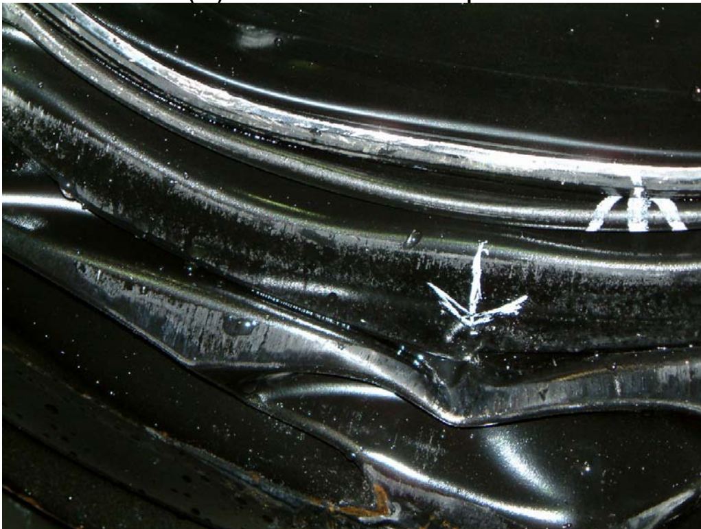
Photo 62 Failed Lot E(32) Drum after 8 O'clock Drop from 3.6 Metres
