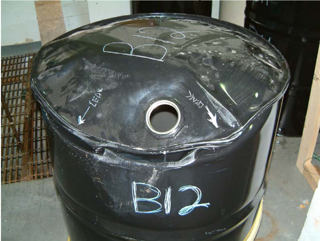
Photo 24 Lot B(26) Drum after 6 O'clock Drop from 1.0 Metres
