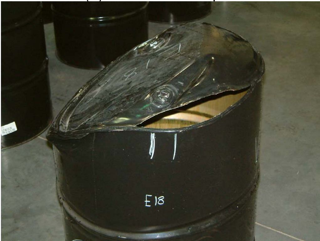
Photo 58 Failed Lot E(18) Drum after 6 O'clock Drop from 4.2 Metres
