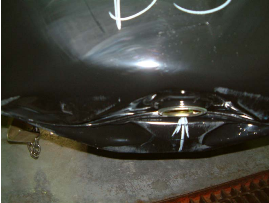
Photo 20 Lot B(38) Drum after 8 O'clock Drop from 0.6 Metres
