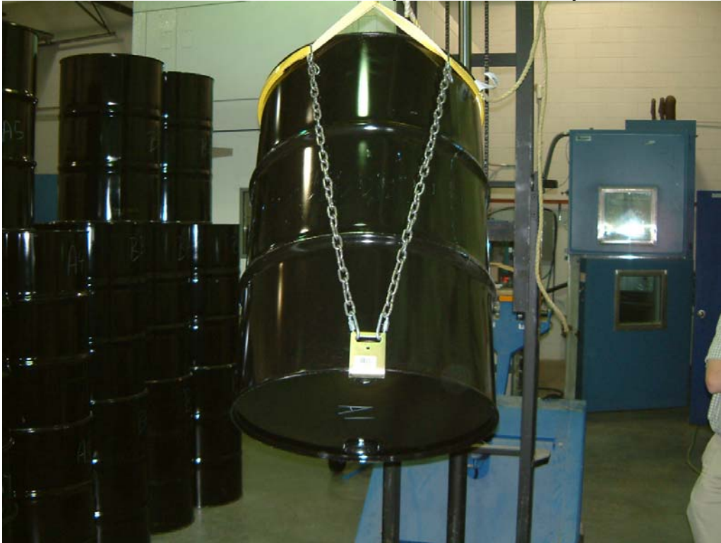
Photo 2 Metre Stick Measuring Procedure for 1.2 Metre Drop
