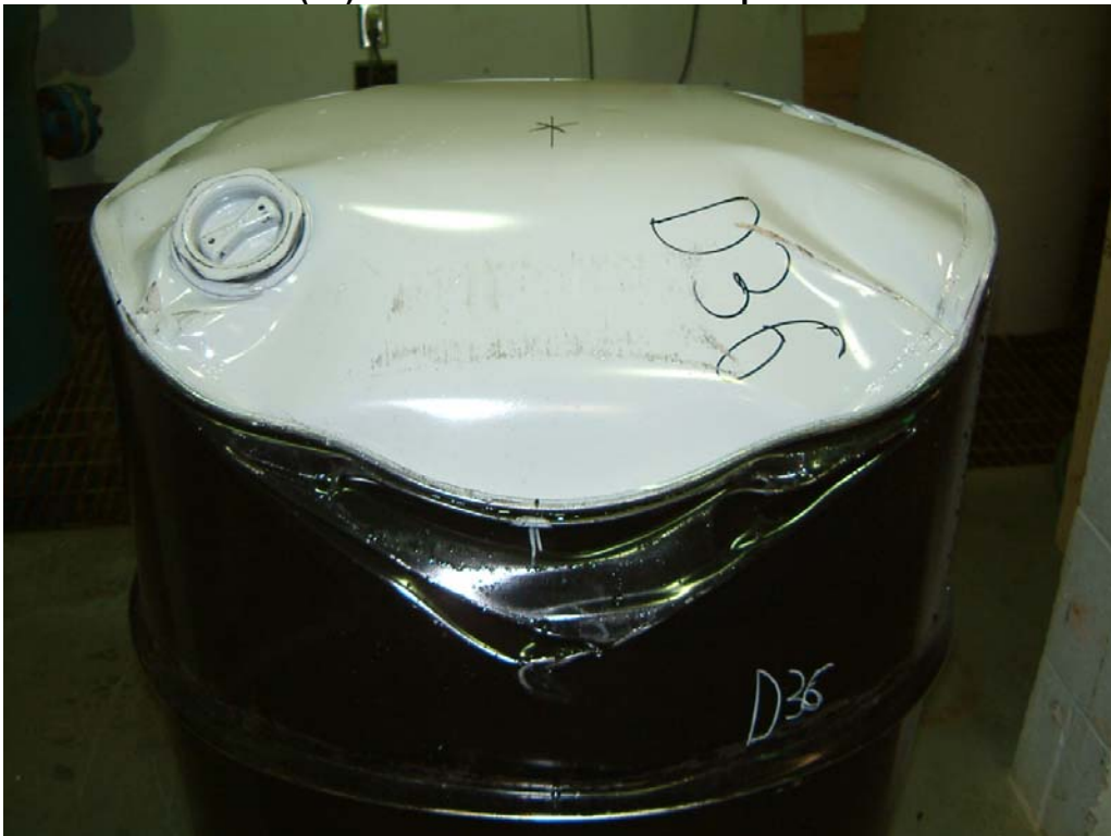
Photo 42 Failed Lot D(36) Drum after 8 O'clock Drop from 2.4 Metres
