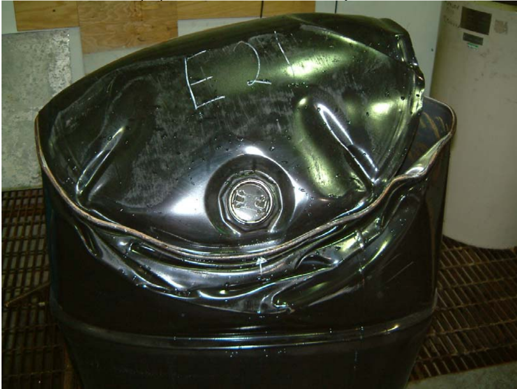
Photo 60 Bottom of Passed Lot E(25) Drum after Drop from 3.8 Metres
