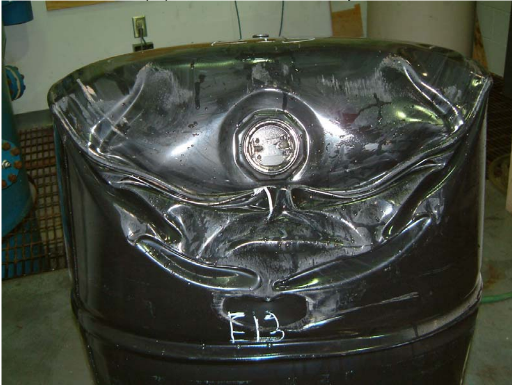
Photo 56 Lot E (14) Drum Prior to 6 O'clock Drop from 3.8 Metres
