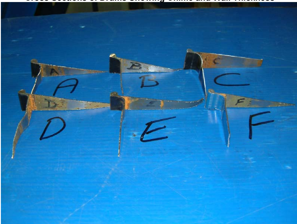
Photo 80 Cross Sections of Drums Showing Chime and Wall Thickness
