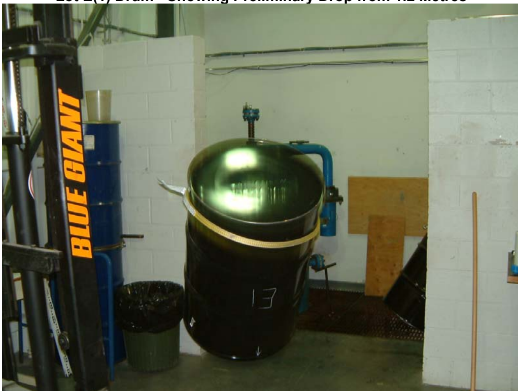
Photo 46 Lot E(1) Drum - Showing Preliminary Drop from 1.2 Metres
