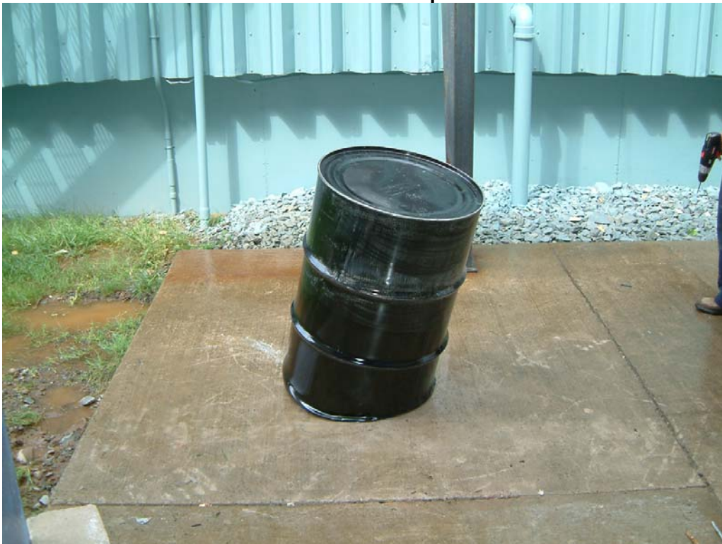
Photo 14 Lot A Drum after 6 O'clock Drop from 5.0 Metres
