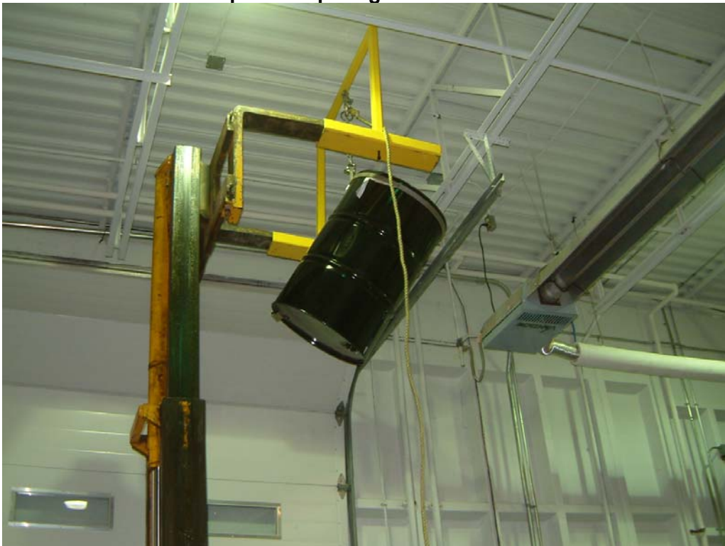
Photo 6 Forklift Setup for Drop Heights Less than 4.4 Metres
