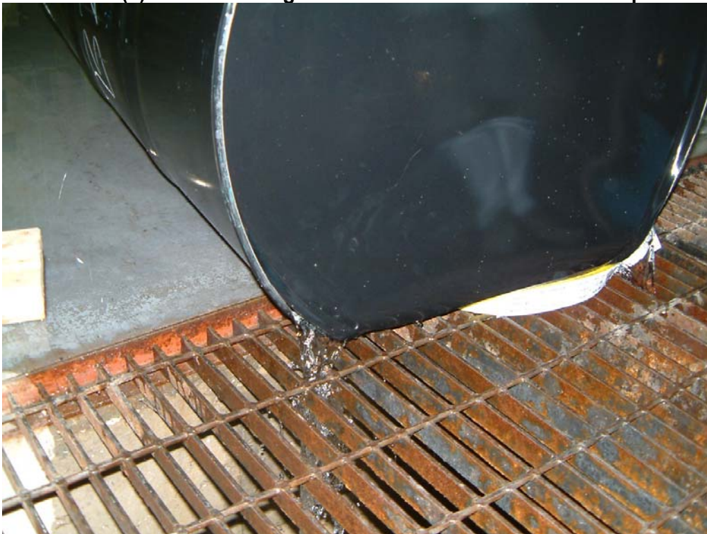
Photo 18 Lot B(2) Drum Showing Leak at Bottom after 2.0 Metre Drop
