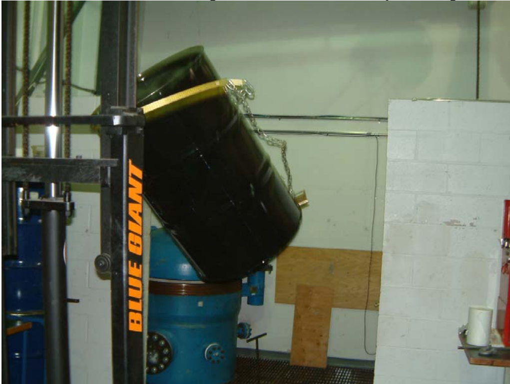
Photo 6 Forklift Setup for Drop Heights Less than 4.4 Metres
