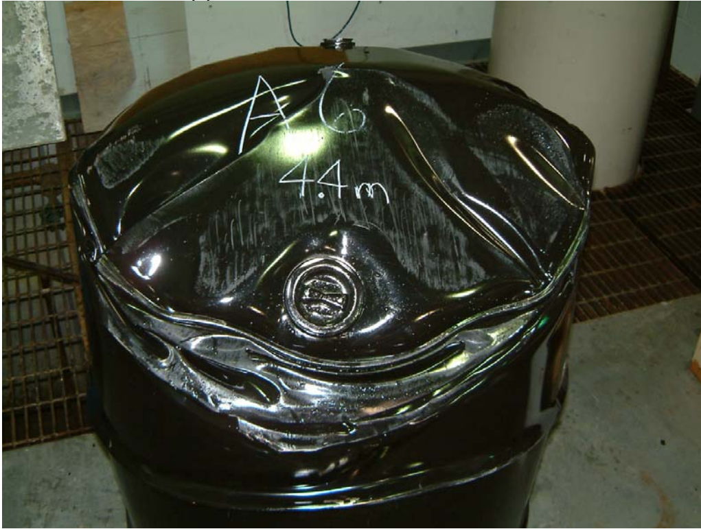
Photo 8 Lot A(6) Drum after 6 O'clock Drop from 4.4 Metres
