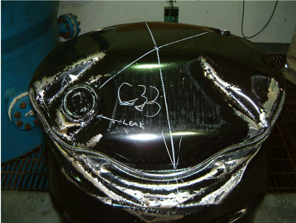
Photo 32 Lot C Drums after Series of 8 O'clock Drops
