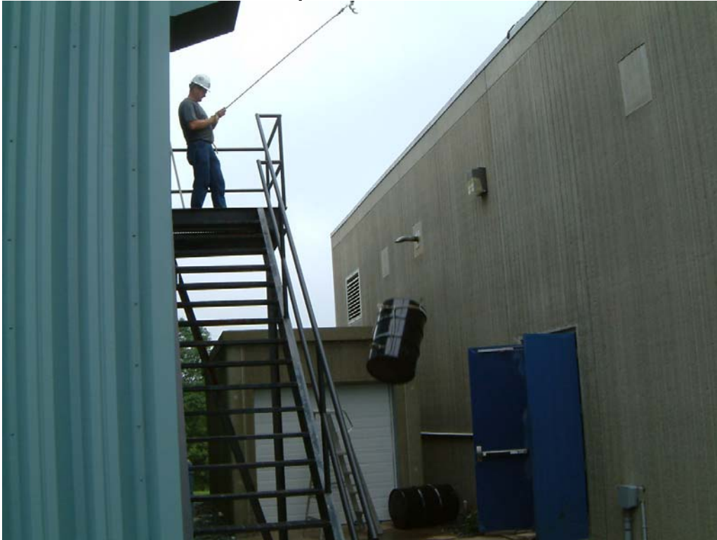
Photo 12 Lot A Drum Showing Failure Mode (6 O'clock) at Top Chime
