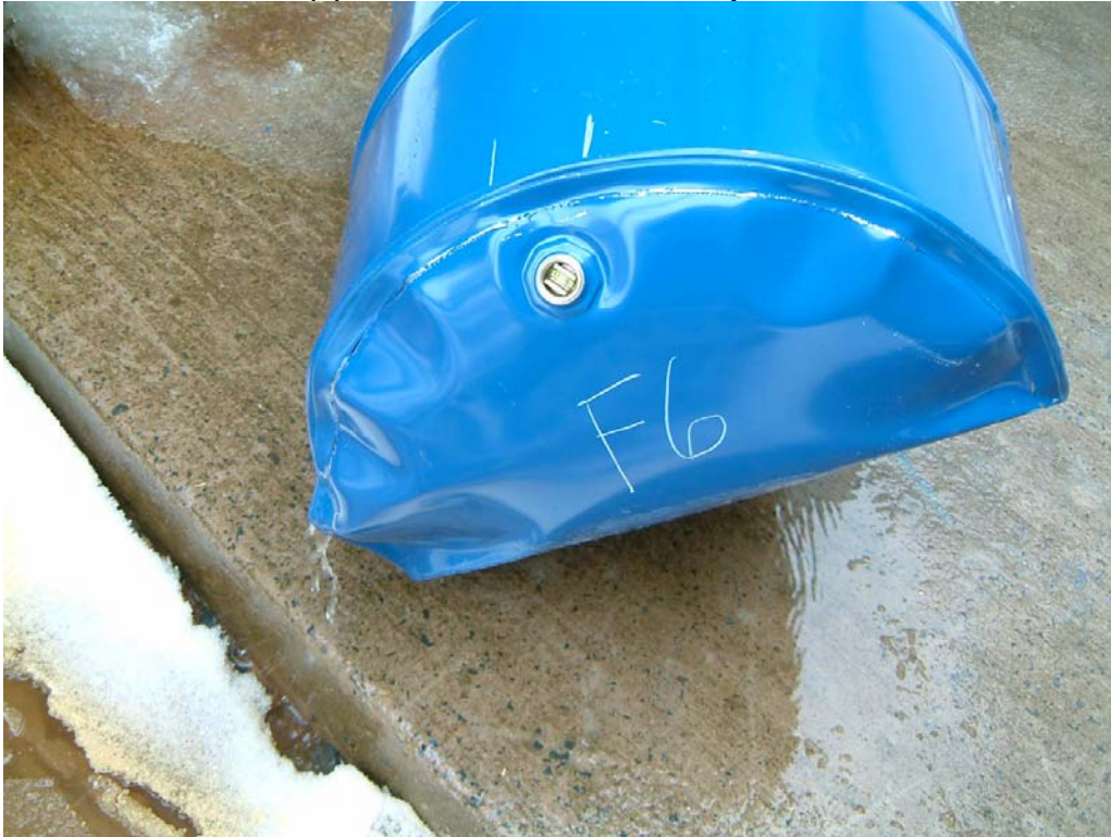
Photo 68 Failed Lot F(9) Drum after 6 O'clock Drop from 5.6 Metres
