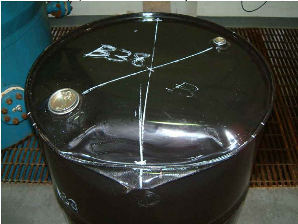
Photo 20 Lot B(38) Drum after 8 O'clock Drop from 0.6 Metres
