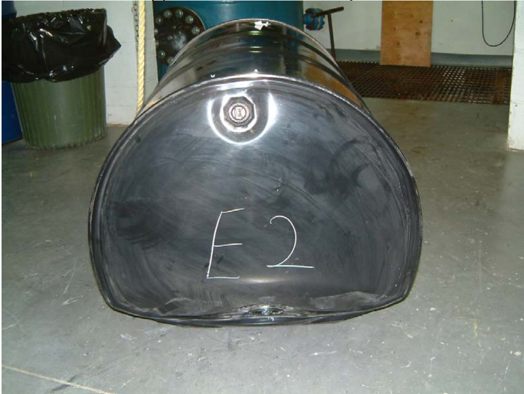
Photo 50 Lot E(2) Drum Bottom after 6 O'clock Drop from 2.0 Metres
