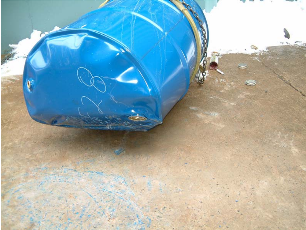
Photo 76 Failed Lot F(34) Drum after 8 O'clock Drop from 4.6 Metres
