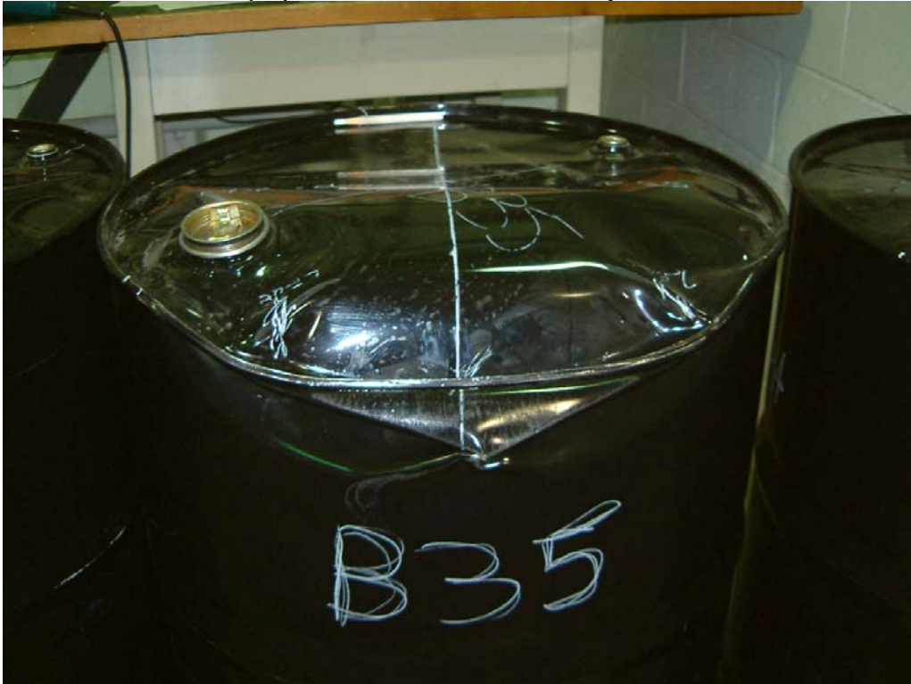
Photo 26 Passed Lot C(1) Drop after 6 O'clock Drop from 1.2 Metres
