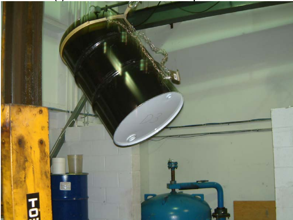
Photo 36 Lot D(3) Drum Release for 6 O'clock Drop from 3.0 Metres
