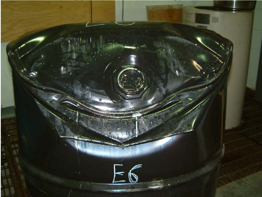
Photo 54 Failed E(11) Drum after 6 O'clock Drop from 3.6 Metres
