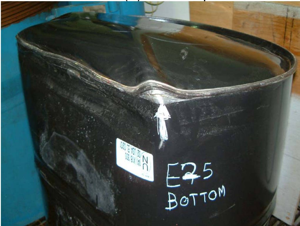
Photo 60 Bottom of Passed Lot E(25) Drum after Drop from 3.8 Metres
