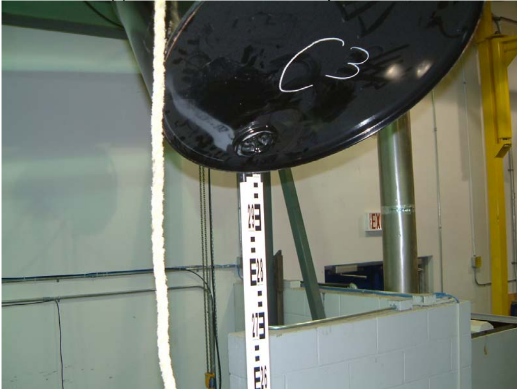
Photo 28 Failed Lot C(3) Drum - Showing Leak at Cover after 3.0 Metre Drop
