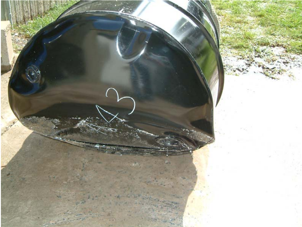
Photo 18 Lot B(2) Drum Showing Leak at Bottom after 2.0 Metre Drop
