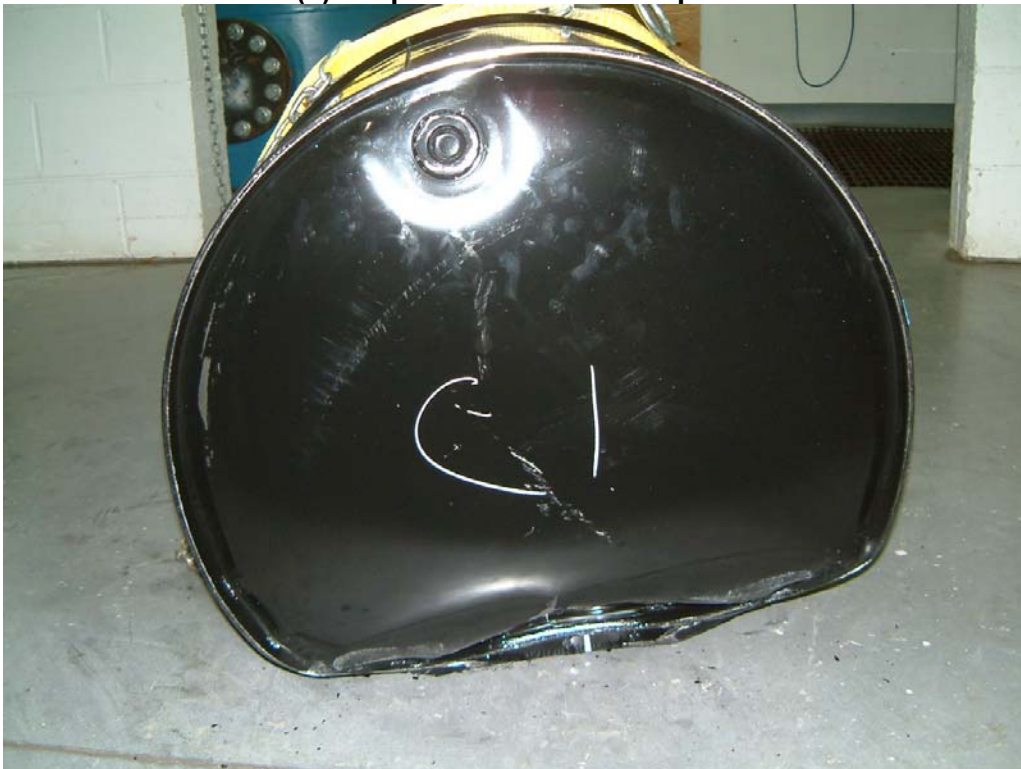
Photo 26 Passed Lot C(1) Drop after 6 O'clock Drop from 1.2 Metres
