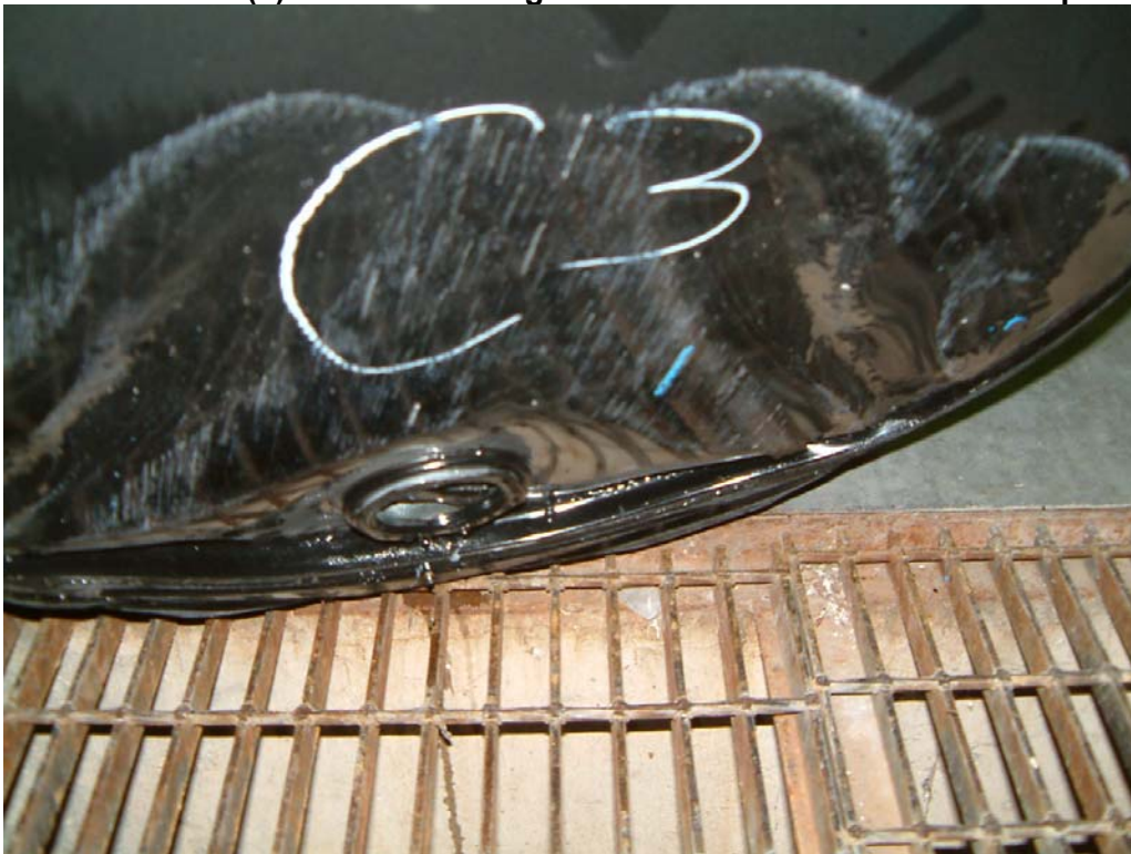
Photo 28 Failed Lot C(3) Drum - Showing Leak at Cover after 3.0 Metre Drop
