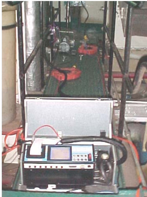
Figure 2.2 ECOM and Particulate Filter Holder Set-Up
