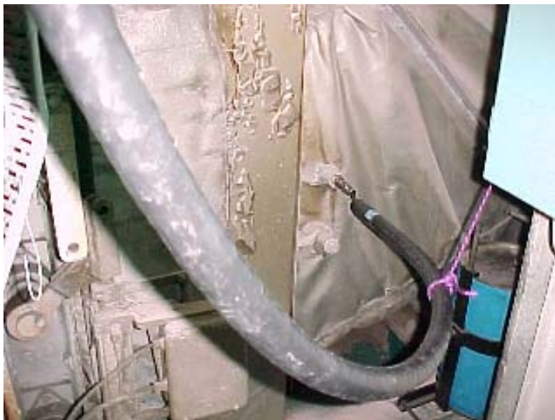
Figure 2.4 Sampling Probe Inserted into the Exhaust Port
