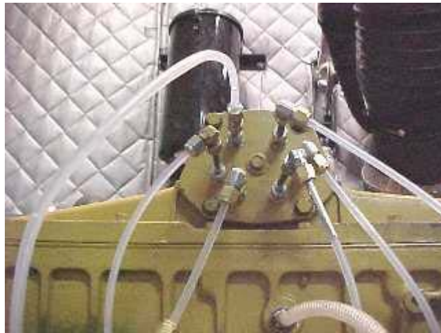
Figure 4.4 Single Point (SP) Injector
