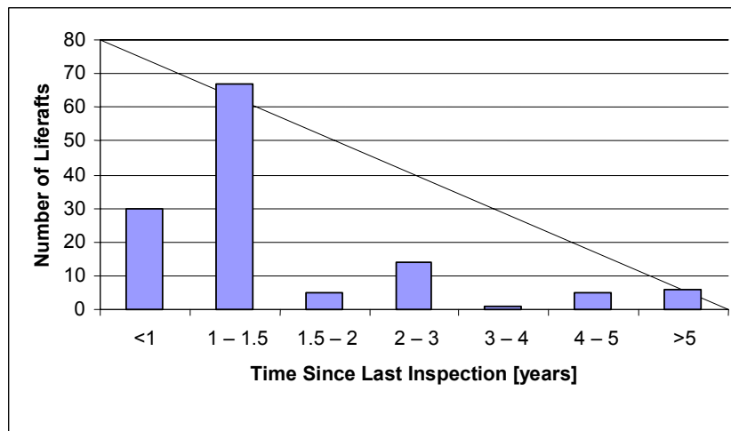
Figure 6.12 Inspection Interval – Critical Problem Serviceable Liferafts
