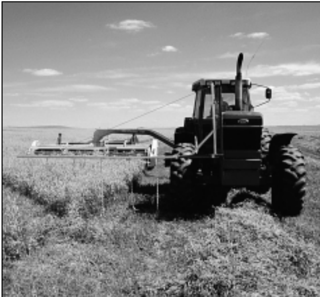
Attaching a flushing bar to the mower - conditioner will scare the hens off the nest and allow them to re-nest.
