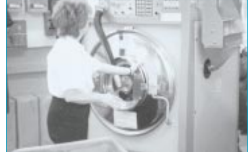
A wet clean facility in Hamilton, Ontario. Wet cleaning equipment eliminates the use of perchloroethylene, a hazardous solvent.
