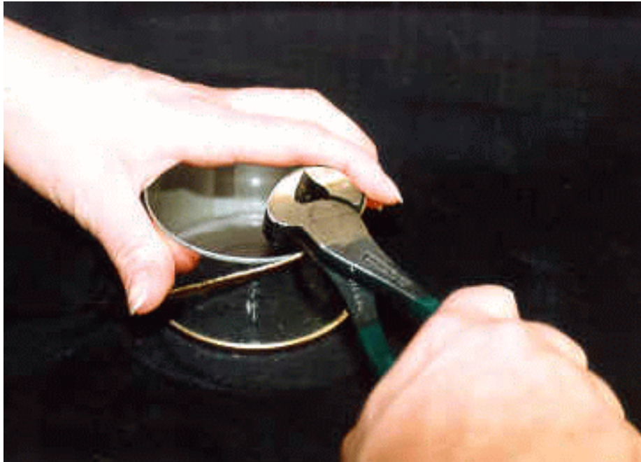
Figure 4.1.3.d - Removing Stripped Part of End
