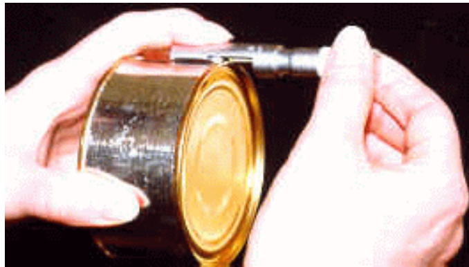
Figure 4.1.2.c - Seam Length Measurement
