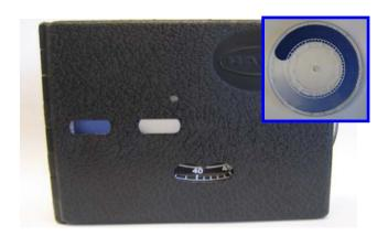
Photo 2: Example of a Colour Wheel Comparator manufactured by HACH (inset: close-up of colour wheel)
