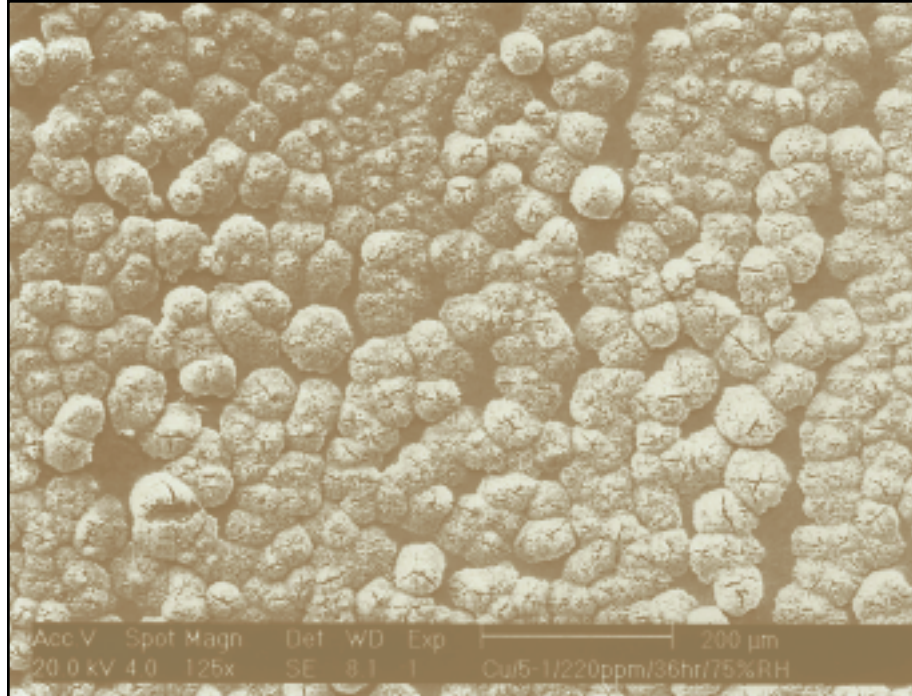
Figure 4. Scanning electron micrograph (SE mode) of surface deposits on copper after exposure to 220 ppm \text{PH}_3 for 36 hours at 30°C and 75% RH
