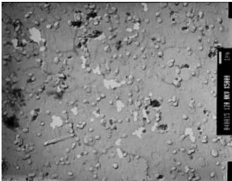
Figure B17 - Typical image from TEM of PM 10 for LD-6000 fuel at 5000 magnification
