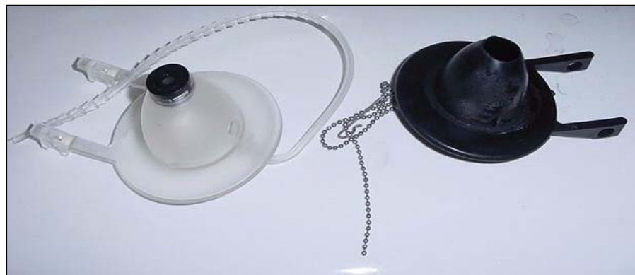
Figure 1 - Rubber Flapper Chain & Metallic Bead Flapper Chain
