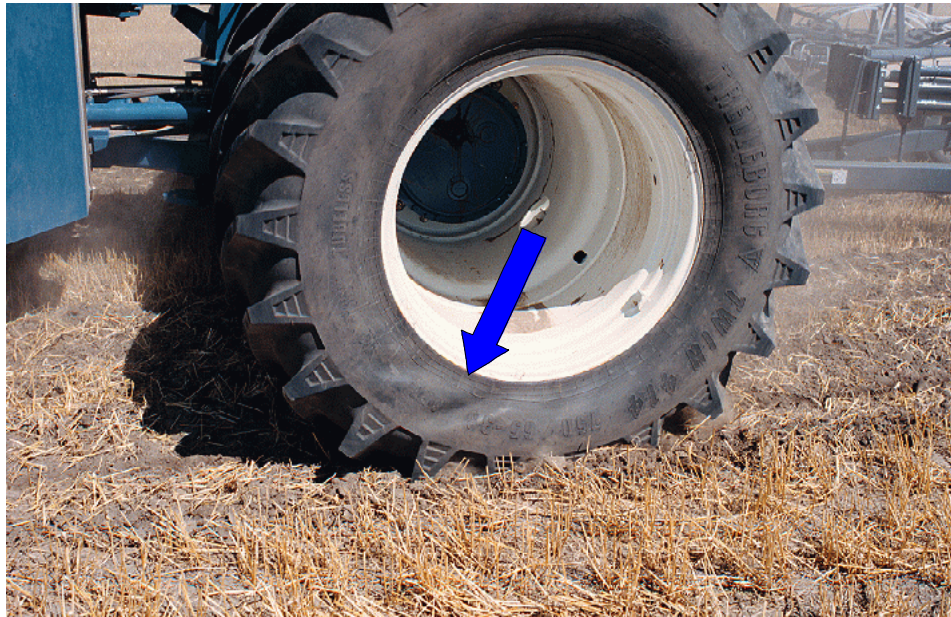
Figure 9. Trelleborg Sidewall Wrinkling under Load
