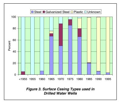
Steel and galvanized steel were the main casing types until the start of the 1980s, at which time plastic casing started to replace the use of steel and galvanized steel casings.
